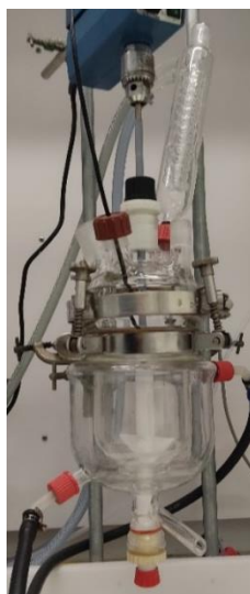
Figure 2-5 - Batch reactor used for transesterification reactions.
