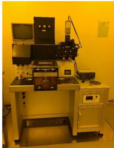
**Figure A-7** Manual alignment equipment in ESIEE Paris CLEANROOM
