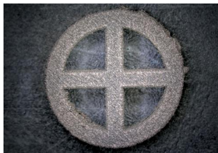
Figure 2-19 A microscopic view of 3-D printed titanium covered with the Diamond coating developed by RMIT researchers [161]
