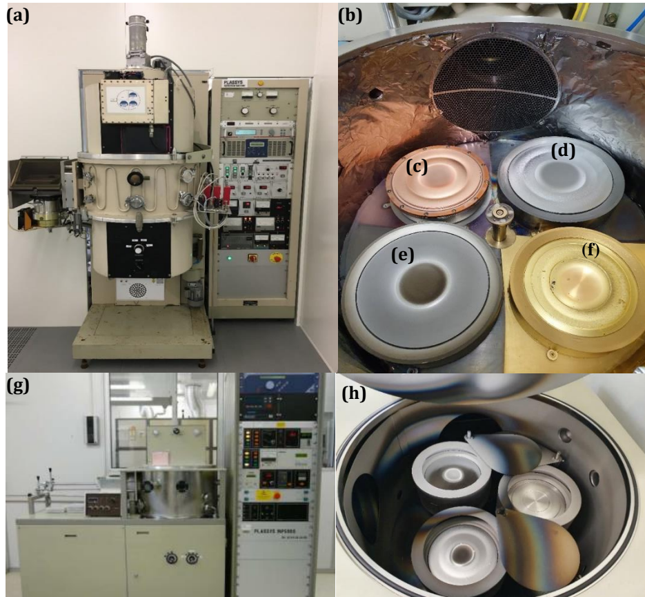
Figure A-3 (a) Cathodic RF magnetron sputtering- ALCATEL - SCM 600 in ESIEE Paris CLEANROOM with Copper (Cu), Chromium (Cr), Titanium Tungsten (TiW), and Gould (Au) target, (b) inside of the sputtering chamber of SCM 600, the (c) Cu, (d) Cr, (e) TiW, (f) Au in the sputtering machine, (g) Magnetron sputtering equipment PLASSYS MP500S, (h) inside the sputtering chamber of MP500S
