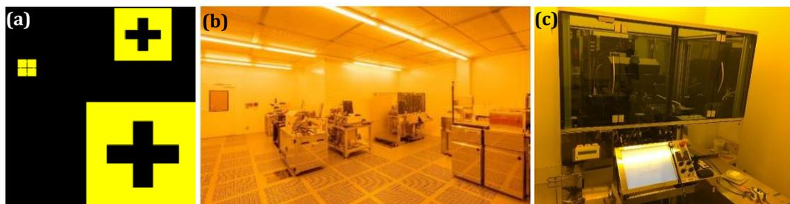
**Figure A-8** (a) Image of Alignment cross on the side of the mask in 2-D design file, (b) 58 m<sup>2</sup> area in class 100 dedicated to photolithography and substrate sealing, (c) Automatic alignment equipment in ESIEE Paris CLEANROOM [283]
