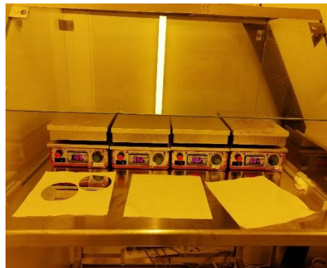
Figure A-6 Hot plate in the ESIEE Paris CLEANROOM heated at 109° C, 65.2° C, 90.2° C, and 50.4° C. The wafers are put on rest period before putting on the hotplate
