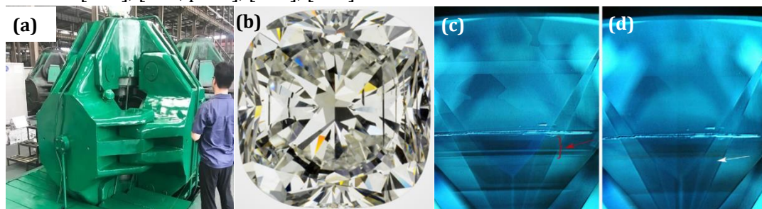
Figure 2- 18 (a)A reactor for fabricating HPHT Diamond, (b) the biggest HPHT Diamond reported by Gemological Institute of America (GIA) [146], (c) Fluorescence image of the HPHT-grown Diamond's pavilion (Taken with DiamondView), (d) The patterning in the corresponding phosphorescence image closely resembles the fluorescence image [113],[158],[159]
