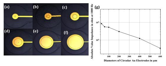
**Figure 3- 40** The samples before used in characterization (a)30  $\mu$ m, (b) 60  $\mu$ m, (c) 100  $\mu$ m (d) 200  $\mu$ m (e) 100  $\mu$ m, (f) 600  $\mu$ m, (g) relation between the size and impedances at a single frequency
