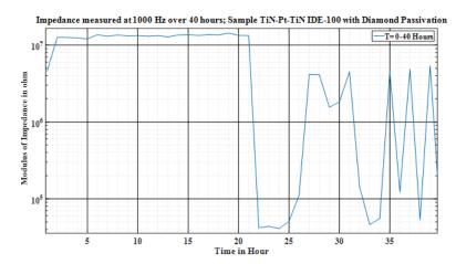
Figure 4-14 Drift in the result due to water leakage
