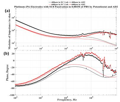
Figure 3-51 (a) mpedance, and (b) phase of 400  $\mu$ m and 600  $\mu$ m Pt samples done in potentiostat and AD2
