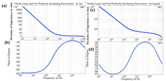
**Figure 3-23** EIS for simulation performed in Figure 3-21 considering imperfect passivation layer, (a) Impedance, (b) phase in air, (c) impedance, (b) phase in liquid
