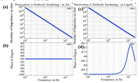
**Figure 3-21** EIS for simulation performed in Figure 3-21 considering perfect passivation layer, (a) Impedance, (b) phase in air, (c) impedance, (b) phase in liquid
