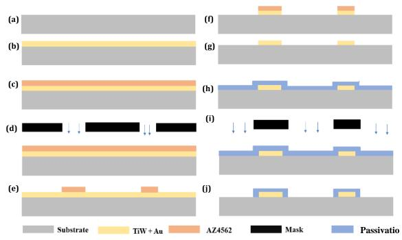
**Figure 2-11** Flow diagram of different steps of microfabrication in cleanroom (a) Substarte, (b) metal layer, (c) photoresist laer, (d) UV exposure, (e) development of resist, (f) etching, (g) removal of resin, (h) spin-coating of passivation layer, (i) UV exposure, (j) after PEB and then development
