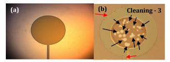
Figure 2-31 The same 600  $\mu$ m circular TiN-Pt-TiN electrode before and after cleaned with cleaning method -3
