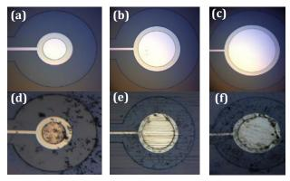
**Figure 3-44** The samples before used in characterization (a) 200  $\mu$ m (b) 400  $\mu$ m (c) 600  $\mu$ m, and after used in characterization (d) 200  $\mu$ m (e) 400  $\mu$ m (f) 600  $\mu$ m
