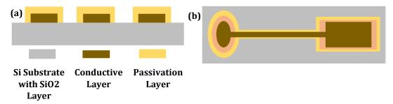
Figure 3-37 (a) 2-D cross section of the electrodes, (b) top view of a single electrode
