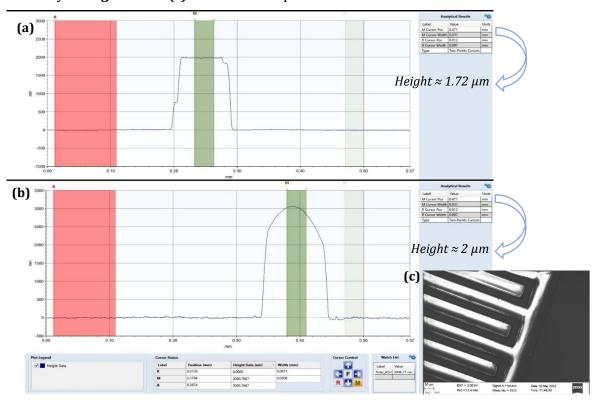
**Figure 4- 10** samples with (a) intrinsic Diamond, (b) SU8 passivation, (c) samples with Diamond passivation seen in SEM
