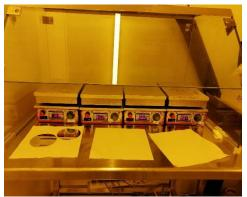
**Figure A- 6** Hot plate in the ESIEE Paris CLEANROOM heated at 109° C, 65.2° C, 90.2° C, and 50.4° C. The wafers are put on rest period before putting on the hotplate
