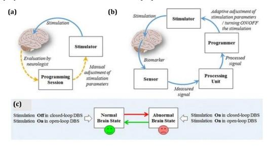
**Figure 1-9** (a) Open-loop DBS, (b) Closed-loop DBS, (c) Simple schematic of the 2 types of DBS [108]
