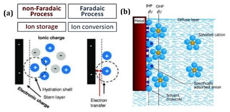
Figure 3-3 (a) Ion storage vs. ion conversion as the key difference between Faradaic and non-Faradaic (capacitive) electrode processes, using different examples, (b) the presence of a double layer when the sample is submerged in the liquid solution, IHP means Inner Helmholtz Plane, and OHP means Outer Helmholtz Plane [205], [210]
