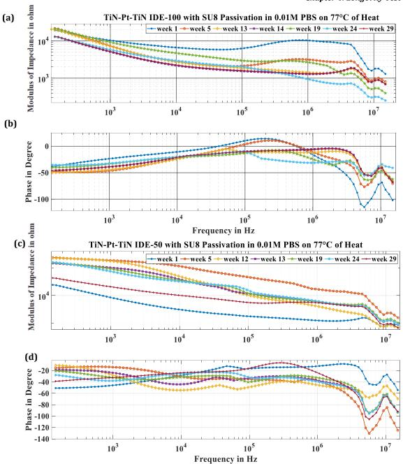
**Figure 4- 19** Data acquisition with AD2 from the samples with SU8 Passivation on heat (a) impedance, (b) phase of IDE with 25 pairs of fingers; (c) impedance, (d) phase of IDE with 50 pairs of fingers. Week 1 to 29 represent the time that the IDE is placed in PBS with temperature and week 29 is equivalent to around 9 years
