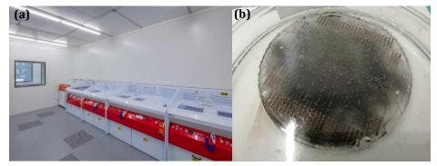
**Figure A-10** (a) Chemistry-2 room in ESIEE Paris Cleanroom for Wet Etching [283], (b) Wet etching of a Glass wafer covered in TiN
