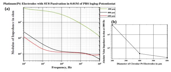
**Figure 3-45** (a) Impedance Spectroscopy data at 1000 Hz for different diameters, (b) the relation between the size and the impedance is inverse
