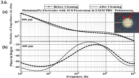
**Figure 3- 47** (a) Impedance of a 400μm in diameter circular Pt electrode in PBS, (b) phase of a 400μm in diameter circular Pt electrode in PBS
