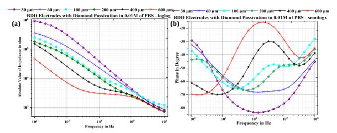
**Figure 3-69** (a) Absolute value of impedance, (b) phase of Diamond electrodes with intrinsic Diamond passivation
