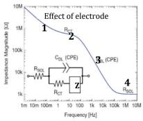
**Figure 3- 2** Bode plot of the impedance magnitude of the Randles equivalent model of an electrochemical interface comprising both non-Faradaic and Faradic phenomena [196]
