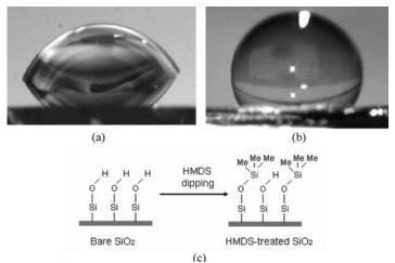
**Figure A- 1** Shapes of a water droplet on an untreated (a) and a HMDS-treated (b) silicon oxide (SiO<sub>2</sub> = Si) substrate. (c) Schematic representation of the chemical reaction occurring on the surface of SiO<sub>2</sub> substrates by dipping in HMDS solution [281]
