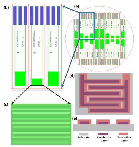
Figure 2-4 (a) The new mask designed for fabrication of IDE with different pairs of fingers in CoventorWare10.4, (b) Zoomed-in vision of 3 single strip with 25 and 50pairs of fingers, (c) zoomed-in view of the finger-like structures, (d) 2-D representation of the top view of an IDE, (e) top view of the IDE structure, (f) 2-d cross-sectional view of an IDE
