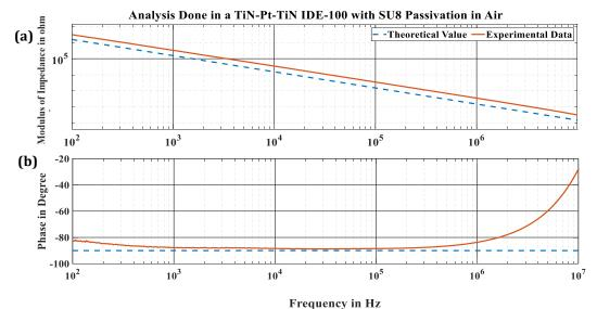
Figure 3-31 (a) Absolute value of Impedance, (b) phase
