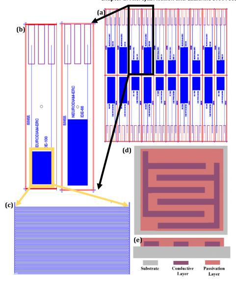
Figure 2-3 (a) The mask designed for fabrication of IDE with different pairs of fingers in CoventorWare10.4, (b) Zoomed-in vision of 2 single strip with 66 and 100 pairs of fingers, (c) zoomed-in view of the finger-like structures, (d) 2-D representation of the top view of an IDE, (e) top view of the IDE structure, (f) 2-d cross-sectional view of an IDE
