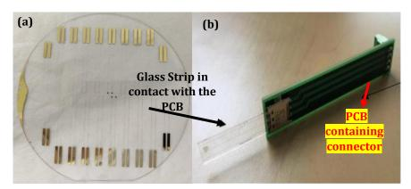
Figure 2-13 (a) Gold electrodes on a glass wafer, (b) Electrode strip connected to the interface PCB
