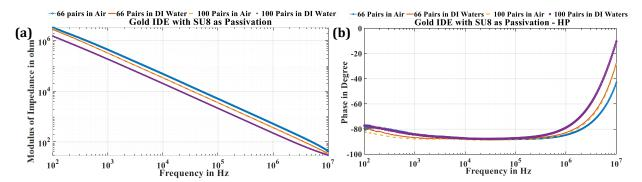
**Figure 3- 16** (a) Absolute value of impedance of IDE in different environment, (b) phase of IDE in different environment
