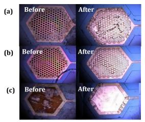
Figure 2-33 Three different 400  $\mu m$  hexagonal TiN electrodes before and after cleaning Figure 2-33 shows 3 different samples (400  $\mu m$  hexagonal TiN electrodes), where the before images show some samples after they were characterized and cleaned with cleaning method - 1 and 2, and the after images show after the same samples were cleaned with cleaning method - 4.
