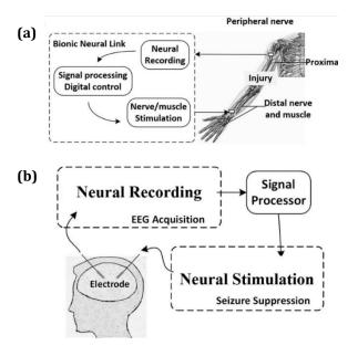
**Figure 1-8** Concept of (a) the Bionic Neural Link and (b) the epileptic seizure detection and suppression using neural recording and stimulation circuits [70]
