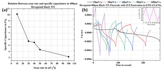
**Figure 3- 62** For 400  $\mu$ m hexagonal black Tin electrode (a) The decrease in specific capacitance with the increase in scan rate, (b) redox reaction rate decreases with the increase in scan rate
