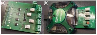
Figure 4-5 (a) Homemade multiplexer and (b) Analog Discovery 2
