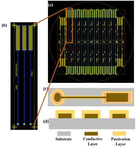
Figure 2-5 (a) The mask designed for fabrication of STE with circular electrode in CoventorWare10.4, (b) Zoomed-in vision of a single strip with 3 sperate circular electrodes, (c) 2-D representation of the top view of an electrode (the image is not to scale), (d) 2-d cross-sectional view of an electrode
