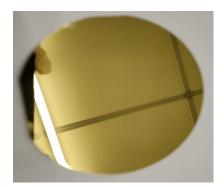
Figure 2- 12 TiW and Gold sputtered on a glass substrate
