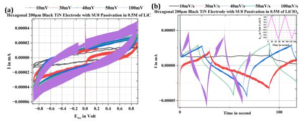
Figure 3- 63 For 200  $\mu$ m hexagonal black Tin electrode (a) The decrease in specific capacitance with the increase in scan rate, (b) redox reaction rate decreases with the increase in scan rate
