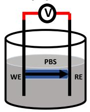
Figure 3-42 Schematic of an EIS in appropriate electrolyte
