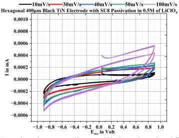
**Figure 3-61** CV performed in 400  $\mu$ m of hexagonal black TiN electrode in different scan rate
