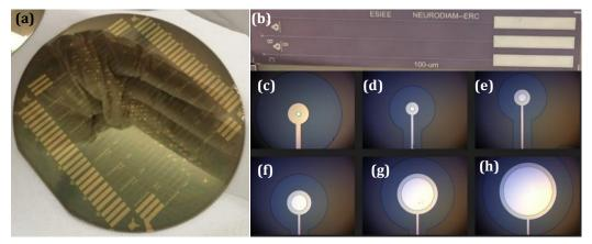
**Figure 2- 14** (a) Platinum electrodes of diameters (b) single strip of cicular Pt electodes on Si substrate with 3 indepent smaples (c) 30mm (d) 60m (e) 100μm, (f) 200μm, (f) 400μm, and (g) 600μm
