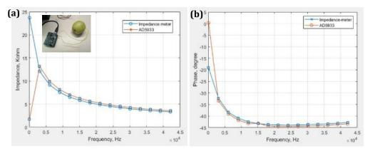
**Figure 3-7** (a) Comparison of the impedance measured of an apple with both the HP equipment and the AD5933 shield + Arduino, (b) phase measured of an apple with both the HP equipment and the AD5933 shield + Arduino
