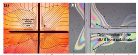
**Figure 1-17** (a) Deposition of collagen and other proteins from the culture media and neurons on the MEA (covered with SU8) substrate due to repeated use, (b) Delamination of the SU-8 master due to repetitive use [100]
