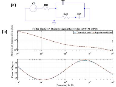
**Figure 3- 67** (a) Proposed equivalent circuit -3, (b) fit curves for this circuit in comparison with the experimental data
