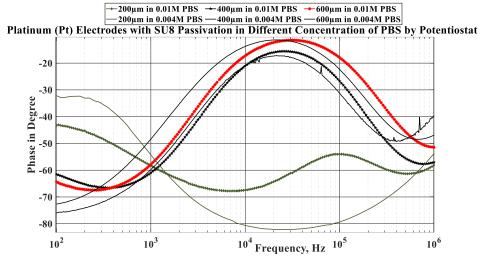
**Figure 3- 50** Impedance of 200  $\mu$ m, 400  $\mu$ m, and 600  $\mu$ m Platinum electrodes in different concentrations of PBS
