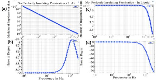
**Figure 3-22** EIS for simulation performed in Figure 3-21 considering imperfect passivation layer, (a) Impedance, (b) phase in air, (c) impedance, (b) phase in liquid with conductivity of 0.01 S/m and relative permittivity of 80
