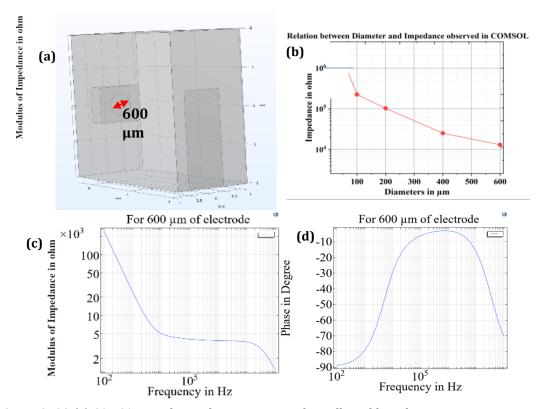
Figure 3-38 (a) COMSOL simulation done in 600  $\mu$ m of metallic gold conductive part against a reference electrode, (b) evolution of the impedance with the change in size observed at 1000 Hz, (c) the result from a sample in simulation environment
