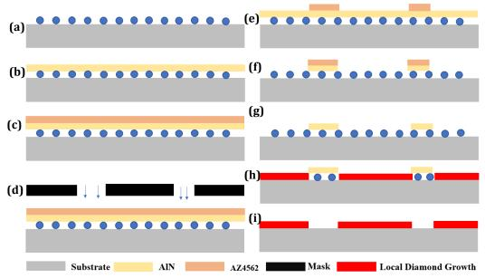
**Figure 2-22** (a) Nanoseeding, (b) AlN layer sputtering, (c) AZ4562 layer spincoating, (d) alignment and UV exposure, (e) uncovered AlN layer etched, (f) photoresist removal, (g) wafer inside the Diamond reactor, (h) local Diamond growth, (i) AlN etching
