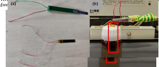
**Figure 4-7** (a) Samples with PCB and wire, (b) manual data collection with HP4194A; the samples are made stable to avoid perturbation during data collection
