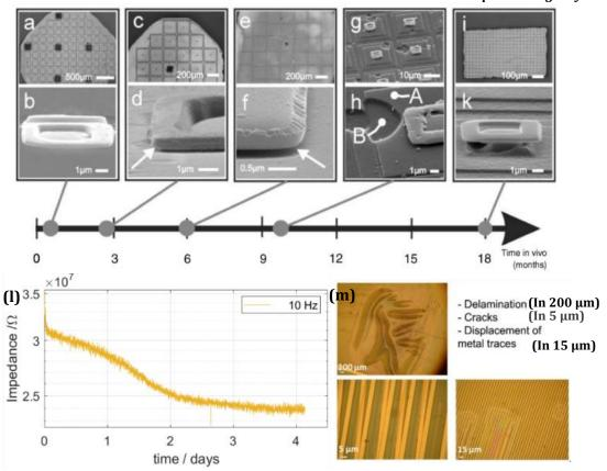
Figure 4-2 Micro-structure analysis of MPDA explanted from animals after 3 weeks to 18 months, (l) Real-time monitored impedance (at 10 Hz) during a soak test at an elevated temperature of 70°C, (m) Microscopy images of different failure types of barrel-activated test samples in gold IDE with PI encapsulation, scale bar shown in each image [252]
