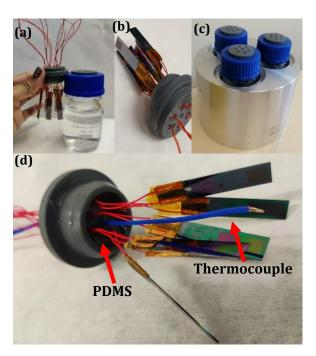
Figure 4-13 (a) the samples after attaching to the cap filled with PDMS, (b) the thermal mess and the glass jar placed in them and ready to be put on heat, (c) the caps with the samples and thermocouple, the red arrow shows PDMS poured inside the caps to make the system more hermetic (d) the samples in caps outside the glass jar that would be placed inside the thermal mess
