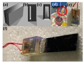
**Figure 4- 15** (a) Side, (b) front and (c) back view of the 3-D caps in the design layout, (d) the 3-D caps inserted and incapsulated in PDMS (red circle), (e)-(f) different views of the 3-D caps when the electrodes contact pads are installed inside
