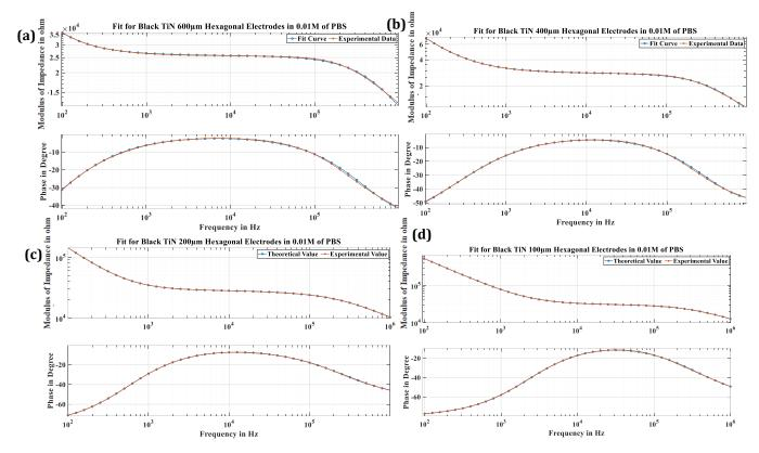
**Figure 3- 65** Experimental data plotted against fit parameter; blue curve – fit data, red curve – experimental data (a) 600  $\mu$ m, (b) 400  $\mu$ m, (c) 200  $\mu$ m, (d) 100  $\mu$ m of Black TiN electrode
