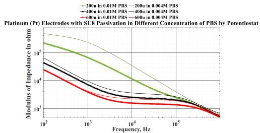
**Figure 3- 49** Impedance of 200  $\mu$ m, 400  $\mu$ m, and 600  $\mu$ m Platinum electrodes in different concentrations of PBS
