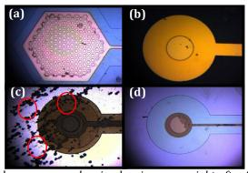
Figure 2- 28 All samples are seen under simple microscope right after fabrication without any treatment (a) 600 μm hexagonal TiN electrode on Si substrate with honeycomb structure on it, (b) 60 μm circular gold electrode on Si substrate (c) 200 μm BDD circular electrode with Diamond passivation on Si substrate (red circles show local Diamond growth), (d) 200 μm circular TiN electrode on Si substrate
