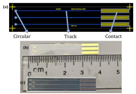
**Figure 2-6** (a) Zoomed-in view of a single sample of the mask (Circular electrodes) (b) a set of 3 separate gold electrode on a glass substrate, (c) a set of 3 separate Diamond electrode on a silicon substrate
