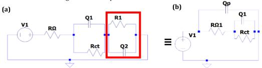
Figure 3-71 Equivalent circuit (a) and (b) has the same equivalent impedance
