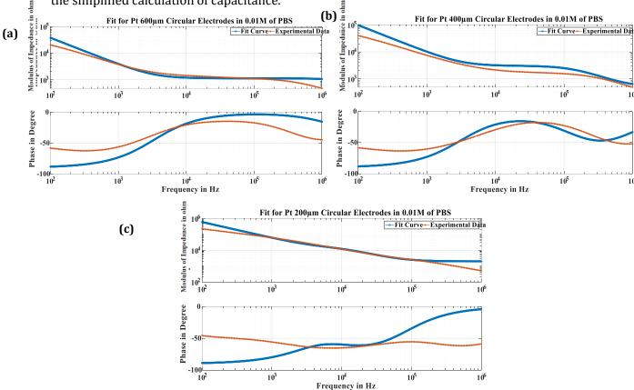
**Figure 3- 48** Experimental data plotted against fit parameter; blue curve – fit data, red curve – experimental data (a) 600 μm, (b) 400 μm, (c) 200 μm of Platinum electrodes
