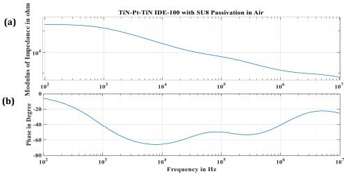
Figure 3-26 (a) Absolute value of impedance, (b) phase
