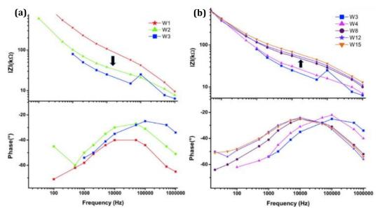
**Figure 4- 3** Bode representation of the impedance spectra recorded in vivo on 30 μm BDD electrode at (a) 1, 2, 3, (b) 4, 8, 12 and 15 weeks [275]
