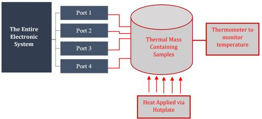
To achieve reliable measurement with the long-life setup, an important step was making a hermetic setup where the electrodes would be kept at a constant temperature to increase the effect of heating for a long period. A very well-established approach is to assume that the rate of aging is increased by a factor of  $2^{\Delta T/10}$ , where  $\Delta T$  is the temperature increase.
