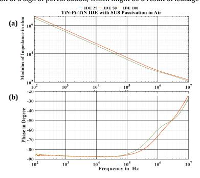
Figure 3-29 (a) Absolute value of impedance, (b) phase
