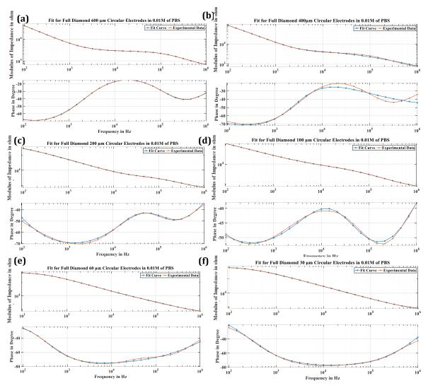
**Figure 3- 222** Experimental data plotted against fit parameter; blue curve – fit data, red curve – experimental data (a) 600 μm, (b) 400 μm, (c) 200 μm, (d) 100 μm, (e) 60 μm, (f) 30 μm of TiN-pt-TiN electrode
