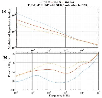
Figure 3-32 (a) Absolute value of impedance, (b) phase in 0.01M of PBS
