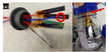
**Figure 4- 16** Red mark shows the origin of non-hermiticity in a thermocouple (b) possible misposition of the cap, which also might have contributed to the reduction of the water level due to lack of proper insulation
