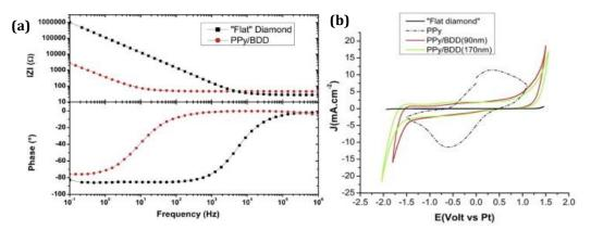
Figure 1-13 (a) EIS Bode representations of flat Diamond & BDD coated porous polypyrrole (PPy) in LiClO<sub>4</sub>Diamond electrode measured in 0.1 M LiClO<sub>4</sub>, (b) Voltammograms of the BDD coated porous polypyrrole (PPy) in LiClO<sub>4</sub> (a) voltammograms of (i) flat boron doped Diamond electrode, (ii) PPy film coated with a 90 nm thick BDD layer and (iii) PPy film coated with a 170 nm thick BDD layer, recorded in 0.1 M LiClO<sub>4</sub> at 100 mV/s [68]
