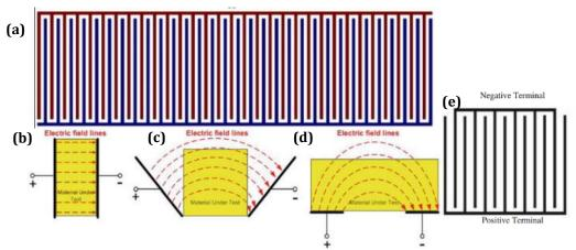
**Figure 2-2** (a) Structure of Interdigitated electrodes (IDE), (b) electric field lines of parallel plate capacitors, (c) electric field lines when the planes are moved further away from each other, (d) electric field line when the plates are at 360° apart from each other, (e)Configuration of a conventional coplaner IDE [133]
