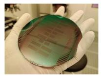
Figure 2-21 Just before putting in the reactor a sample with etched AlN
