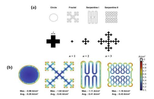
**Figure 2-9** Literature proves the power consumption Circular > Serpentine1 > Serpentine 2> Fractal, (a) different shapes of electrodes, (b) current distribution in different shapes of electrodes [68]
