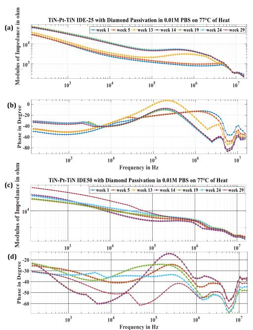
Figure 4-17 Data acquisition with AD2 from the samples with Diamond Passivation on heat (a) impedance, (b) phase of IDE with 25 pairs of fingers; (c) impedance, (d) phase of IDE with 50 pairs of fingers. Week 1 to 29 represent the time that the IDE is placed in PBS with temperature and week 29 is equivalent to around 9 years.
