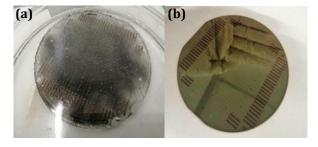
Figure 2-24 (a) Wafer being etched in etching liquid on heat, (b) wafer with etched TiN
