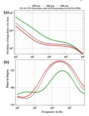
Figure 3-54 (a) Absolute value of impedance, (b) phase in samples of different diameters
