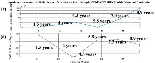
**Figure 4- 18** Trendline observed in samples' (a) impedance, (b) phase in IDE-25; (c) impedance, (d) phase in IDE-50 with Diamond passivation
