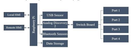
Figure 3-13 Functional diagram of the Multiplexer
