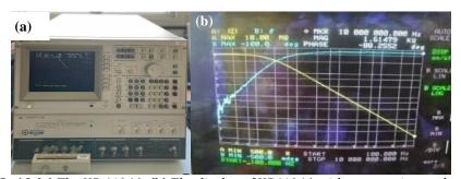
Figure 3-10 (a) The HP 4194A, (b) The display of HP4194A with an experimental result
