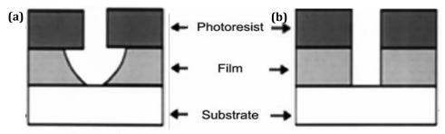
**Figure A-11** (a) Wet etching that helps acquire isotropic etching, (b) dry etching that helps acquire anisotropic etching [41]
