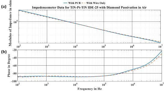
Figure 4-12 (a) Impedance and (b) phase
