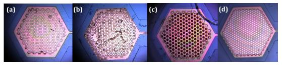
**Figure 3-74 (**a) Samples right after fabrication without any cleaning, (b) samples after using once and cleaning with cleaning method-1, (c) samples after using once and cleaning with cleaning method-2, (d) samples after fabrication and using the cleaning method-3
