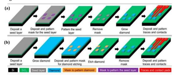
Figure 2-15 Schematic plots of the two typical microfabrication methods for making Diamond microelectrode arrays. (a) The bottom-up approach where Diamond electrodes are grown directly on a pre-patterned seed layer. (b) The top-down approach where a continuous Diamond film is grown on the seed layer followed by Diamond etching to form the electrode patterns [112]
