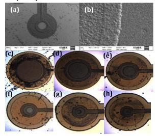
Figure 3-68 (a), (b) BDD electrode passivated with intrinsic Diamond seen under SEM, (c) 600 μm, (d) 400 μm, (e) 200 μm, (f) 100 μm, (g) 60 μm, and (h) 30 μm samples seen under simple microscope
