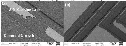
**Figure 3-35** Tear in the AlN layer during fabrication at different magnification (a) 10 μm scale, (b) 20μm scale
