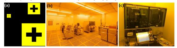
**Figure A-8** (a) Image of Alignment cross on the side of the mask in 2-D design file, (b) 58 m<sup>2</sup> area in class 100 dedicated to photolithography and substrate sealing, (c) Automatic alignment equipment in ESIEE Paris CLEANROOM [283]
