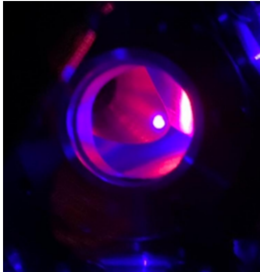
Figure 3.7: 3D blue MOT in steady state with repumpers on. According to [101], the atom number is estimated to be \sim 7 \times 10^6 .
