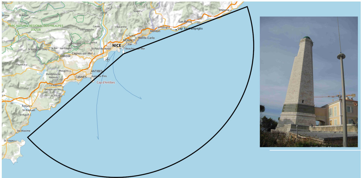
694 FIG. 1. Location and theoretical coverage of the SeaSonde CODAR installed in Saint-Jean Cap Ferrat. The 695 field of view is limited to the West by the Cape of Antibes and to the East by Cape Saint Ampelio. The arc of 696 circle marks a typical 65 km coverage. The SeaSonde mast at the lighthouse of Saint-Jean Cap Ferrat (upper 697 right).
