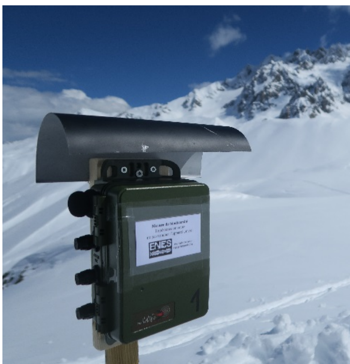
Figure 2.28 – Example of the type of audio recorder deployed on Flaine site (SM4, Wildlife Acoustics).
