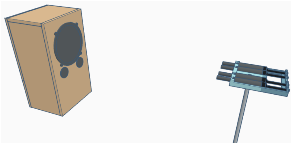
Figure 2.9 – 3D view of the calibration setup for the three microphones, with a reference microphone, in the source axis (distance scale not respected).
