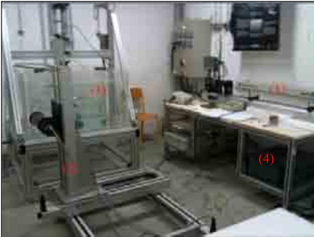
Figure (2.4): The Laser Doppler Velocimetry (LDV) testing apparatus, (1) Laser source. (2) Traverse system, (3) Tested tank, (4) Flow velocity analyser.
