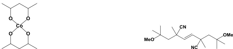
Figure 2 : Cobalt(II) acetylacetonate  $[\text{Co}(\text{acac})_2]$  et V-70 ou 2,2'-Azobis(4-methoxy-2,4-dimethyl valeronitrile).
