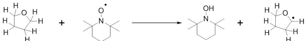
Figure 84: Putative reaction of THF and (2,2,6,6-Tetramethylpiperidin-1-yl)oxyl (TEMPO) to give  $\text{TEMPO}^{\text{H}}$  and tetrahydrofuryl radical.
