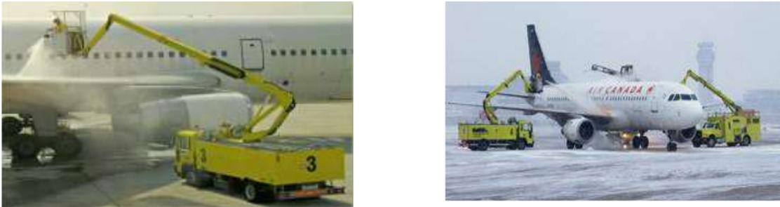
Figure 1.10: On-going de-icing process
