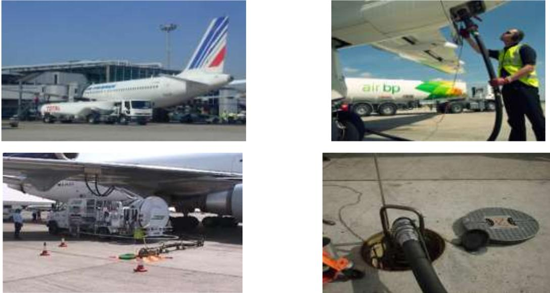
Figure 1.7: Different aircraft fuelling processes
