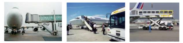
Figure 1.3: Different devices to handle passengers boarding and de-boarding processes
