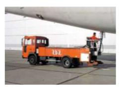
Figure 1.9: Potable water supply process
