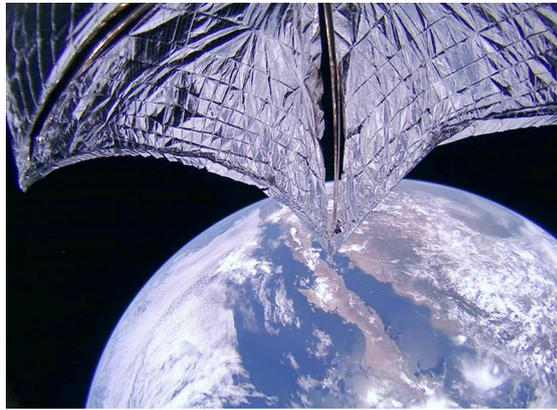
Figure 1.2: LightSail 2 selfie with the deployed solar sail.
