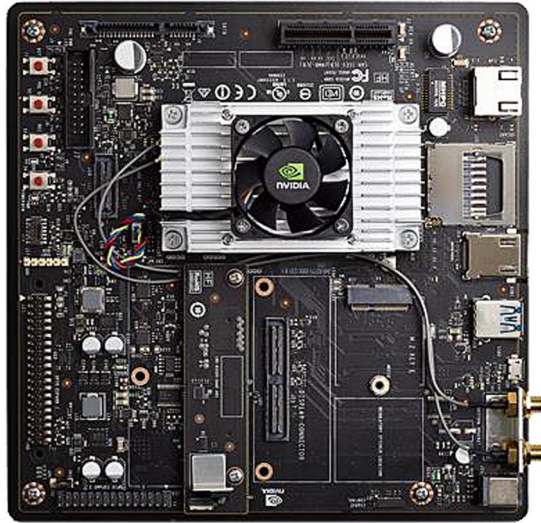
Figure 2.2: An overview of the NVIDIA Jetson TX2, which was utilised in our experiments. See section 4.6.1.
