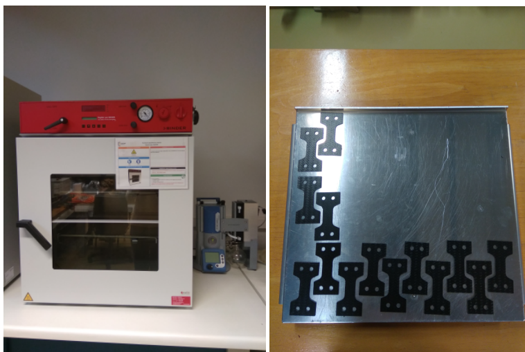
(a) Desiccator BINDER Vacuum drying chamber (b) Specimens placement on racks
