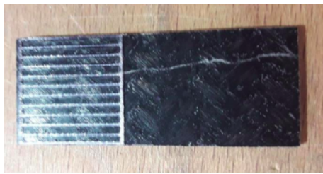
Figure 3.4 – Integration of energy directors on a specimen used for the processing parameters definition
