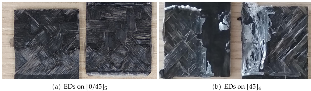
Figure 3.10 – Post-fracture SLJ [0/45]_S/[45]_4 specimens - study on the welding energy
