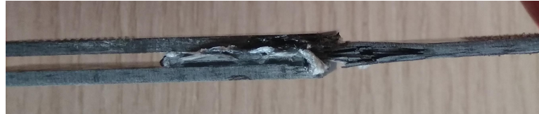
Figure 3.11 – Substrate fracture of DLJ specimen
