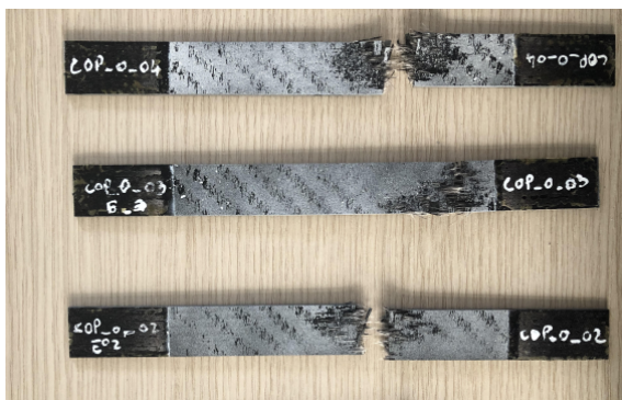
Figure 2.20 – Post-mortem specimens - tensile tests on [0]_4
