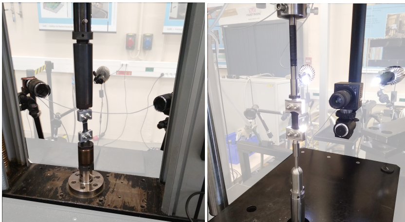
(a) SLJ specimen on the quasi-static test machine (b) SLJ specimen on the dynamic tensile test machine
