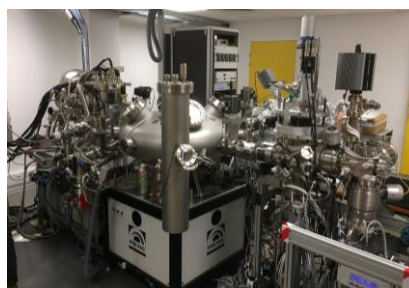
Figure 2-8. XPS apparatus used in this study
