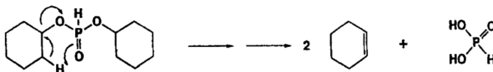
Figure 5-18. The pyrolysis mechanisms of di-cyclohexyl hydrogen phosphite (cHPi) [16].
