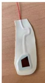
Figure 4.3 p-GaP photoelectrode as prepared in this work.
