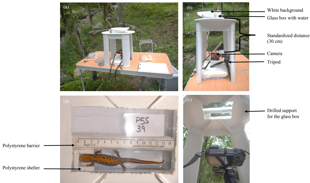
Figure 2. Photography set up for ventral pattern recognition of the Pyrenean brook newt, located close to the river bank (a and b). Individuals are placed in the glass box placed on a drilled support, between the barrier and the side of the glass box, and covered by a white background (c and d). They are photographed from below with a tripod-mounted camera placed at a standardized distance of 30 cm below the glass box.
