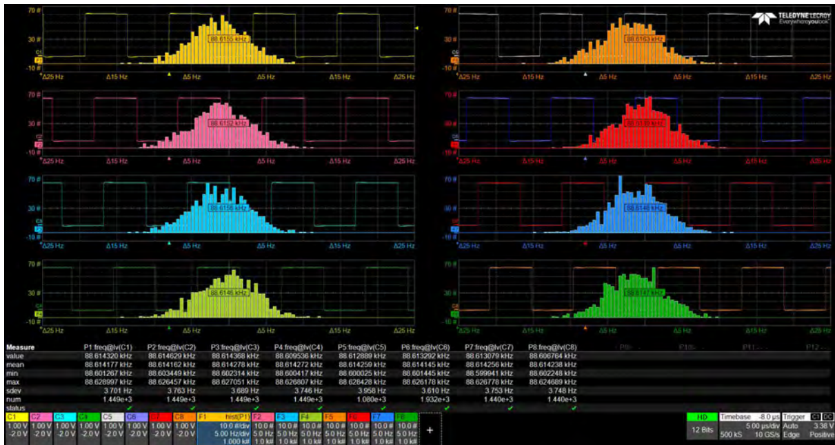
Figure IV-32 – Noise immunity: frequency jitter measurement.
