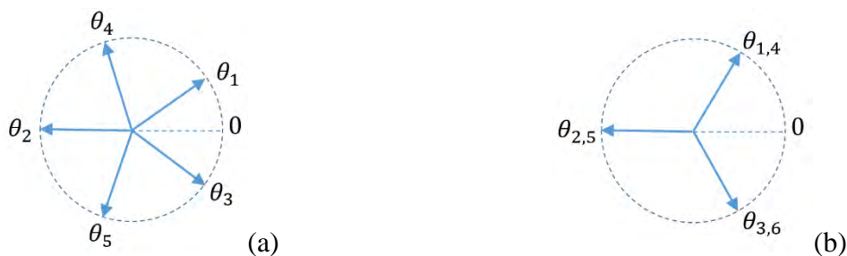
Figure II-18 – Interleaving issue when phase differences are equal to 2/N : a) N odd case ( N = 5 ), b) N even case ( N = 6 ).
