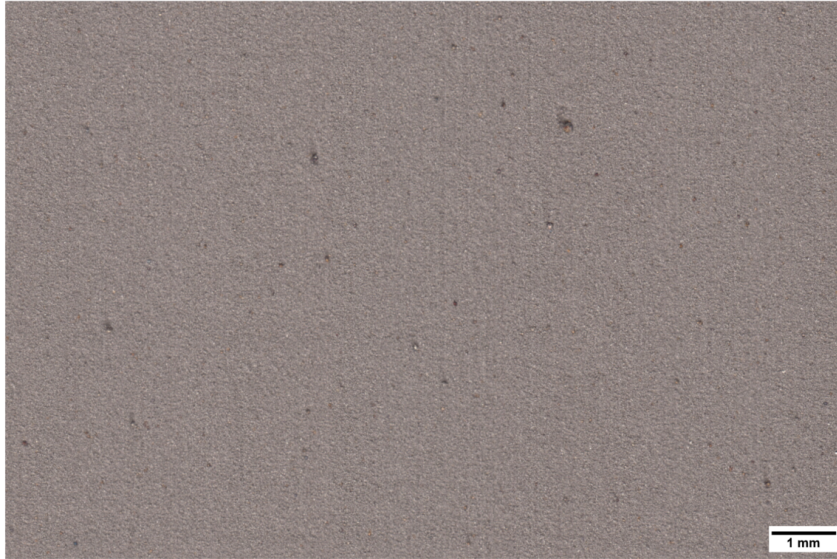
Figure 4.20 – Powder bed scan of un-sieved powder after one printing cycle (P1-u) displaying large spatters on the surface.
