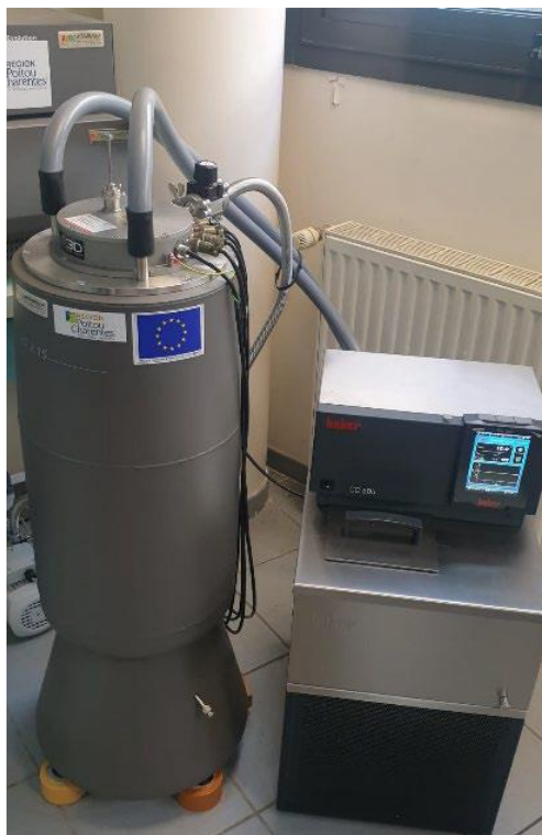
Fig. 3.10. Scheme of the Calvet calorimeter.
