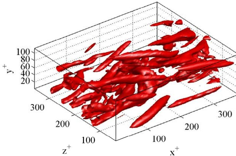
Figure 3.6: Coherent structures visualized by the  $\lambda_2$ -criterion for the single-phase case at  $Re = 1575$  before the flow relaminarizes. The magnitude of the contours shown here is equal to four times the standard deviation.
