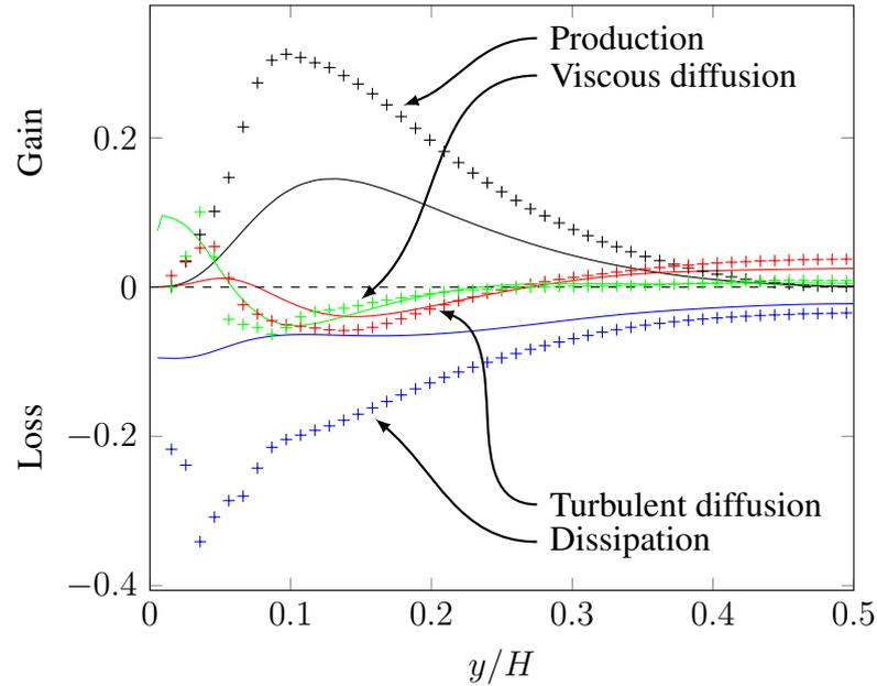
Figure 3.17: Different contributions to the budget of  $\overline{\langle u^2 \rangle}$  plotted in half of the domain for  $Re = 1575$ . Solid lines stand for the single-phase case and symbols are for the two-phase case. Normalized by  $u_*^4/\nu$ , with  $u_* = \sqrt{0.5 C_f \langle u \rangle^2 / \rho}$ .
