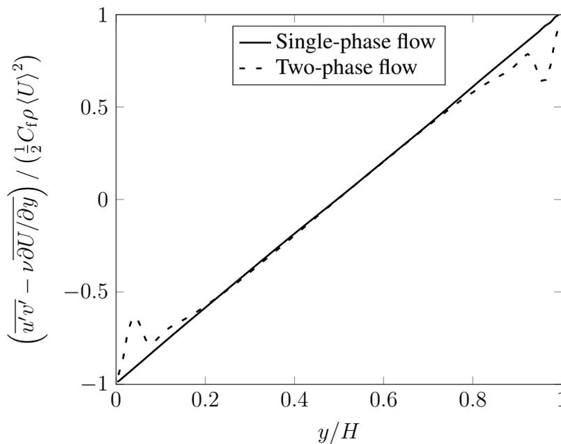
Figure 3.10: Total shear stress  $\tau_{xy}$  profiles at  $Re = 1575$ .
