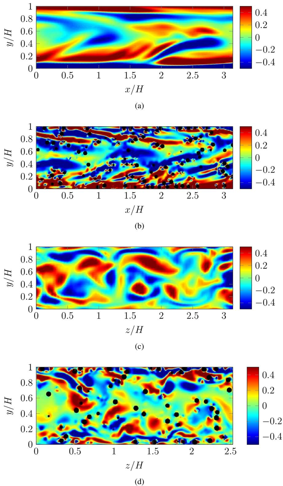
Figure 3.15: 2D slices of (a–b) spanwise  $\omega'_z$  and (c–d) streamwise  $\omega'_x$  vorticity fluctuations at  $Re = 1575$  in the median section of the simulation domain. The fluid is flowing from left to right in (a–b). (a–c) and (b–d) correspond to single and two-phase flows, respectively.
