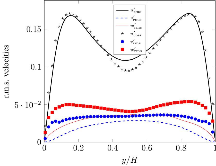
Figure 3.13: Profile of the r.m.s. velocity fluctuations scaled by  $\langle U \rangle$  at  $Re = 1575$ . Symbols stand for two-phase flows, in the flow ( $\star$ ), wall normal ( $\bullet$ ) and spanwise ( $\blacksquare$ ) directions. Lines present the results of single-phase flow simulations in the flow (solid), wall-normal (dashed) and spanwise (thin line) directions.
