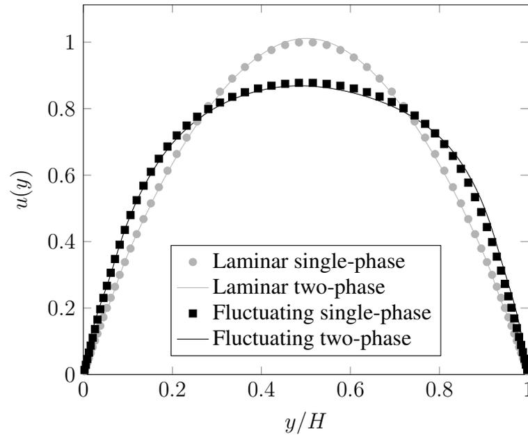
Figure 3.9: Average velocity profile of fluctuating flows at  $Re = 1575$  (thin line for single-phase flow and square symbols for two-phase flow) and of laminar flows (solid line for single-phase flow and circle symbols for two-phase flow).
