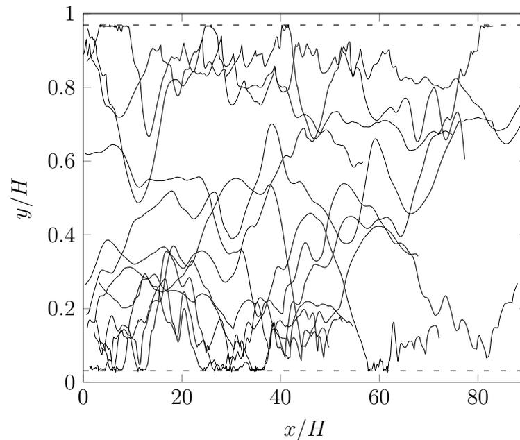
Figure 3.7: Sample of particle trajectories projected in the flow-shear plane  $(x, y)$  at  $Re = 1575$ . The horizontal solid lines indicate the wall positions. Horizontal dashed lines indicate the position of the particle center when the particle starts to overlap the wall.
