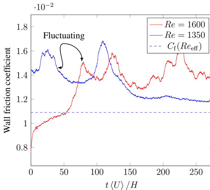
Figure 3.19: Temporal evolution of the wall friction coefficient for  $Re = 1350$  and  $Re = 1600$  obtained respectively from turbulent-to-laminar and laminar-to-turbulent transition. The dashed line is the laminar prediction at  $Re_{eff} = 1130$  which corresponds to the  $Re = 1350$  simulation.
