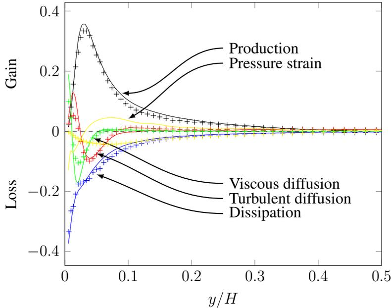
Figure 3.16: Kinetic-energy balance of  $\overline{u'^2}$  normalized by  $u_*^4/\nu$  ( $u_*$  being the friction velocity) and plotted in the lower half of the domain for  $Re = 6000$ . Solid lines stand for a resolution of  $64^3$  meshes while symbols are for a meshing of  $256 \times 100 \times 258$  meshes.
