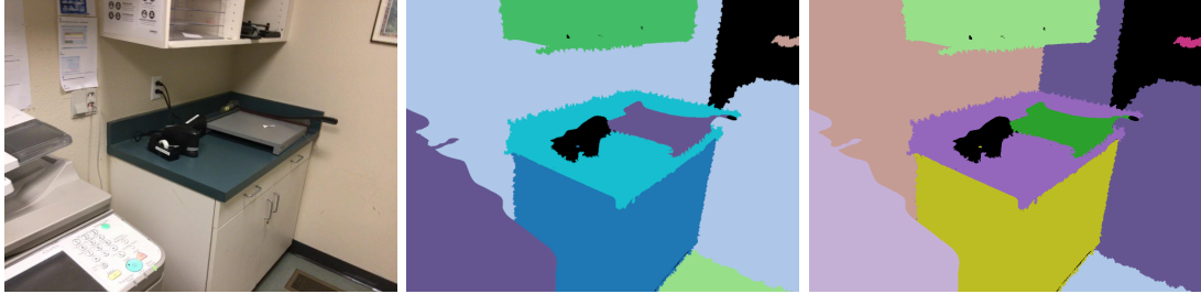
FIGURE 5.18: Frame from a ScanNet [37] sequence (left), semantic segmentation (middle) and instance segmentation (right). The “walls” –semantically represented by a uniform (pale blue) region– are broken up into two distinct (pale orange and purple) instances.
