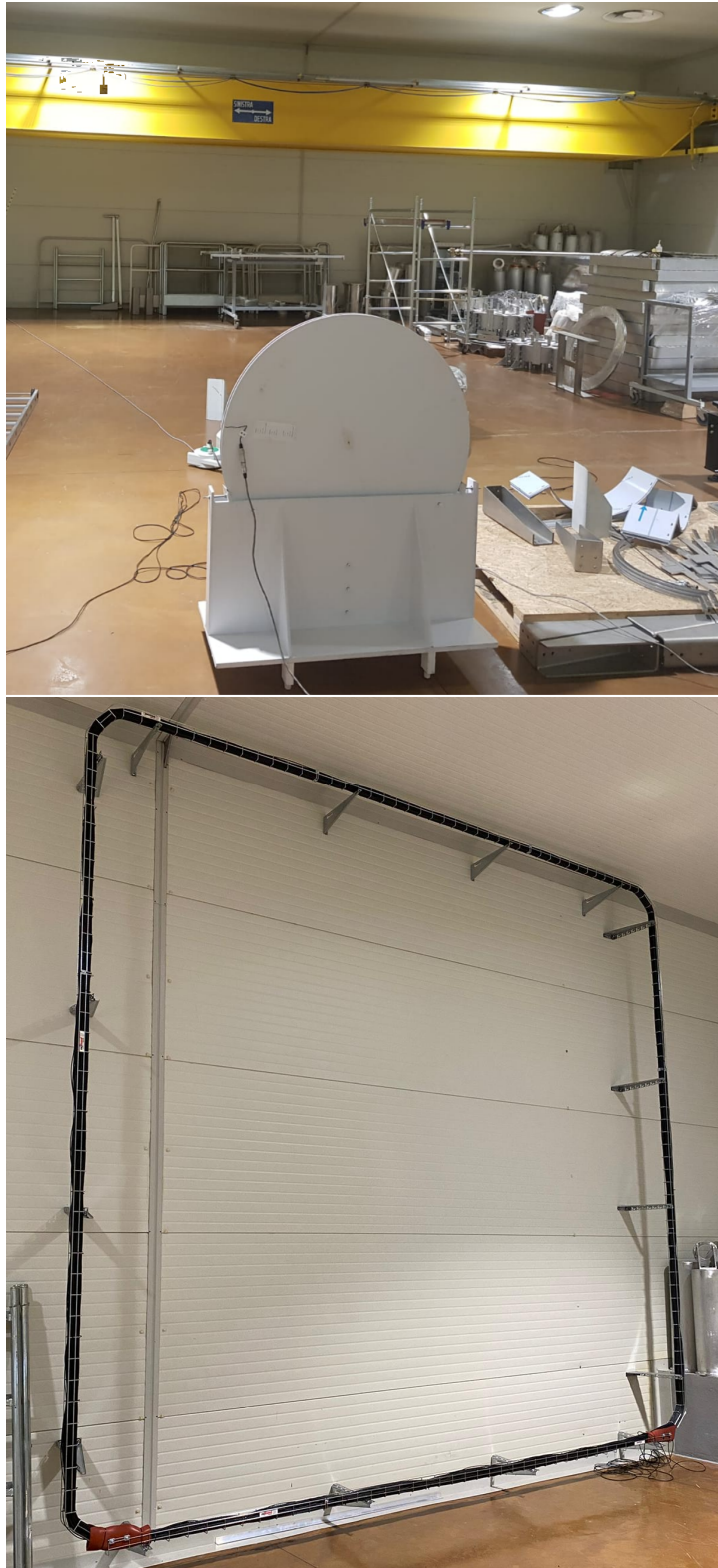
Fig. 7.5.: Top: the 1m-diameter, circular coil used for magnetic injections during O3. Bottom: the new coil in Virgo's CEB, planned to be used during O4. Note the wall to which this coil is attached is the same as the wall in the back of the top photo.
