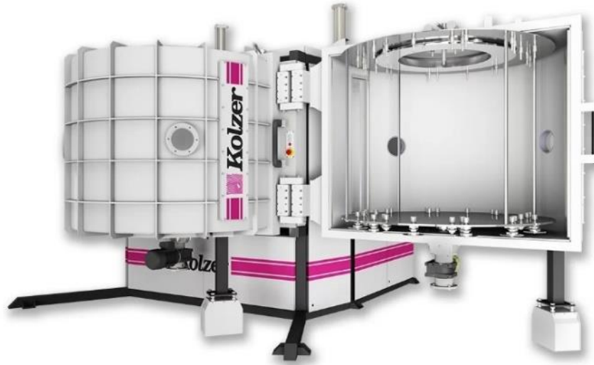
Figure III-3: Industrial PECVD equipment, provided by Kolzer SRL 23 .
