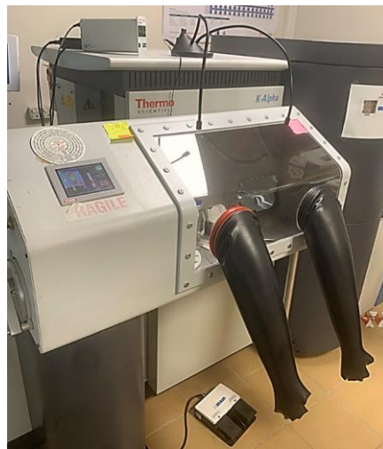
Figure 4: Thermo K-alpha spectrometer used for all XPS analysis.
