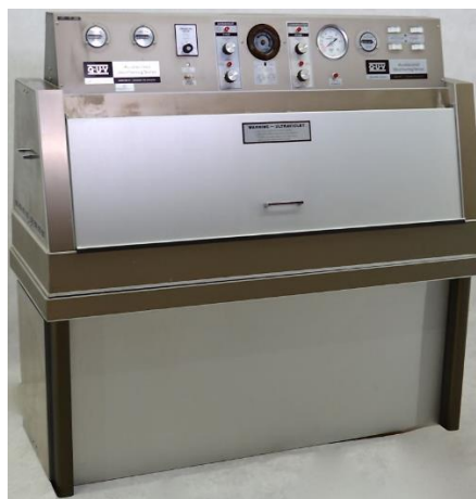
Figure IV-8: UV ageing test chamber from Q-Panel Company used for the tests.
