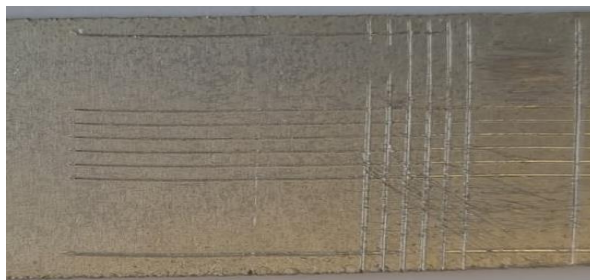
Figure II-21: Adhesion test results for NDR hybrid coating.
