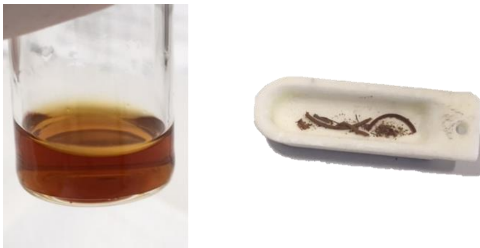
Figure I-10: Hybrid Lignin/Silicon solubilized and after dry, forming a dark brown powder.
