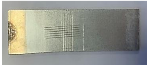
Figure IV-16: Adhesion test from DR hybrid coating exposed to UV ageing.
