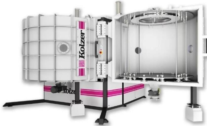
**Figure III-3:** Industrial PECVD equipment, provided by Kolzer SRL<sup>23</sup>.
