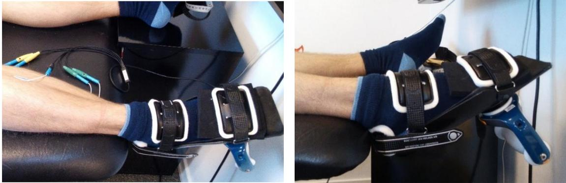
*Figure 38. Dispositif PSAD (Portable Spasticity Assessment Device), position flexion plantaire (P1)*
