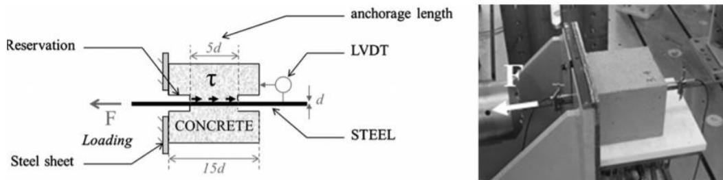
Figure 2.3 Pull-out set up (Torre-Casanova et al., 2013)
