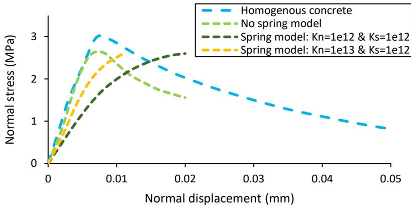
Figure 5.5 Normal stress versus normal displacement for uniaxial tensile tests performed on the homogenous concrete sample using the values listed in Table 4.4 for Mazars model parameters, and on CubeA by taking  $E_{mor} = 23 \text{ GPa}$ , with linear spring model for the mortar-aggregates interface; Stiffnesses are in  $\text{N/m}^3$
