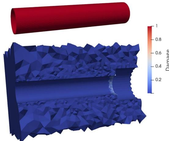
*Figure 4.15 Distribution of damage in the concrete and the interface at the end of the simulation ( $FED = 3.6$  mm) for the reference simulation performed on the smooth sample using FCZM*
