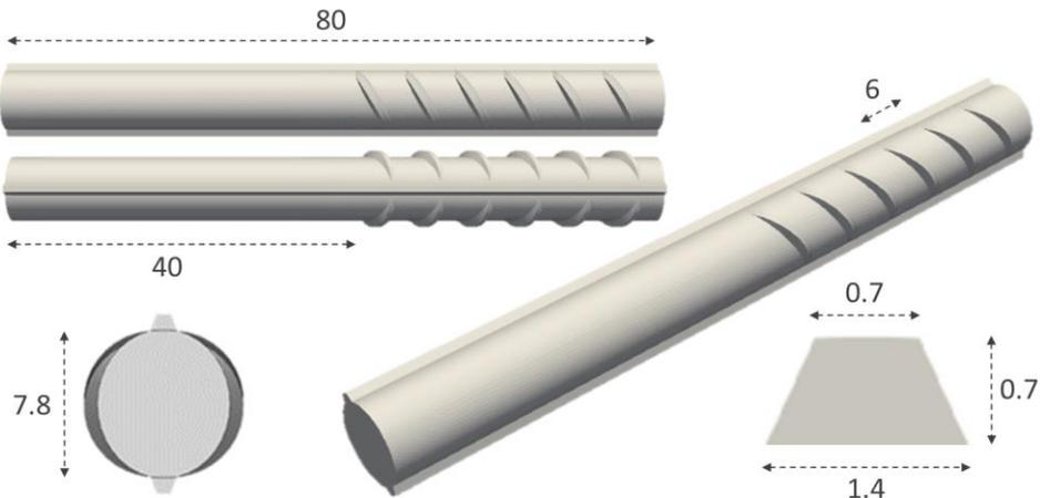
Figure 4.12 Dimensions of the modelled spiral steel bar (in mm)
