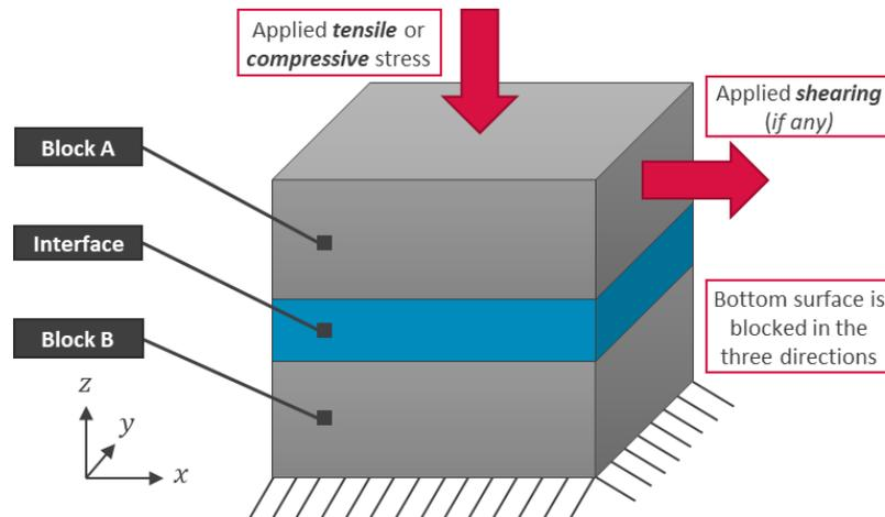
Figure 3.17 Geometric model for the one-interface element simulations
