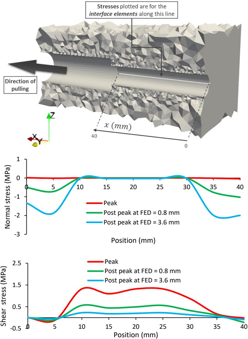
Figure 4.16 Normal stress, and the shear stress in the direction parallel to the axis of the steel bar, in the steel-concrete interface elements at three different FED for the reference simulation
