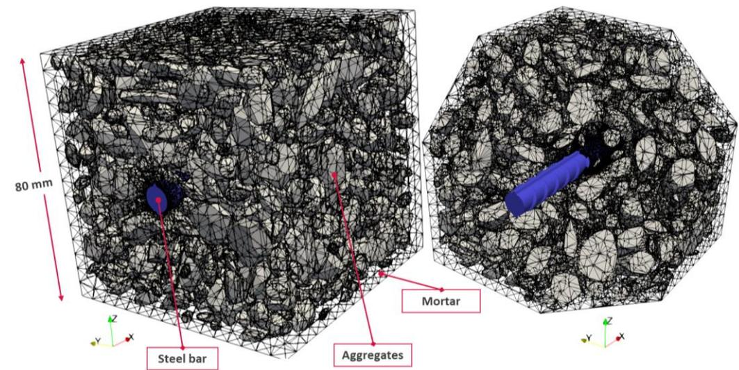
Figure 5.2 Visualization of sample SAgg3, showing the aggregates phase (in white), ribbed steel bar (in blue) and mortar (transparent)
