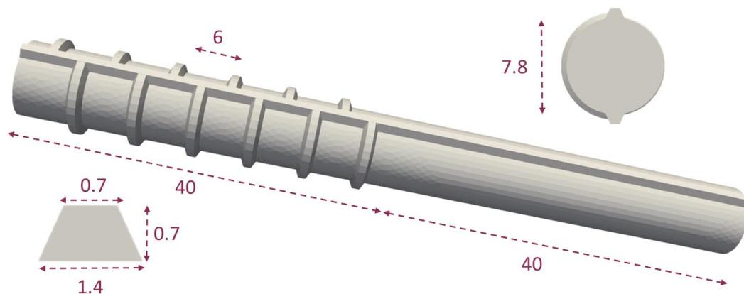
Figure 5.22 Dimensions of the modelled herringbone steel bar (in mm)
