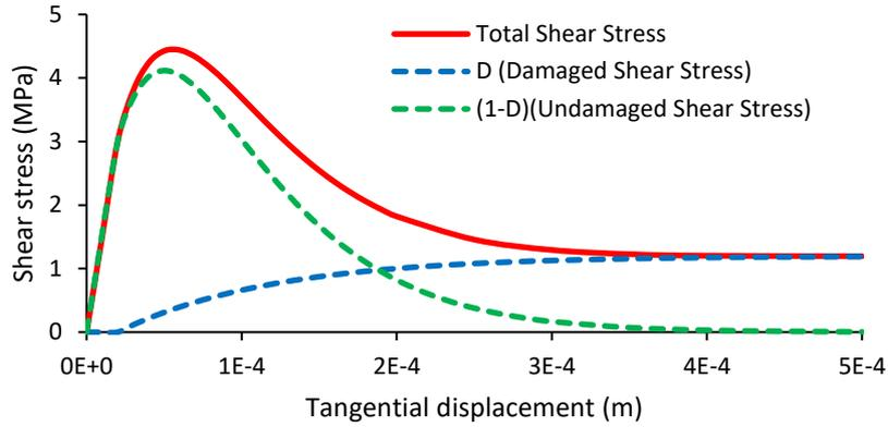
Figure 4.3 Total shear stress, damaged part's shear stress and undamaged part's shear stress versus tangential displacement for the frictional cohesive zone model under -3 MPa compressive stress
