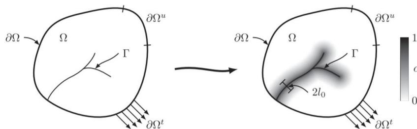
Figure 2.8 Schematic depiction of the phase field method, in which the crack is modelled by the field  $c$  where a black color corresponds to a fully damaged material ( $C = 1$ ) and a white color corresponds to a fully intact material ( $C = 0$ ); the  $l_0$  parameter controls the width of the process zone (Arriaga and Waisman, 2018)
