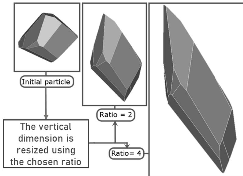
Figure 3.3 Resizing one dimension of a polyhedron particle
