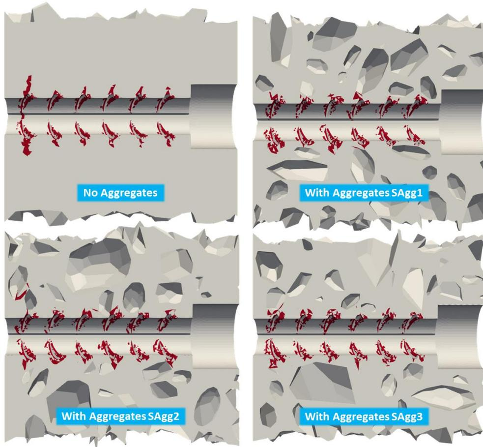
Figure 5.11 Full damage ( $D \geq 0.99$ ) in concrete for the homogenous case, and in mortar for the three heterogeneous cases, at the central plane normal to the z-axis of the extracted volume, when bar's displacement is 1 mm
