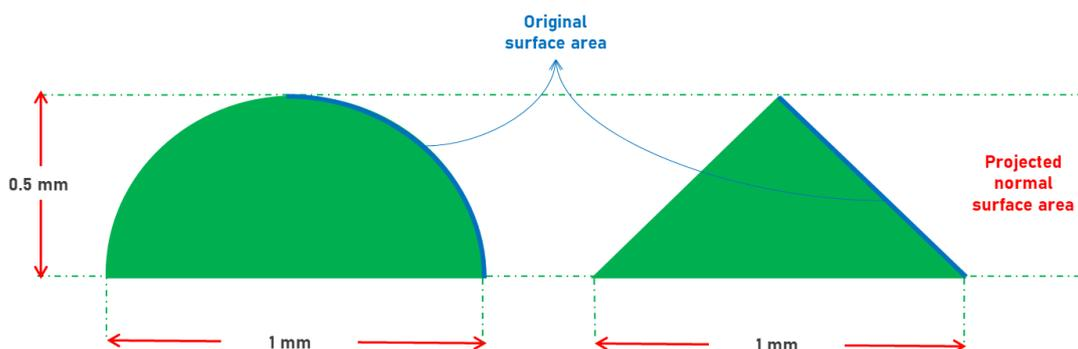
Figure 5.26 Original surface area (in blue) and projected surface area (in red) in 2D for a semicircular rib and a triangular rib used in (Higuchi et al., 2022)
