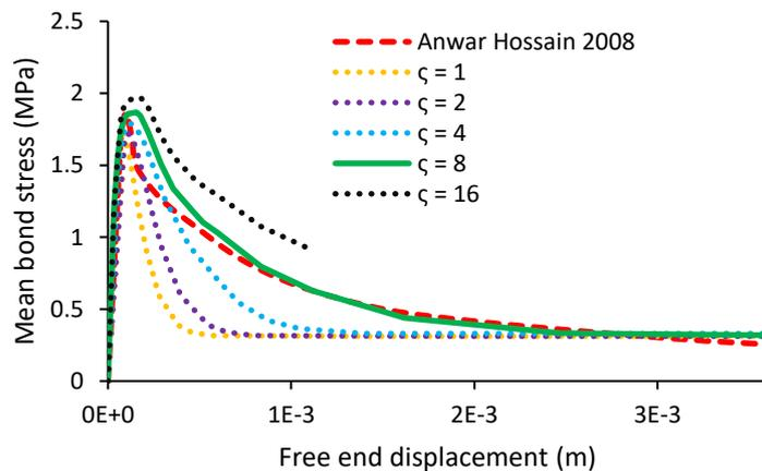
Figure 4.10 Mean bond stress versus free end displacement for the numerical simulations performed on the sample having a smooth bar and the experimental results extracted from (Anwar Hossain, 2008) by varying  $\zeta$
