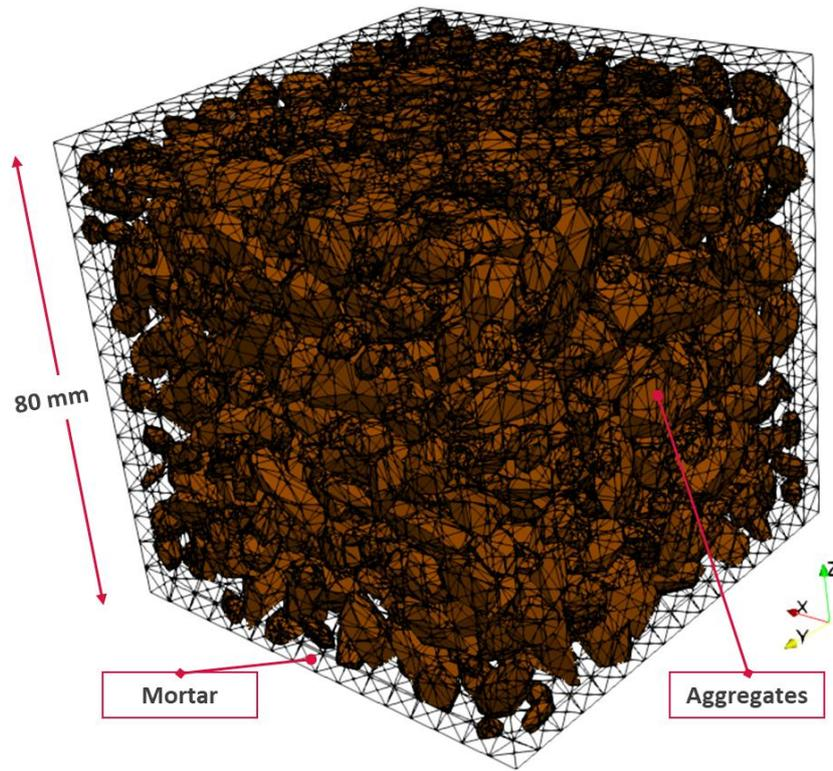
Figure 5.3 Visualization of sample CubeB, showing the aggregates phase (colored) and mortar (transparent)
