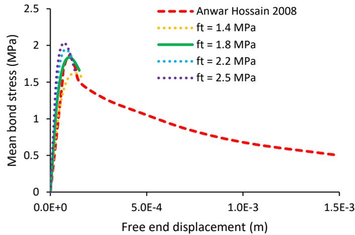
Figure 4.8 Mean bond stress versus free end displacement for the numerical simulations performed on the sample having a smooth bar and for the experimental results extracted from (Anwar Hossain, 2008) by varying  $f_t$
