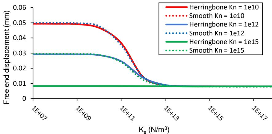
Figure 3.11 Variation of the free end displacement as a function of the shear stiffness for the herringbone sample and the smooth sample; normal stiffness  $K_n$  is fixed at  $10^{10}$  ,  $10^{12}$  and  $10^{15} \text{ N/m}^3$  in each group, and the final imposed displacement is 0.05 mm
