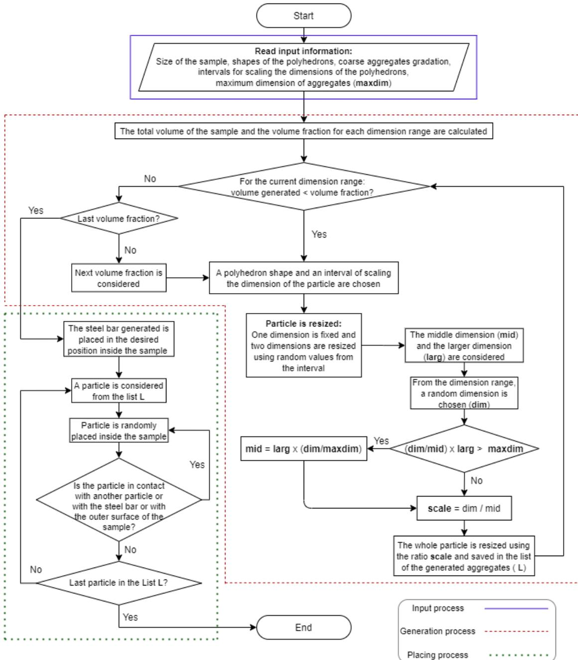
Figure 3.4 Flowchart to generate and place the aggregates
