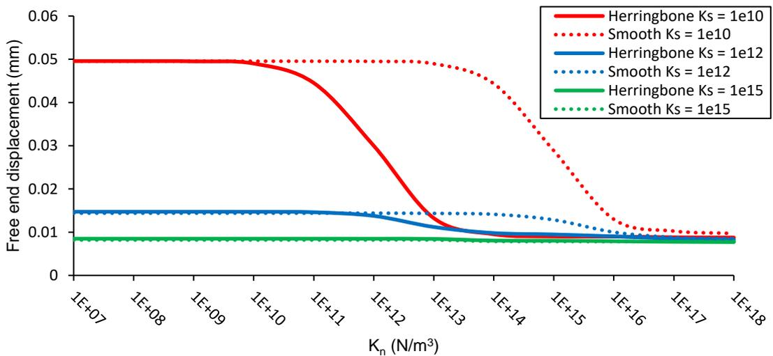
Figure 3.12 Variation of the free end displacement as a function of the normal stiffness for the herringbone sample and the smooth sample; shear stiffness  $K_s$  is fixed at  $10^{10}$ ,  $10^{12}$  and  $10^{15} N/m^3$  in each group, and the final imposed displacement is 0.05 mm
