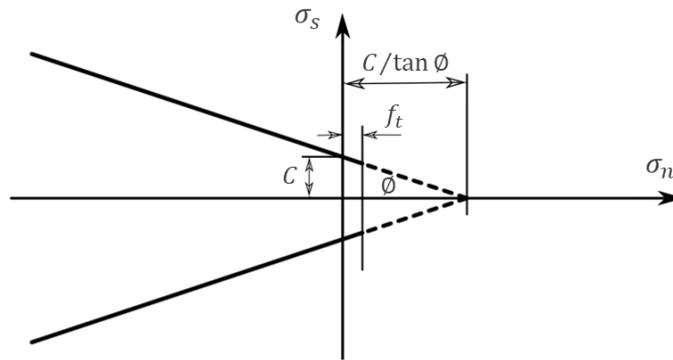
Figure 3.16 Mohr-Coulomb's failure criterion for the Coulomb's interface model
