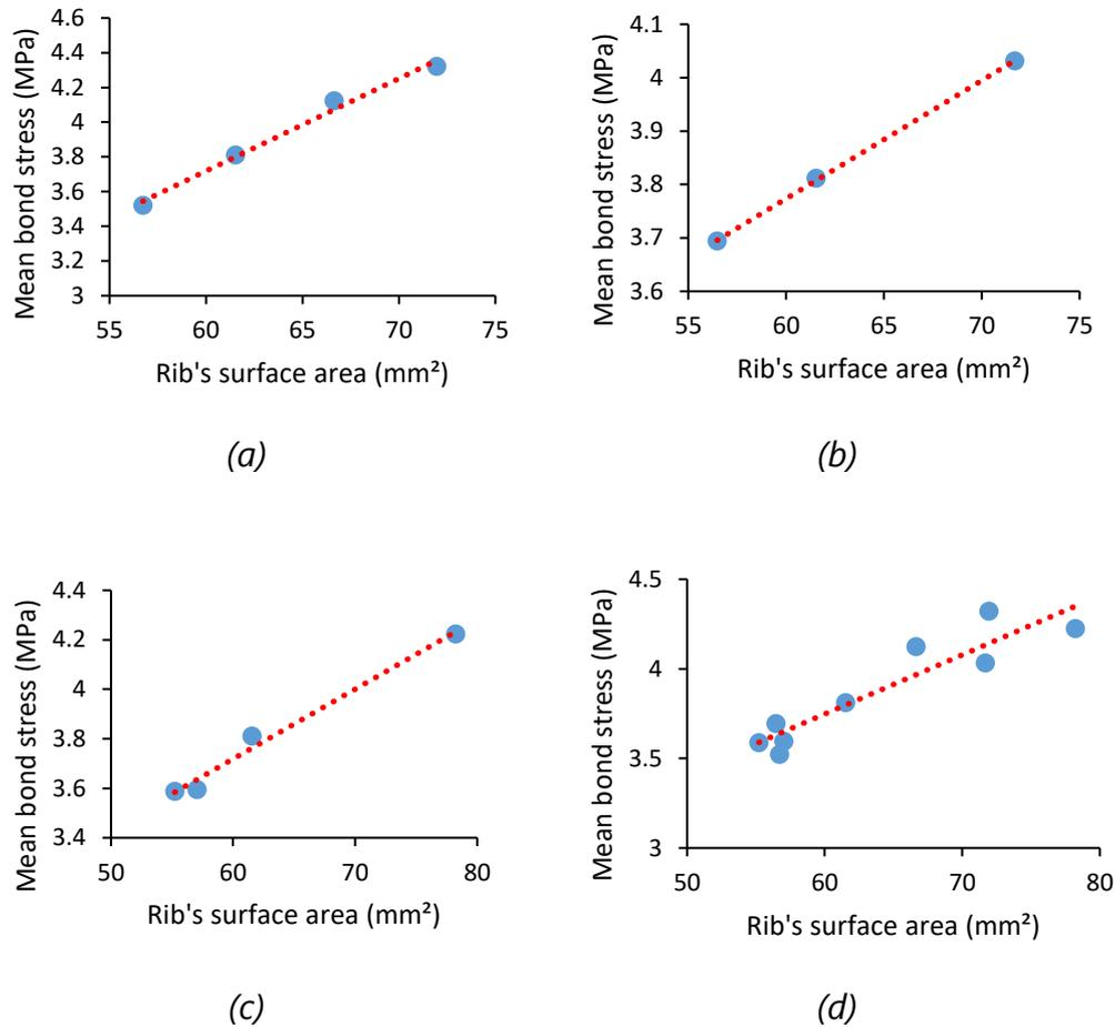
Figure 5.18 Mean bond stress, at  $FED = 2$  mm, versus rib's surface area for the groups of samples having the following pattern: (a) varying rib's height; (b) varying rib's smaller and larger width equally; (c) varying rib's angle (d) all three groups together
