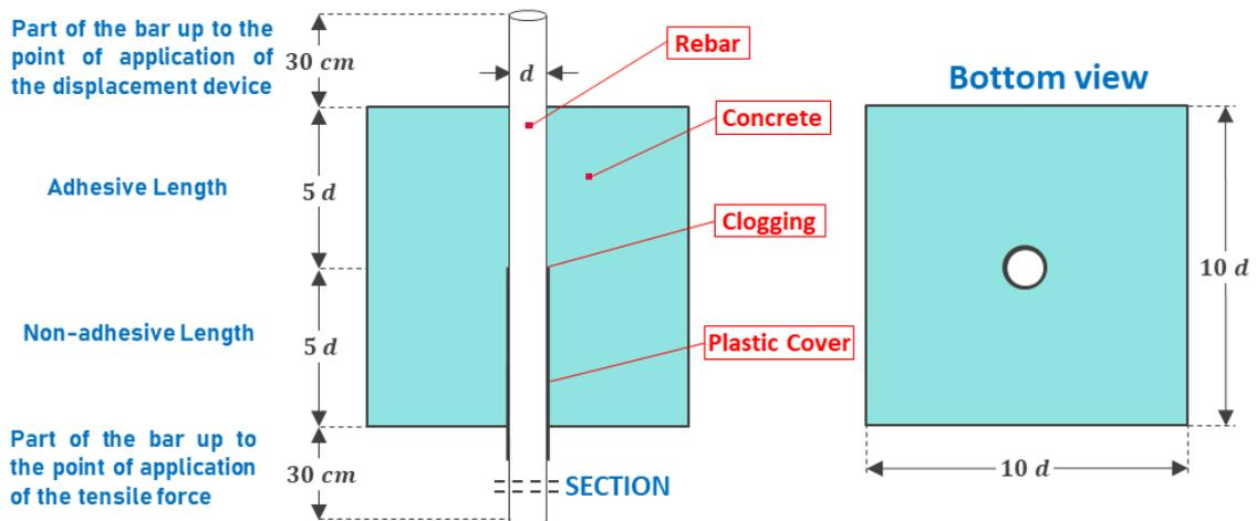
Figure 2.1 Description and dimensions of the test piece, based on (RILEM, 1970)
