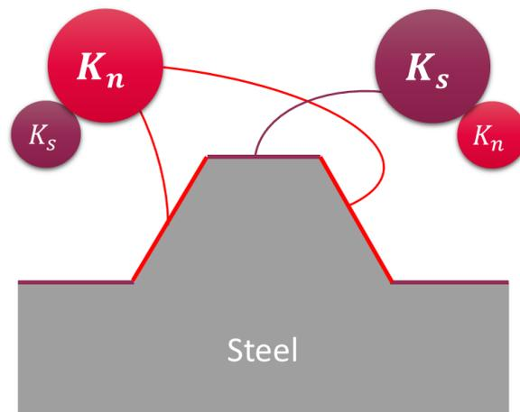
Figure 3.10 The dominating parameters at and near a rib of a steel bar
