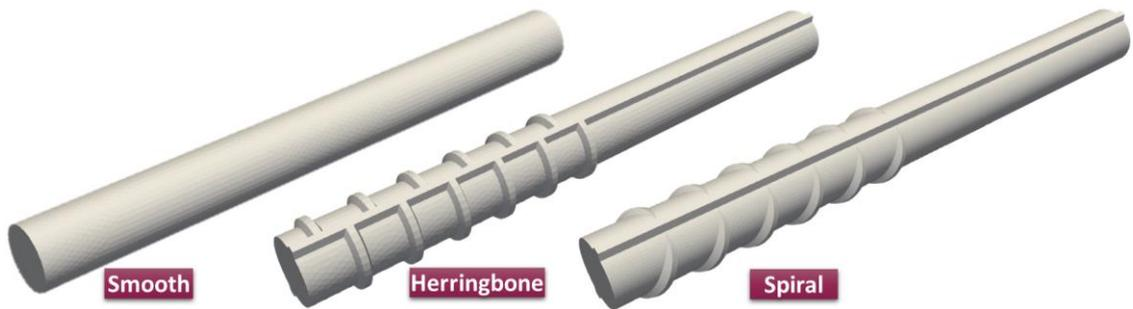
*Figure 3.1 The three modelled steel bars; smooth bar, herringbone-ribbed bar and spiral-ribbed bar*
