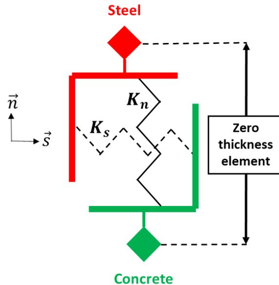
Figure 2.9 Normal and shear spring stiffnesses between a steel element and a concrete element
