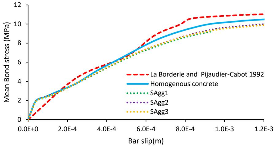
Figure 5.8 Mean bond stress versus slip for the homogenous pull-out test discussed in subsection 4.3.3.2, and for the heterogeneous pull-out test simulations performed on samples SAgg1, SAgg2 and SAgg3
