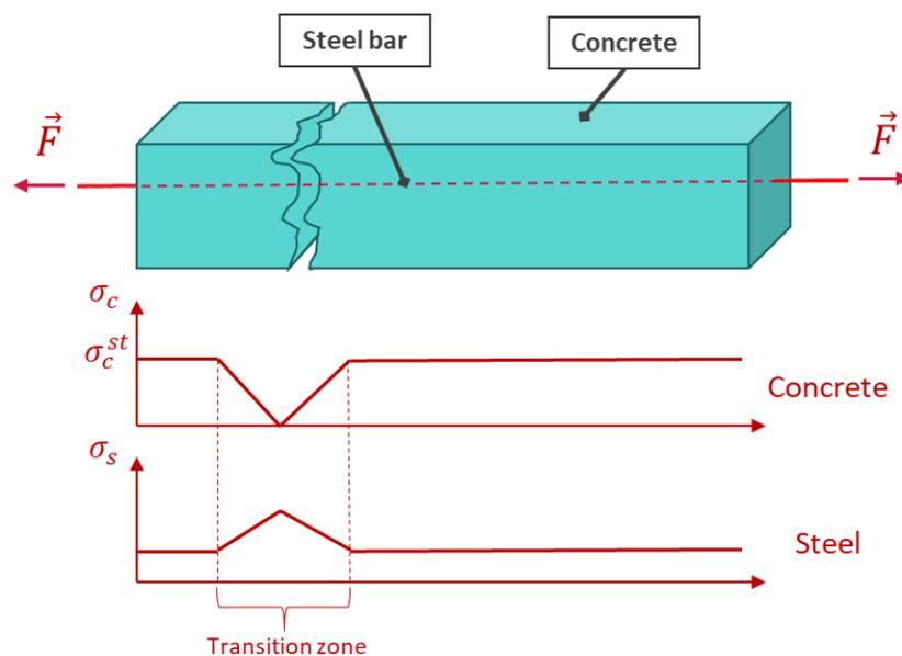
Figure 1.1 Distribution of stresses in steel and concrete in a reinforced concrete tie after the first crack;  $\sigma_c$  and  $\sigma_s$  are the stresses in concrete and steel respectively, and  $\sigma_c^{st}$  is the concrete strength, based on (Casanova et al., 2012)
