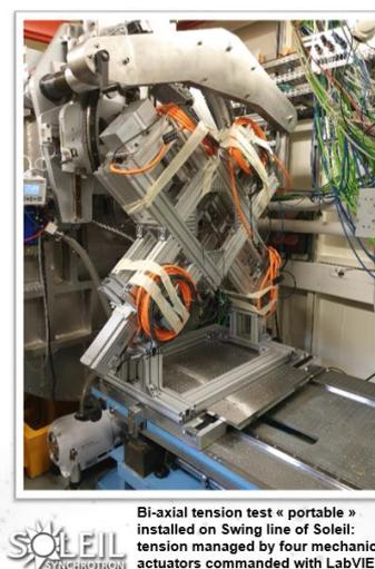
during the heating and stretching stage. Biaxial stretching of the sample is then provide at a maximum speed of  $450\text{m}\cdot\text{s}^{-1}$ . The force is controlled with the LabView programming software. The displacement field can be followed from a high speed camera and the strain field can be determined using the digital image correlation technique.
