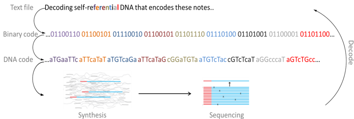
Figure 1. 21: Depiction of strategy followed for storing digital information in DNA form and each sequential retrieval by sequencing techniques.
