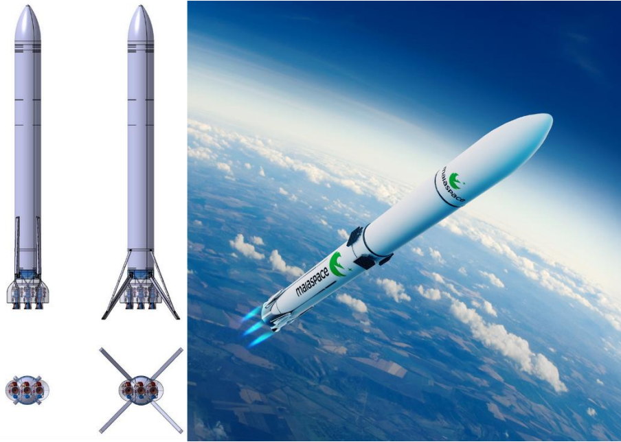
Figure 4: THEMIS methalox demonstrator developed by ArianeGroup (left) and reusable launch vehicle based on THEMIS proposed by MaiaSpace (right) [18]
