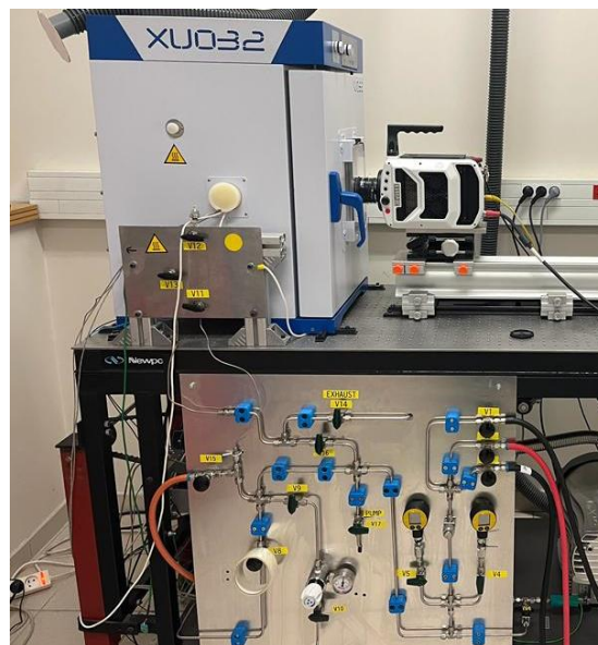
Figure 22: The complete OPTIPRIME experimental setup in its furnace with its filling system and high-speed camera
