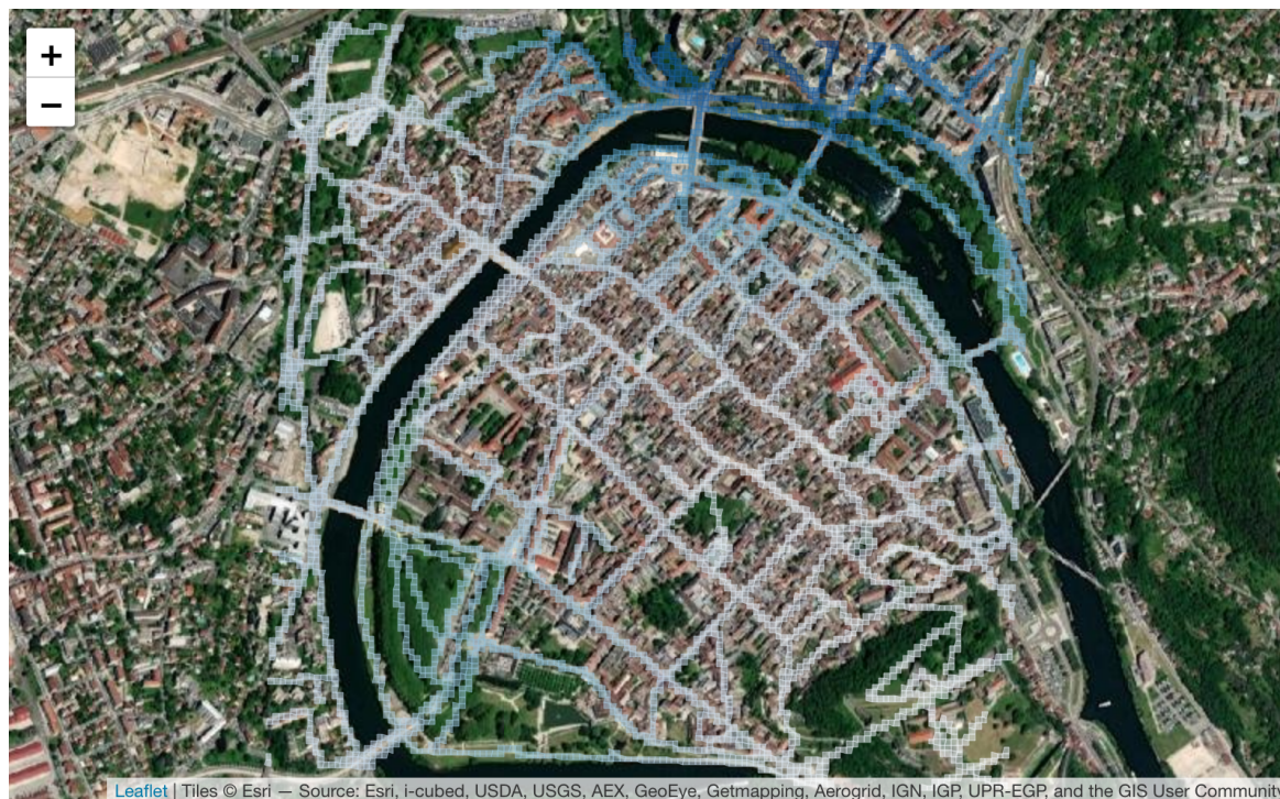
FIG 4.12: Kernel estimate of intensity for the road crashes of Besançon city centre. With package leaflet .
