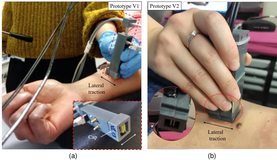
Figure 4.14: Setup for *in vivo* tests. (a) Example of forearm tests with prototype V1. A customized cap is used to allow 1 mm indentation depth of the bender tips on the skin surface. (b) Example of lower back tests with prototype V2. The indentation depth is adjustable so that the exerted normal force is within the test range.
