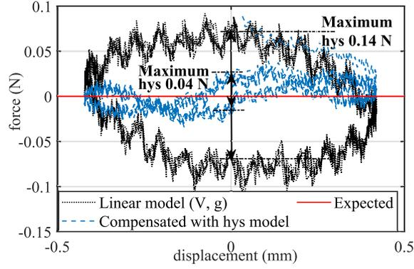
Figure 3.11: Hysteresis compensation using a hysteresis model. The piezoelectric bender was driven by a full-scale sinusoidal voltage at 1 Hz with its tip free. The tip force is expected to be null. The black dot curve is estimated from the linear model  $(V, g)$ , following equation (2.15). The blue dash curve shows the compensation results with the hysteresis model, following equation (3.10).
