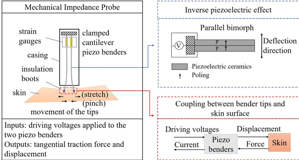
Figure 2.1: Scheme of the portable MIP. Force and displacement are in the tangential direction.
