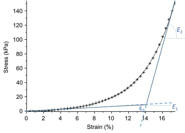
Figure 1.4: Experimental data (cross symbols) obtained on a right forearm solicited along  $0^\circ$ -axis; corresponding exponential model fit (solid line) from equation (1.3) and geometrical description of physical parameters. Obtained values:  $A = 1.3$  kPa,  $B = 27.4$ ,  $E_1 = 62.7$  kPa,  $E_2 = 4250$  kPa,  $\varepsilon_T = 13.9\%$ , and the quantified goodness-of-fit  $R^2 = 99.95\%$  [19].
