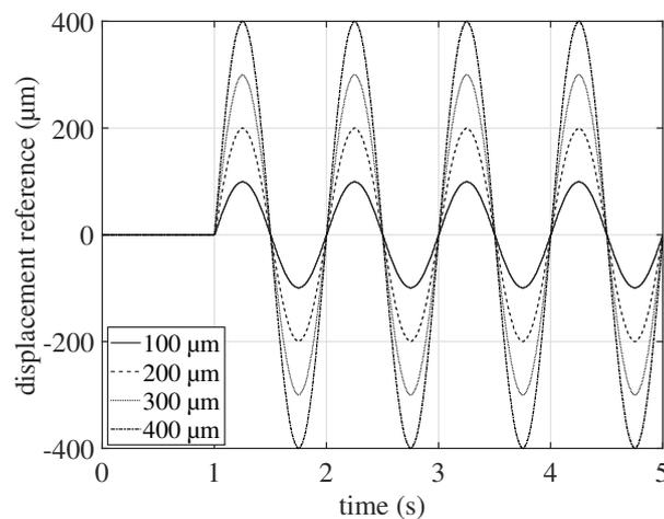
Figure 4.2: Cyclic loading pattern with four displacement amplitudes.
