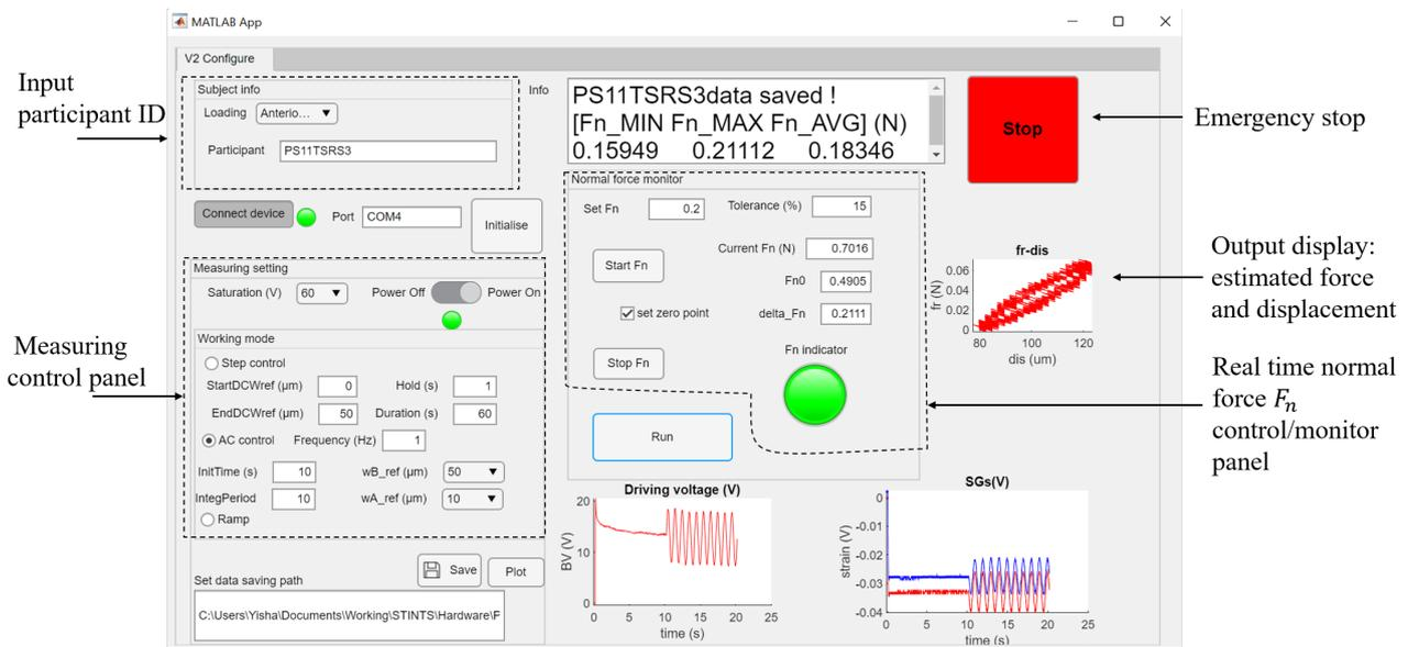
Figure 4.16: Graphical user interface designed for the MIP.
