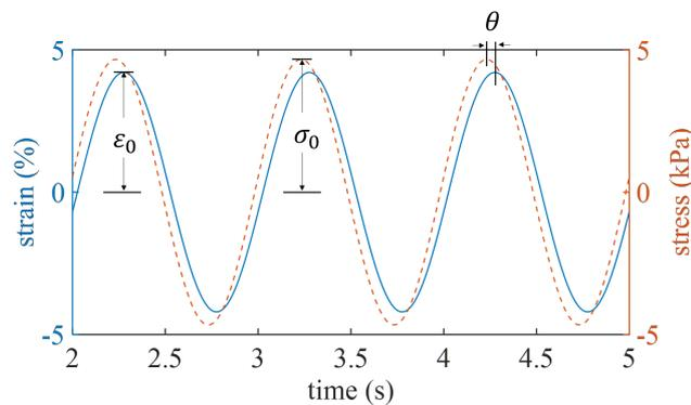
Figure 4.4: Strain and stress of viscoelastic materials.
