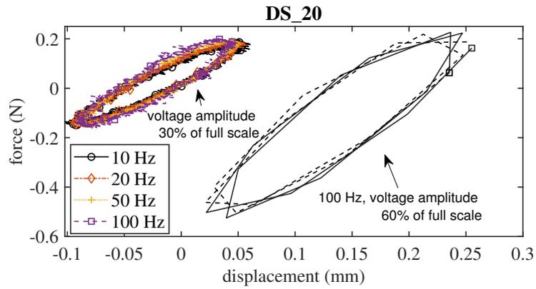
Figure 2.30: Phantom DS\_20 retested with a lower voltage amplitude 22 V, about 30% of full scale. Results obtained at 100 Hz under voltage amplitude about 60% of full scale are plotted as a comparison.
