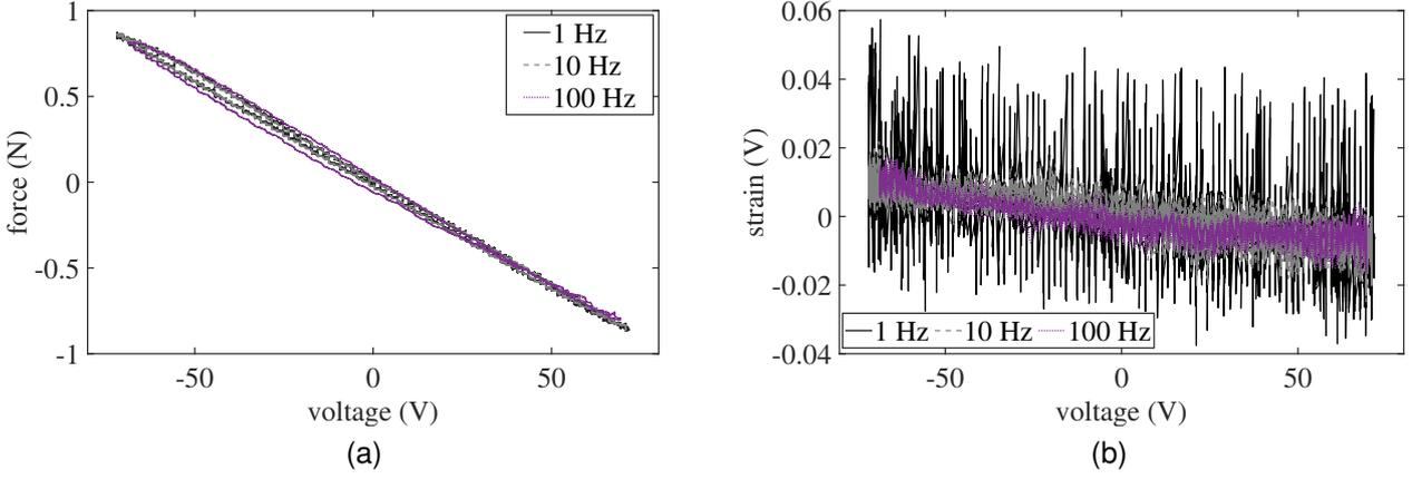
Figure 2.21: Blocking force (a) and strain (b) when the piezo bender is subject to full-scale sinusoidal voltage with its tip blocked.
