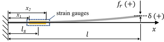
Figure 2.6: Geometry of the clamped cantilever bender with strain gauges glued on the top and bottom surfaces.  $x_1$  and  $x_2$  denote the starting and ending positions of the strain gauges.  $l_s$  indicates the center position of the gauges.
