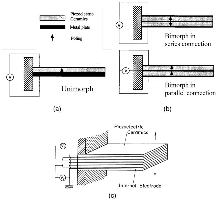
Figure 1.10: (a) Structure of a unimorph bender. (b) Structure of a bimorph bender [42]. (c) Structure of multilayer bimorph actuator [43].
