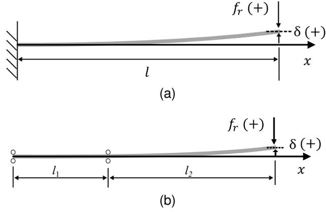
Figure 2.2: Mechanical structures. (a) Clamped cantilever piezoelectric bender. (b) Dual-pinned piezoelectric bender.  $l$  denotes the active length of the piezoelectric bender.  $l_1$  is the distance between the two groups of pins along  $x$  axis and  $l_1 + l_2 = l$ .
