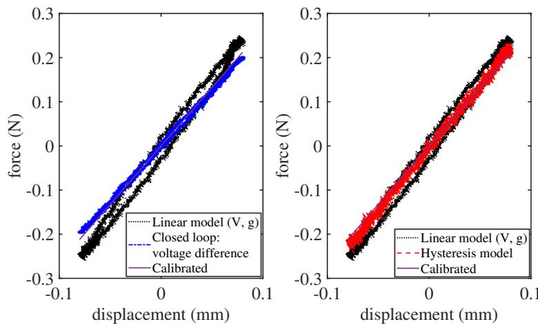
Figure 3.17: Estimated force as a function of estimated displacement with different force sensing approaches. Force estimated from the linear model ( $V, g$ ) referring to (2.15). Force estimation under closed-loop displacement control referring to (3.13). Force estimation with hysteresis model referring to (3.10). The calibrated force–displacement curve is reproduced from the calibration results of the spring load.
