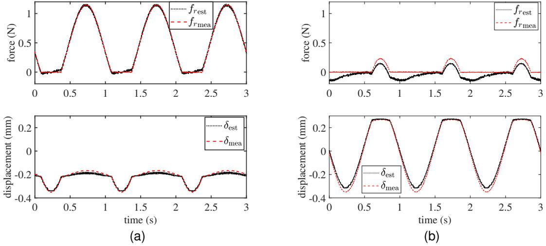
Figure 2.24: Sensing model validation under voltage and force excitation. (a) Hard stop around  $-0.21$  mm. (b) Hard stop around  $0.25$  mm. The black dot curves present the estimated force and displacement ( $f_{r\_est}$ ,  $\delta_{est}$ ) and the red dash curves are the measured results ( $f_{r\_mea}$ ,  $\delta_{mea}$ ).
