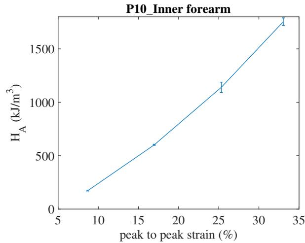
Figure 4.7: Strain-energy density dissipation as a function of peak-to-peak strain (mean  $\pm$  standard deviation (SD) of the 3 cycles). Data from one participant.
