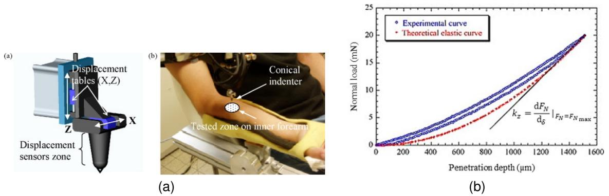
Figure 1.5: Indentation setup (a) and obtained curve (b) [20].
