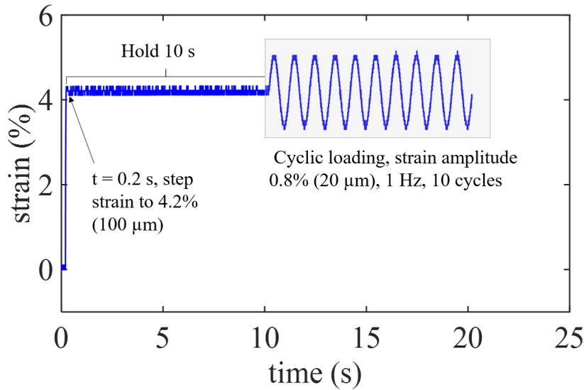
Figure 4.15: Loading pattern of the skin for dynamic mechanical analysis. The skin was stretched to 4.2% at  $t = 0.2$ s, then the strain was held for 10s, followed by a sinusoidal cyclic load at 1 Hz, with a strain amplitude of 0.8%.
