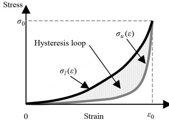
Figure 4.3: The typical uniaxial stress–strain relationships of soft tissue in the loading and unloading processes during a certain time period.  $\sigma_l(\varepsilon)$  and  $\sigma_u(\varepsilon)$  denote the stress curves during loading (strain increased) and unloading (strain decreased) [85].
