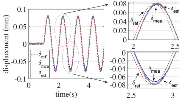
Figure 3.16: Evaluation on displacement sensing and control. The reference displacement is a sine wave with a frequency of 1 Hz, amplitude 0.08 mm. The spring is loaded at the bender tips.  $\delta_{ref}$ ,  $\delta_{mea}$ , and  $\delta_{est}$  represent reference displacement, measured displacement, and estimated displacement.
