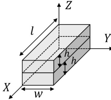
Figure 2.3: Schematic of bimorph piezoelectric bender.
