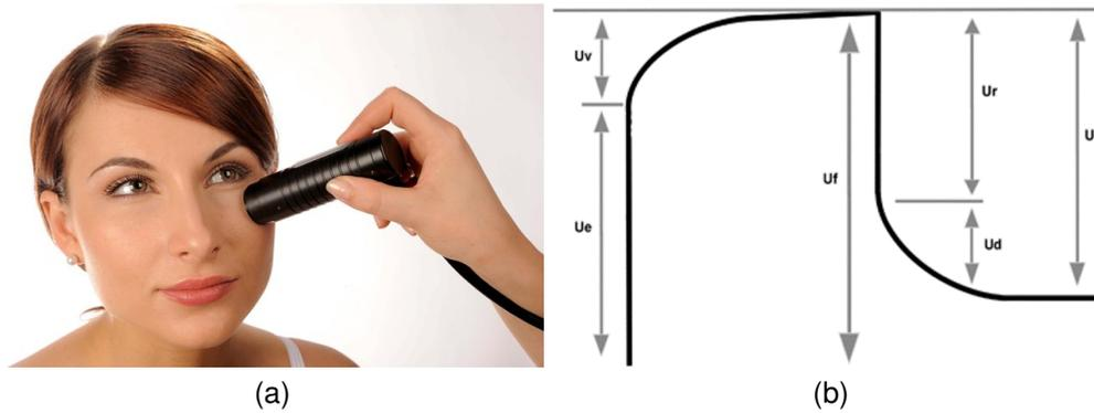
Figure 1.6: Suction tests. (a) Cutometer<sup>®</sup> Dual MPA 580. (b) skin deformation-time curve obtained with suction tests, parameters presented in the figure are skin distensibility ( $U_f$ ), immediate distensibility ( $U_e$ ), delayed distensibility ( $U_v$ ), maximum recovery ( $U_a$ ), immediate recovery ( $U_r$ ), delayed recovery ( $U_d$ ) [21].
