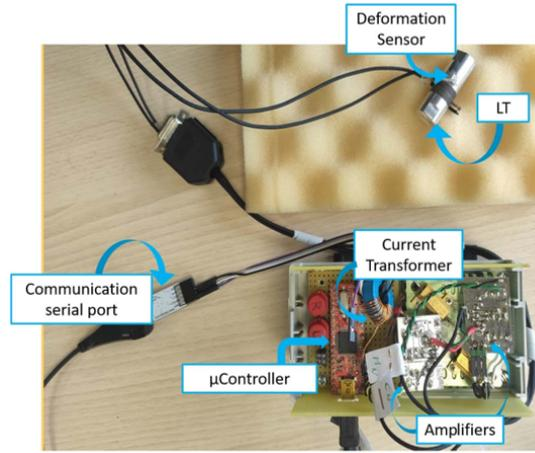
Figure 1.15: Langevin transducer used for mechanical impedance measurements [49].
