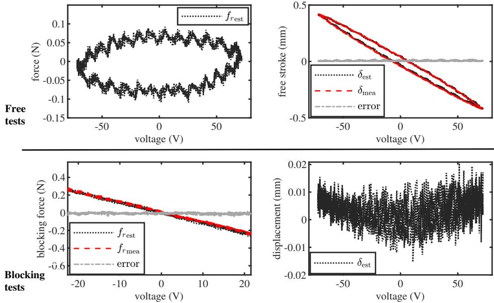
Figure 2.22: Sensing performance under extreme cases (tip free and tip blocked). Estimated force and displacement ( $f_{r_{est}}$ ,  $\delta_{est}$ ) are compared to measured results ( $f_{r_{mea}}$ ,  $\delta_{mea}$ ). The piezoelectric benders were subject to a full-scale voltage at 1 Hz. Top row: free tests, under voltage excitation only. Bottom row: blocking tests, under voltage and force excitation.
