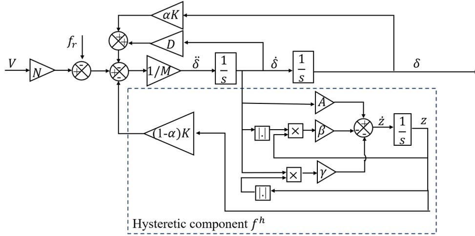
Figure 3.5: Block diagram of the hysteresis model.
