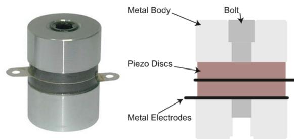
Figure 1.14: Bolt-clamped Langevin transducer with two piezoelectric layers [48].
