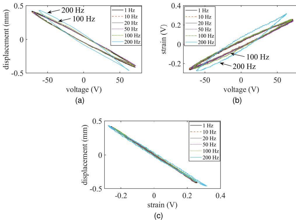
Figure 2.19: System responses to high voltage excitation at various frequencies (a full-scale voltage command was sent to the DSP). Tip displacement  $\delta$  (a) and bending strain  $g$  (b) in response to voltage excitation  $V$ . The relationship between displacement and bending strain is presented in (c).
