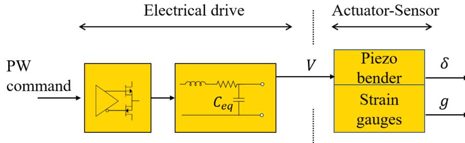
Figure 3.1: Block representation of the subsystems. The piezo bender (represented by the equivalent capacitor  $C_{eq}$ ) is a part of the low pass filter.
