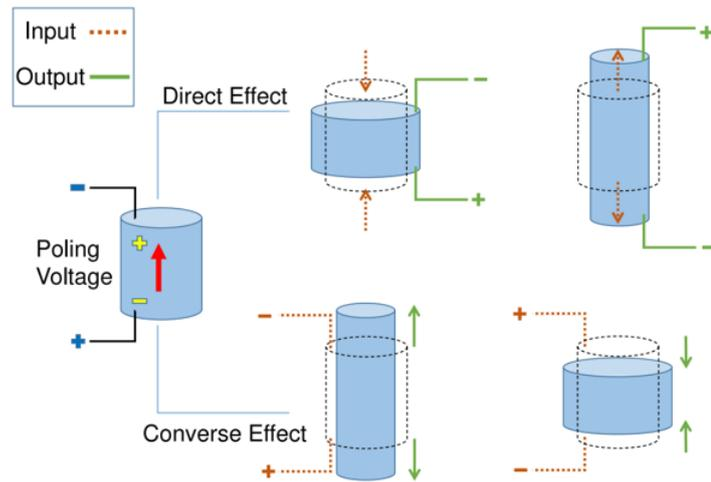
Figure 1.9: Direct and converse effects in piezoelectric ceramic [38].
