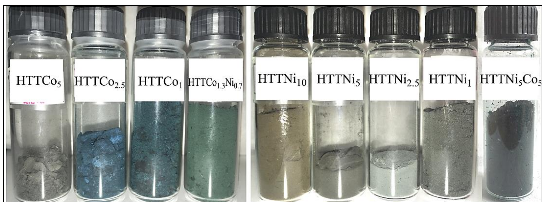
Figure 4.27. As-obtained TM Chloride modified-PSZ polymers according to the Si:Metal ratio.
