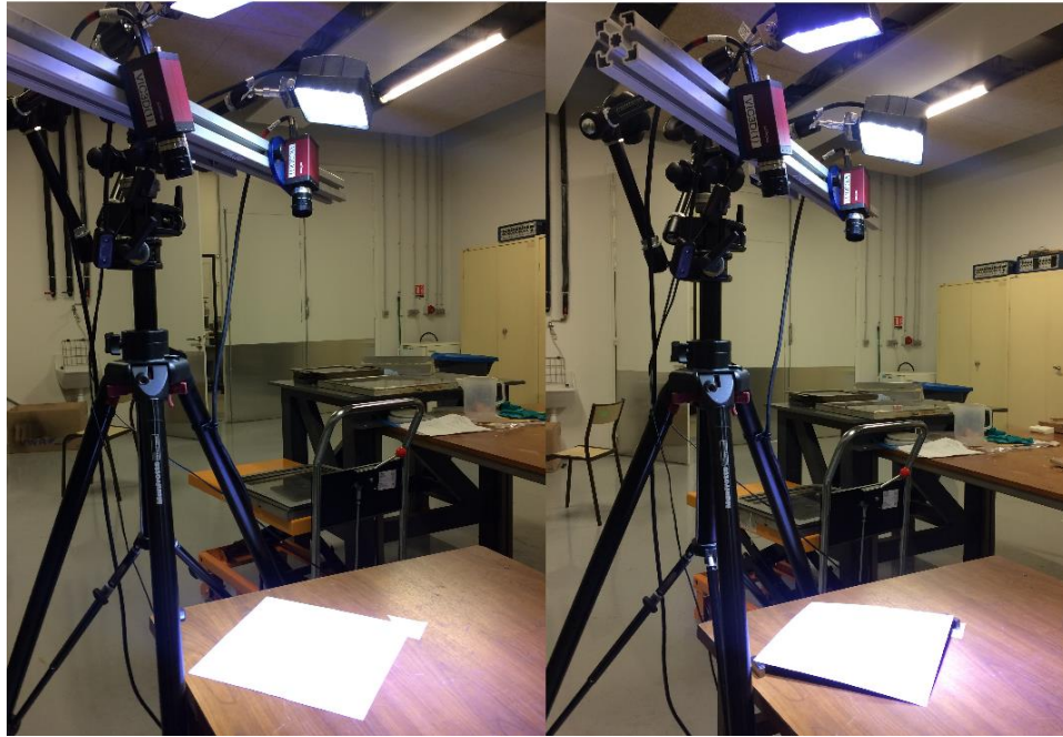
Figure 3.18 Measurement setup for DIC.
