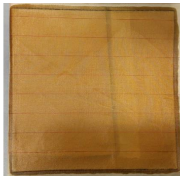
Figure 3.44 Permeability of peel-ply to liquid resin.
