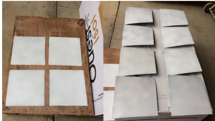
Figure 3.16 Spray white colour on the top surface of laminate.
