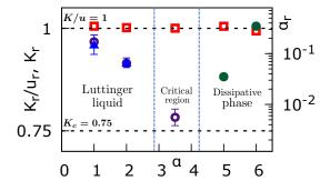
FIG. 5. Renormalized value of different parameters of the action for K=1, s=0.5.  $K_r/u_r$  (red square) remains constant and equal to 1 for all values of  $\alpha$ .  $K_r$  decreases from K=1 to  $K_c=0.75$  as  $\alpha$  increases and approaches  $\alpha_c$ .  $\alpha_r$  becomes relevant in the dissipative phase and increases as a function of  $\alpha$ . This behavior of the parameters helps us locate the critical region  $\alpha_c \in (3,4)$ .
