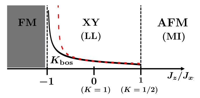
Figure 2.4: Phase diagram of 1D commensurate XXZ spin chain. The system can be solved exactly with Bethe Ansatz, and bosonization captures the XY phase (described by LL theory) and the AFM system (described by Mott Insulator theory). The LL parameter K calculated via bosonization  $K_{\text{bos}}$  (black solid line) matches well with the value obtained from Bethe Ansatz  $K_{\text{BA}}$  (red dashed line) in the region  $J_z \ll J_{xy}$  and diverges at the Ferromagnetic transition.
