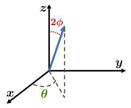
Figure 2.3: The physical interpretation of the fields  $\phi$  and  $\theta$  in context of the original microscopic system. The spin (blue arrow) can rotate in three dimensions.  $2\phi$  (red) is the angle it makes with the z-axis, and  $\theta$  (green) represents the angle between x-axis and the spin's projection on the x-y plane.
