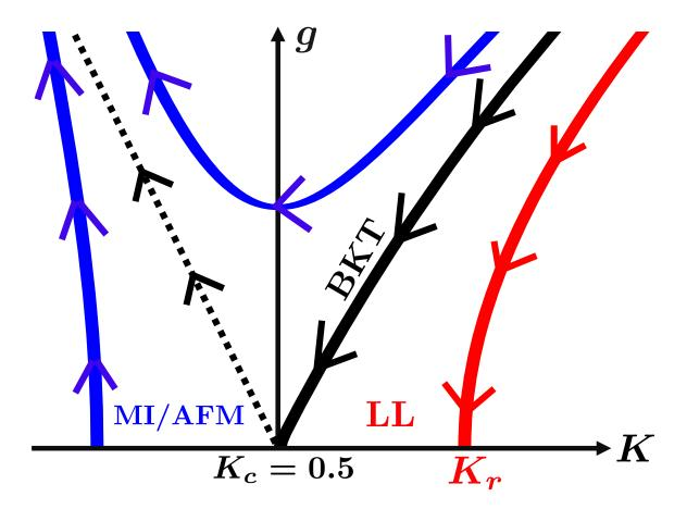
Figure 3.1: RG flow of Sine-Gordon model. The red line corresponds to the LL phase, where  $K_r$  is finite and  $g_r = 0$  (see text). The separatrix is given by the solid black line  $g_c = K - K_c$ . For  $g > g_c$  with  $K \ge K_c$  and for any value of  $\alpha$  with  $K < K_c$ , the cosine term becomes relevant as  $g_r = \infty$  and  $K_r = 0$ , indicating the presence of a new phase. The arrowheads denote the direction of the flow.
