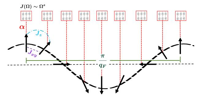
FIG. 1. Schematic diagram of a one-dimensional quantum XXZ spin chain coupled with local dissipative baths.  $J_{xy}$  denotes the hopping energy and  $J_z$  is the interaction between the two nearest neighbour spins. The baths are characterized by their spectral function  $J(\Omega) \sim \alpha \Omega^s$ . At zero temperature, the baths induce an SDW phase with periodicity  $\pi/q_F$ , where  $q_F$  is the Fermi-momentum related to the magnetization of the chain (see text).
