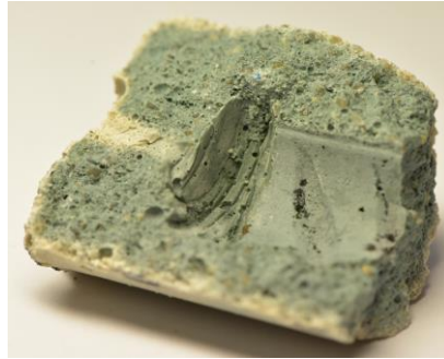
Figure 51: Mortar of a SSC anode after 90 days of galvanic coupling ( [\text{NaCl}] = 30 \text{ g/L} ).
