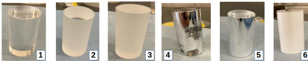
Figure 6.20 – Photos of different BGO configurations that we tested. (1) Polished BGO. (2) Half-polished BGO. (3) Not polished BGO. (4) Al-coated BGO. (5) BGO wrapped in the ESR film. (6) BGO wrapped in the PET film.
