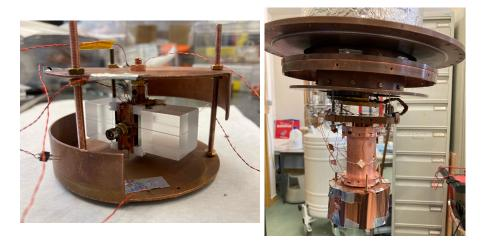
Figure 5.2 - left: The small prototype inside its copper structure. *right*: The cryostat configuration during the cryogenic measurement. The closed nylon assembly structure is at the bottom, attached to another detector unrelated to this Chapter.
