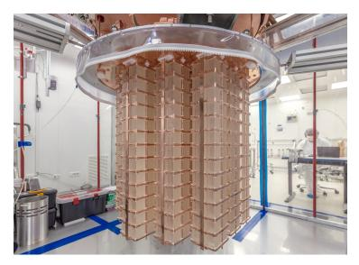
Figure 2.11 – Cuore towers inside the opened cryostat.
