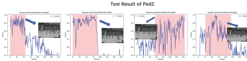
Figure 5.5: Test results on the dataset UCSD(ped2). The pink background is the area where the real anomaly occurs; The blue curve represents the change of the anomaly score with the time series. These Figure show that the model proposed in this contribution has high and stable detection capabilities
