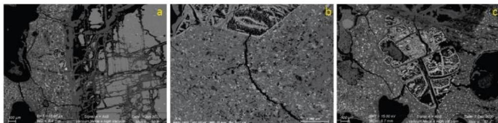
**Figure 13.** DJI-4-1 SEM pictures in AsB mode displaying (a) a centimeter-scale plagioclase partially altered to kaolinite/smectite with an olivine next to it in a smectite and oxide matrix; (b) close-up view of the iron-rich smectite matrix near a Mn-oxide; (c) fractured Mn-oxide with white Fe enrichment.
