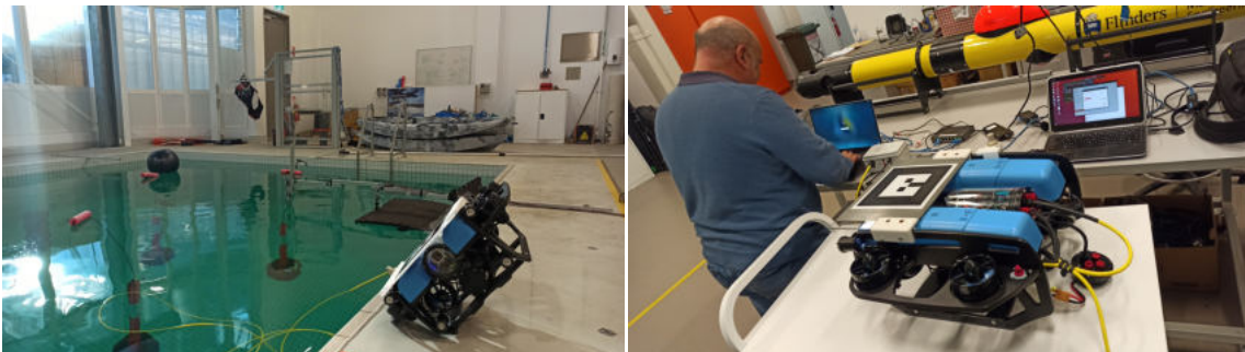
(a) The BlueRov2 platform resting on the side of the water tank at FLINDERS University. (b) A Kalman filter fuses IMU and camera data to estimate the marker's position.
