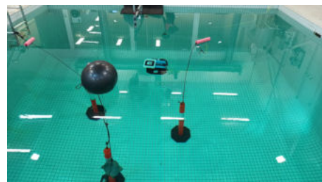
(d) The setpoints are chosen so as to always be visible by the camera, resulting in a working space of about 5m long, 3m wide, and 3m deep.
