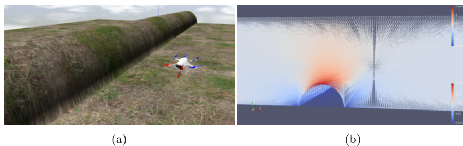
Fig. 3: Visualization of the simulated environment in Gazebo (a) and the wind field in Paraview (b). The complete details of the wind field we used can be find on the RotorS-based extended wind plugin page.
