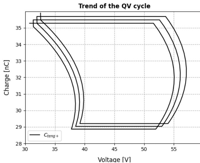
**Figure 34:** QV cycle simulation of  $C_{t+}$ .
