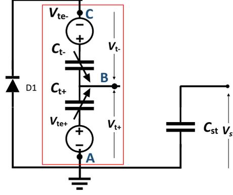
**Figure 26:** Topology of double Bennet formed for the instance from  $E^i$  to  $F^i$ . Conduction of diode  $D_1$  creates a parallel connection of TENG's capacitors.
