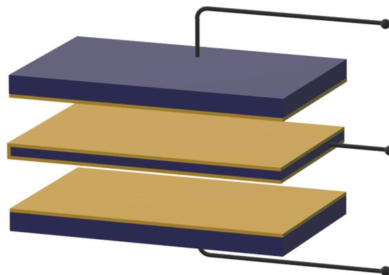
**Figure 15:** *A mechanical model of double capacitive eKEH.*
