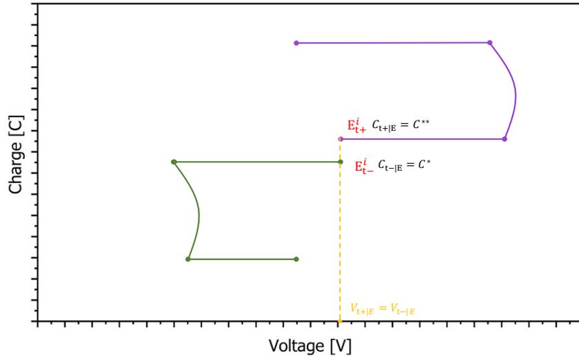
**Figure 25:** The evolution of the QV cycle for the instance from  $D^i$  to  $E^i$  defined by the equal voltages of transducer's capacitors at the final point of the instance.
