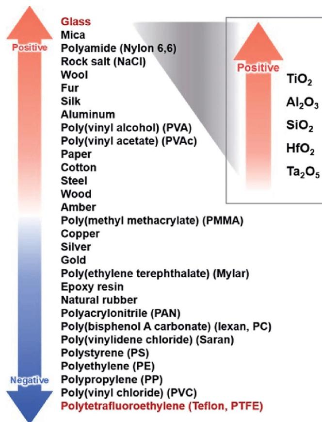
**Figure 9:** A triboelectric scale defining positive and negative charge trapping capabilities of range of materials.[28]
