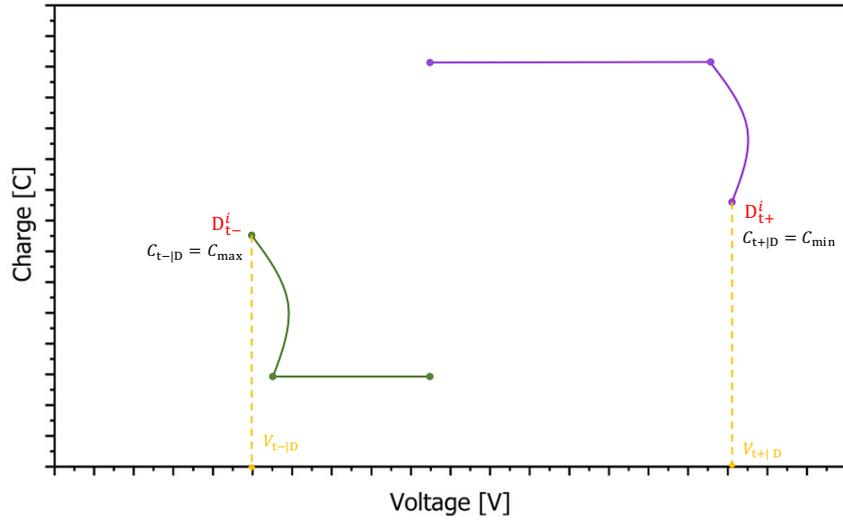
**Figure 23:** The evolution of the QV cycle for the instance from  $B^i$  to  $D^i$ . The Series configuration of the capacitors causes the charges to flow.
