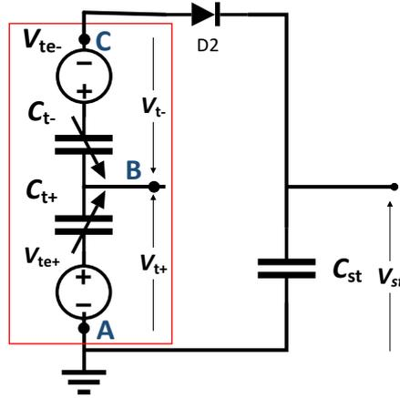
**Figure 22:** Topology of double Bennet formed for the instance from  $B^i$  to  $D^i$ . The diode  $D_2$  conducts, resulting in two TENG's capacitors and a storage capacitor being connected in series.
