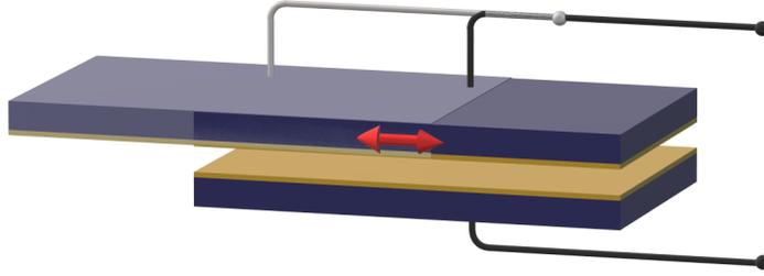
**Figure 6:** A model of an in-plane overlapping eKEH demonstrating the sliding movement of the mobile electrode.
