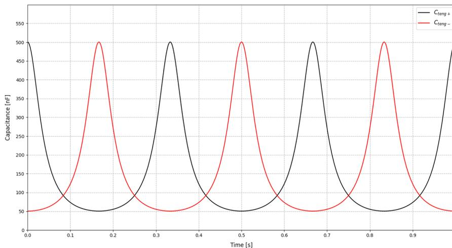
**Figure 30:** Simulated capacitance shapes of  $C_{teng+}$  and  $C_{teng-}$ .
