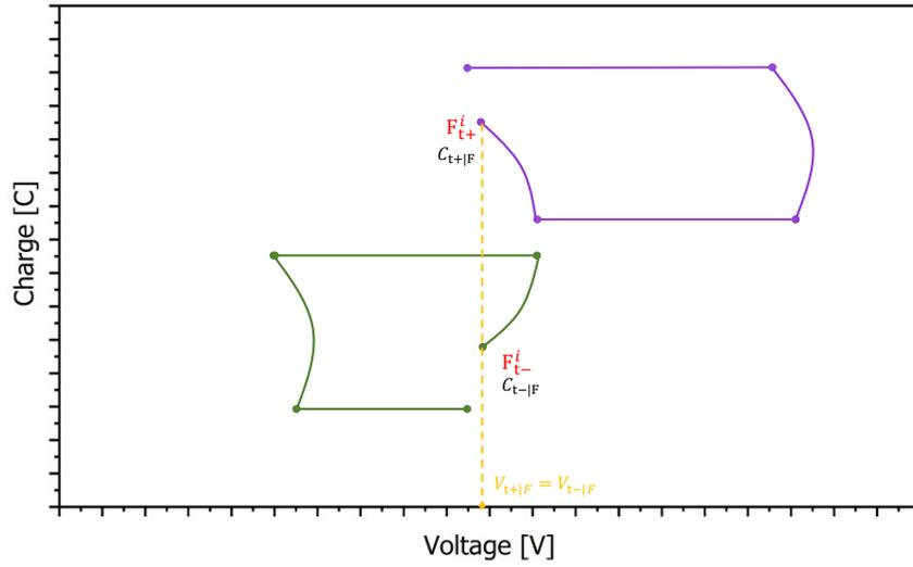
**Figure 27:** The evolution of the QV cycle for the instance from  $E^i$  to  $F^i$ . The parallel connection of TENG's capacitors starts the charge accumulation process in  $C_{t+}$ .
