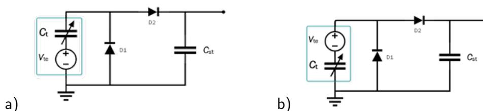
**Figure 42:** Half-wave circuit with a) TENG capacitor's plate with triboelectric layer is grounded (circuit labeled as half-wave 1). and b) Another plate of the capacitor is grounded and plate with triboelectric layer is connected towards the rest of the circuit (half-wave 2).
