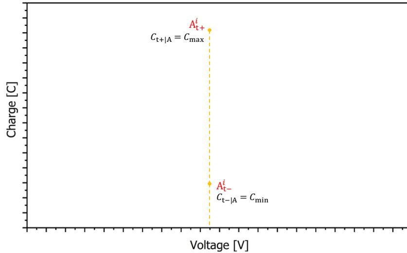
**Figure 19:** Initialization of the QV cycle with point  $A^i$ , at which  $C_{t+} = C_{max}$  and  $C_{t-} = C_{min}$  set at the same potential.
