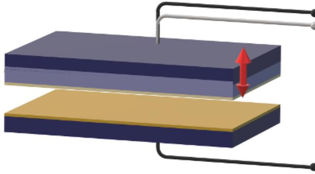
Figure 8: A model of gap-closing eKEH demonstrating the misplacement of mobile electrode.
