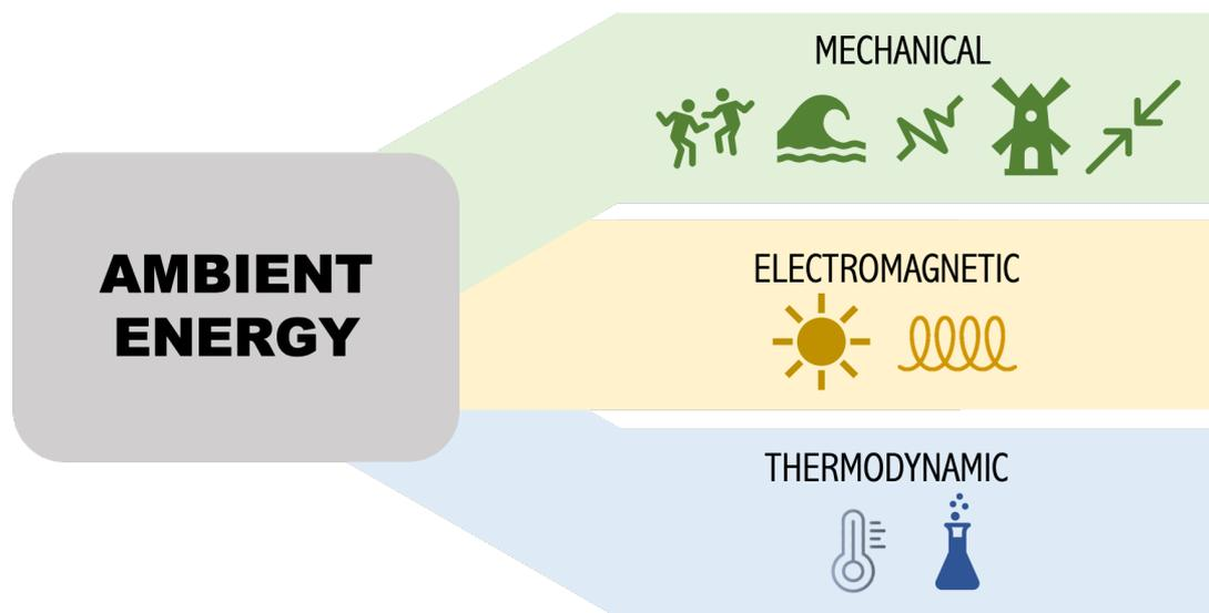
**Figure 2:** The three forms of ambient energy used in energy harvesting: mechanical (human movement, bodies of water, vibrations, wind and pressure), electromagnetic (solar energy and induction) and thermodynamic (temperature gradient and chemical reactions).
