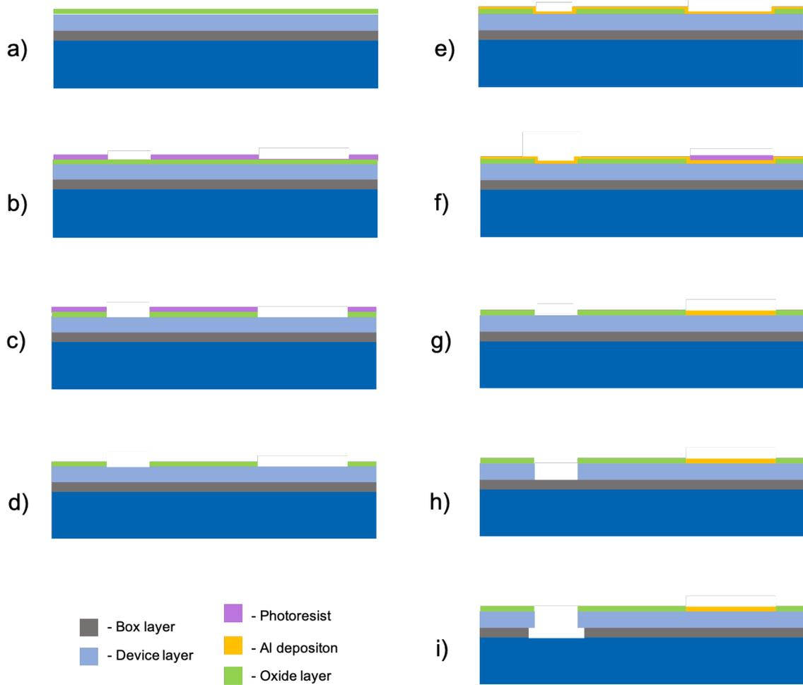
**Figure 56:** *The fabrication process. a) SOI wafer with oxidation. b) Photoresist added as a sacrificial layer and photolithography. (general trenches) c)Oxide etching. d) Cleaning. e) Al deposition. f) 2nd photoresist layer and photolithography. (pad area) g)Al etching and wafer cleaning. h) DRIE of the full thickness of the device layer. (anisotropic) i)Oxide etching using vapor HF. (isotropic)*
