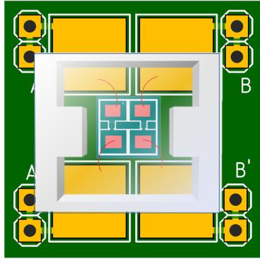
**Figure 57:** Packaging used for fabricated switches for their integration on a more robust PCB. The package is composed of an adapter on which the sample is mounted and wire bonded, which is then covered by a frame and protection glass.
