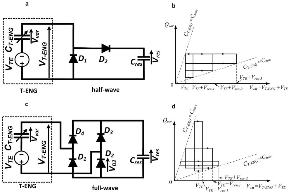
**Figure 12:** Half-wave and full-wave rectifying circuits and their QV cycles. a) The schematic representation of the HW. and b) The QV cycle that yields from the HW operating. c) The schematic representation of established connection between TENG and diodes forming a FW. d) The QV cycle generated by operation of FW. The two QV diagrams are plotted with assumption of  $C_{res} \gg C_{max}$ . [37]
