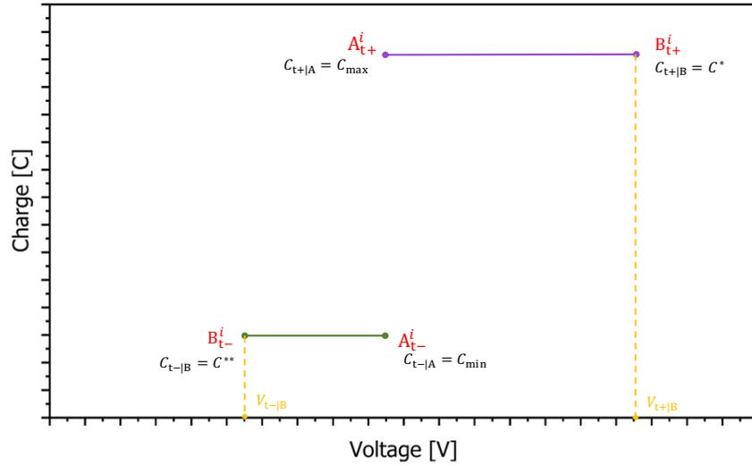
**Figure 21:** The evolution of the QV cycle for the time interval  $A^i$  to  $B^i$ . Constant charge and variation in voltages are present for both  $C_{t+}$  and  $C_{t-}$ .
