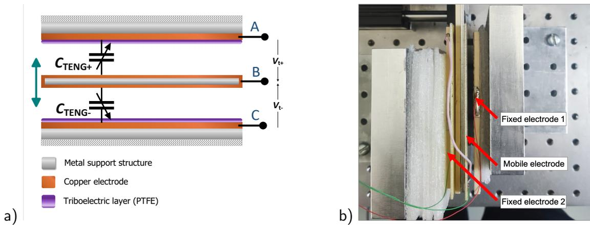
**Figure 36:** a) A schematic representation of plate distribution and materials on them constructing a double TENG. b) A photograph of constructed TENG with one fixed plate on the right, a mobile plate in the middle and another fixed plate on the left side
