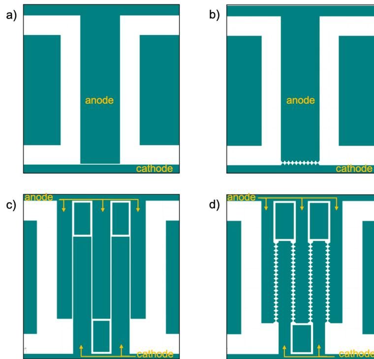
**Figure 55:** *Designs of fabricated switches. a) A single beam with a flat surface facing the cathode. b) A single beam with 10 triangle-like extrusions at its end facing the same extrusions on the cathode. c) Comb-like structure of five fingers with flat surfaces on both anode and cathode. d) Comb-like structure with 100 extrusions distributed over 3 anode and 2 cathode fingers.*
