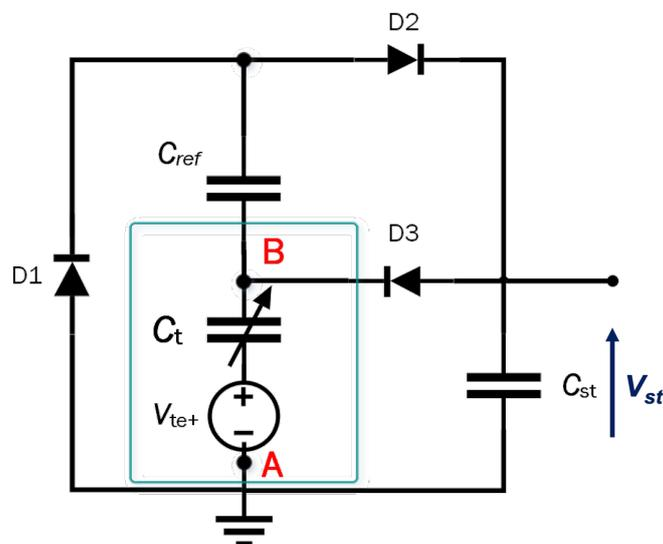
Figure 44: The schematic of classic Bennet's doubler circuit.
