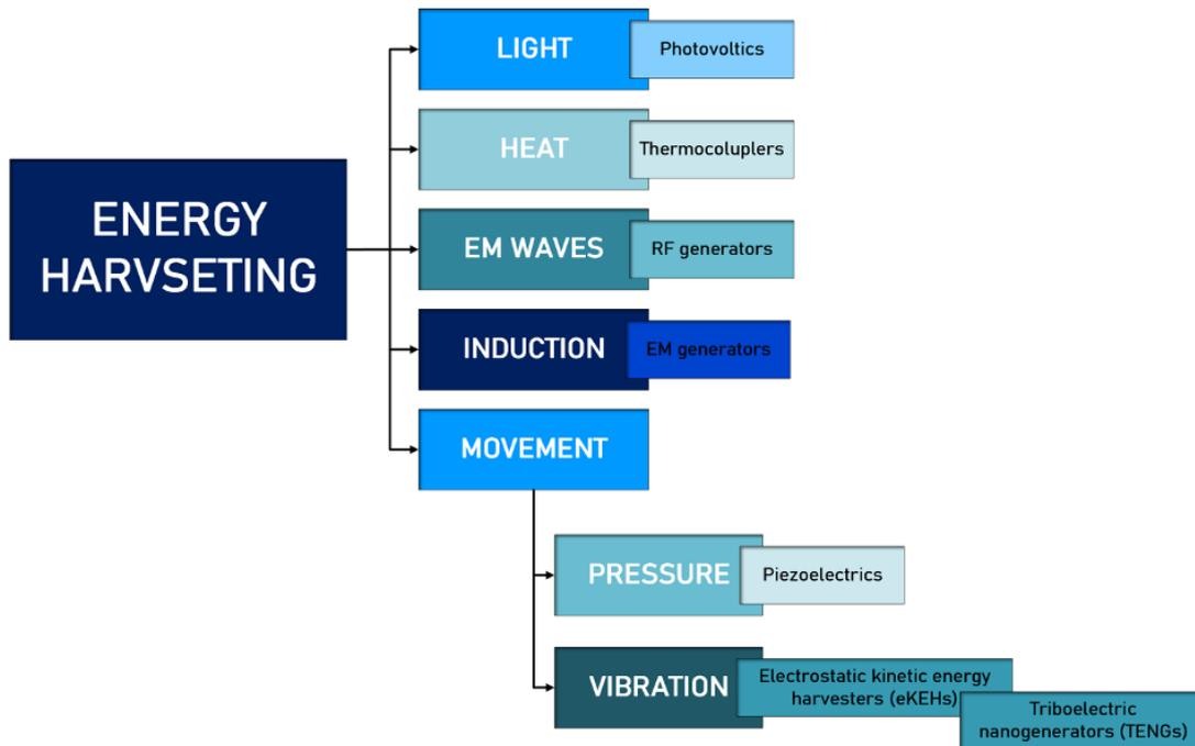
**Figure 3:** A map of energy harvesting based on energy source. It includes: light, heat, electromagnetic waves, induction and movement. Movement can come in a form of pressure (piezoelectric) and vibrations (eKEHs).
