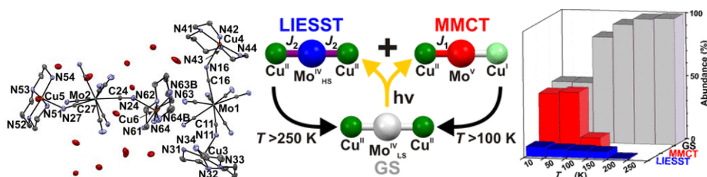
Figure I. 31 (Left) The asymmetric unit of [\text{Cu}^{\text{II}}(\text{enpnen})]_2[\text{Mo}^{\text{IV}}(\text{CN})_8]\cdot 6.75\text{H}_2\text{O} . (Middle) Schematic of the ground-state model, the MMCT excited-state model, and the LIESST excited-state model. (Right) Abundances of the ground state (GS), light-induced MMCT and LIESST states for the irradiation at 10, 50, 100, 150, and 200 K. Reproduced from Ref. [125] with permission from the American Chemical Society 2018.
