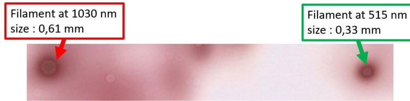
Figure 4.4.1: Example of a photosensitive paper measurement showing the impact of filaments of two different sizes attributed to the two laser wavelengths at 1030 nm and 515 nm.
