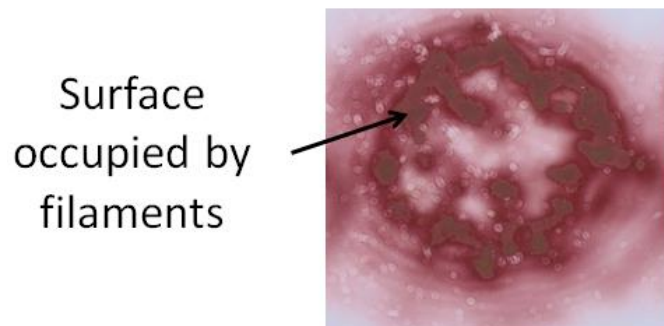
Figure 5.2.1: Example of a photosensitive paper measurement made using the telescope focusing beam.
