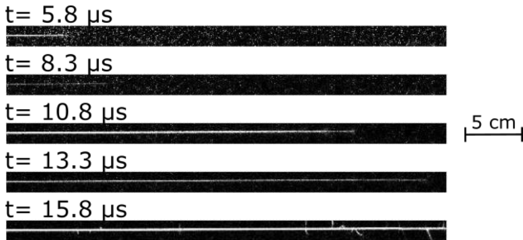
Figure 2.3.2: Streamer-leader propagation of a discharge produced by our 300 kV Tesla generator, recorded with a high-speed camera at a speed of 400 000 frames/s. The stepping of the propagation is clearly visible (note that this stepping is also partially due to the oscillation of the background field), and the mean speed is measured to be in the range of 10^4 - 10^5 \text{ m.s}^{-1} , characteristic of a streamer-leader discharge.
