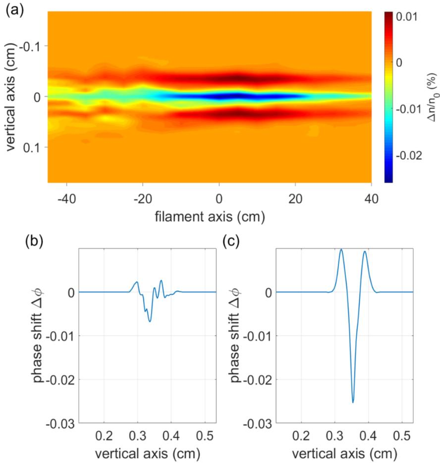
**Figure 2.2.1:** (a) Phase shift induced by the under-dense channel created by the filamentation of the 150 mJ, 780 fs pump laser, measured 1  $\mu$ s after the laser pulse. Profiles of the phase shift measured at the position -40 cm (b) and 0 cm (c) along the filament axis. The laser propagates from the negative to the positive values of the filament axis, and the lens focal plan is at  $z = 10$  cm.
