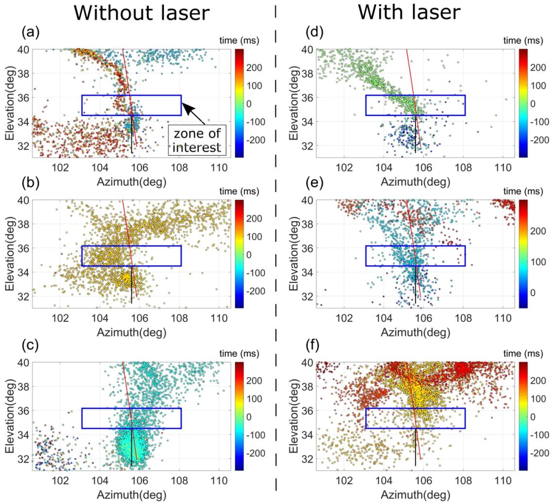
**Figure 4.3.1:** Plot of temporal and spatial distributions of the VHF sources for the events without laser (a) LLR N2, (b) LLR P5, (c) LLR N7 and the events with laser (d) LLR P1, (e) LLR P3, (f) LLR P4 (see table 1 and 2 for the date of the events). The Sântis tower is represented on each plot as a black line, the laser path is represented as a red line. The blue rectangles correspond to the zones of interest where guiding effect is observed (height = 60 m, width = 185 m).
