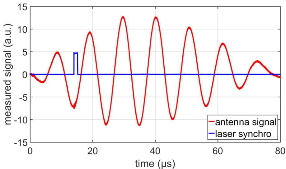
**Figure 2.1.2:** Plot of the oscilloscope measurement showing (in blue) the signal of synchronization of the laser pulse, and the signal of the antenna measuring the voltage at the high voltage electrode of the Tesla generator (in red).
