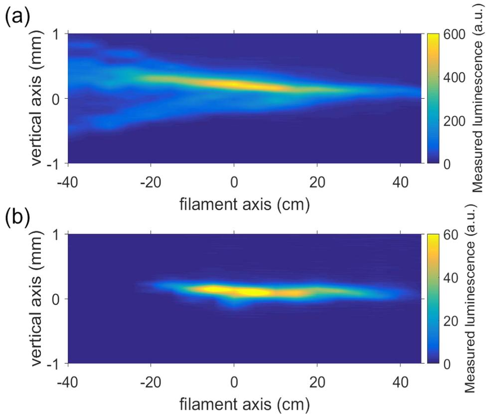
**Figure 2.1.2:** Picture of the luminescence of the plasma measured for an energy of (a) 150 mJ and (b) 20 mJ, for a pulse duration of 780 fs. The laser propagates from the negative to the positive values of the filament axis, and the lens focal plane is at  $z = 10$  cm.
