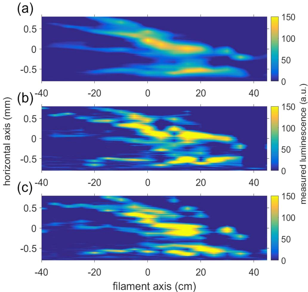
**Figure 2.4.1:** Picture of the luminescence from the plasma measured for an energy of 150 mJ, pulse duration 780 fs, taken from the top. (a) is averaged over 50 laser pulses, while (b) and (c) are from two different single shots.
