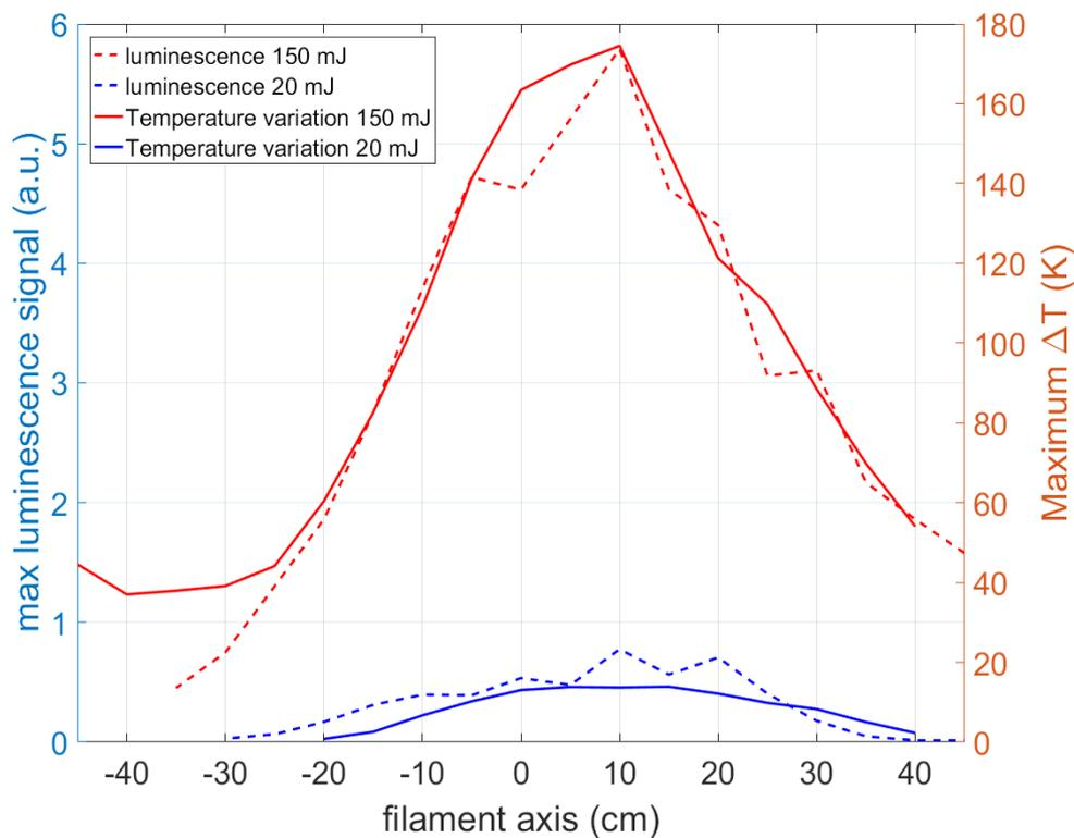
**Figure 2.2.5:** Comparison between the evolution along the filament axis of the maximum of the temperature variation and the luminescence, induced by the filaments created for a pump energy of 150 mJ (in red) and 20 mJ (in blue). The laser propagates from the negative to the positive values of the filament axis, and the focal plane of the 7 m lens is at  $z = 10$  cm.
