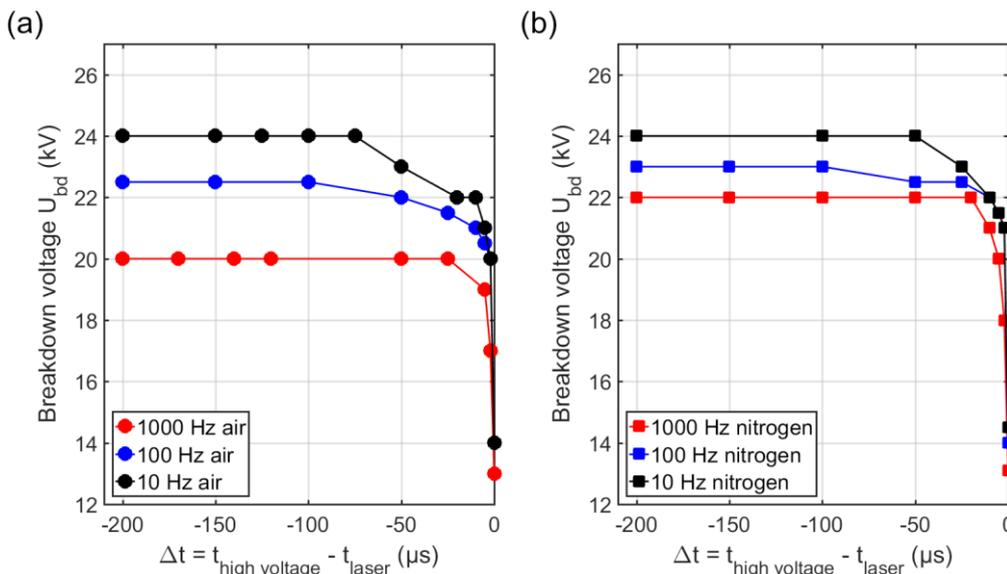
**Figure 3.7.2:** Breakdown voltage measured with 0.8 mJ, 35 fs laser pulses focused at  $f/100$ , as a function of the delay between the high voltage pulse and the last laser pulse, at different laser repetition rates. (a) Measurements made in ambient air. (b) Same measurements made in pure nitrogen. In both cases, the natural breakdown without laser is 29 kV.
