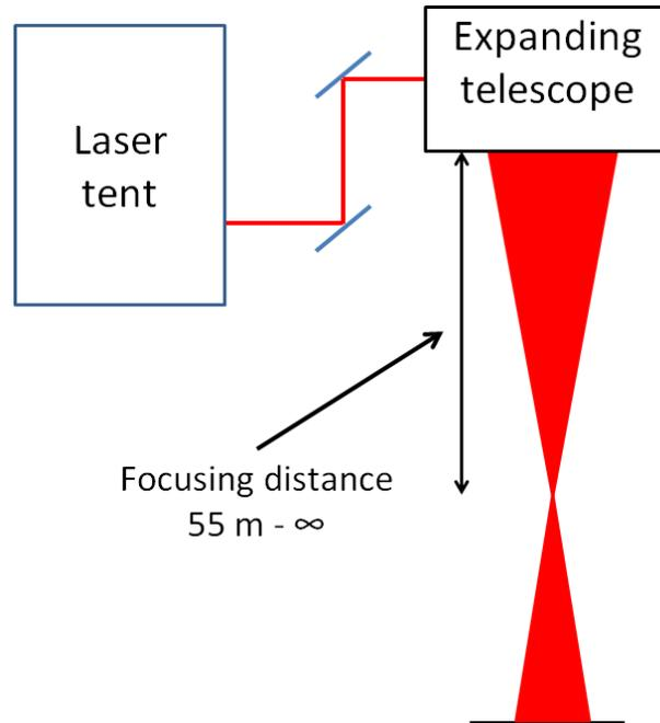
**Figure 5.1.1:** Experimental setup using the focusing telescope.
