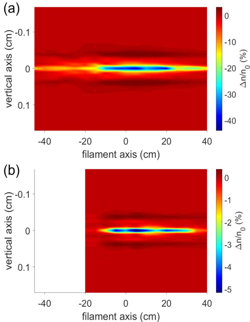
**Figure 2.2.2:** Neutral density variation induced by the filamentation of a 780 fs laser pulse with an energy of 150 mJ (a) and 20 mJ (b), measured 1  $\mu$ s after the laser pulse. The laser propagates from the negative to the positive values of the filament axis, and the focal plane of the 7 m lens is at  $z = 10$  cm.
