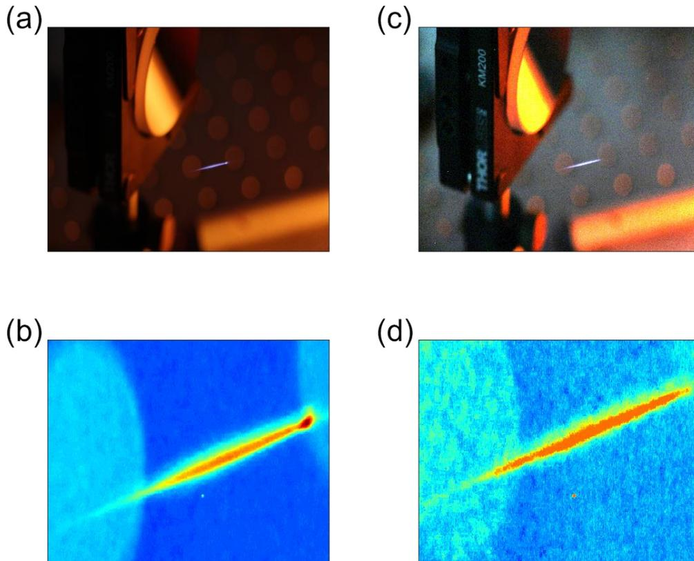
**Figure 3.9.1:** Real colour picture of the light emitted by the filament taken by (a) integrating during 1 s with the laser set at 100 Hz and (c) integrating during 10 s with the laser set at 10 Hz. (b) and (d) are the corresponding picture of the filament region only of (a) and (b) by converting them in false color. In all the pictures, the laser propagates from right to left.
