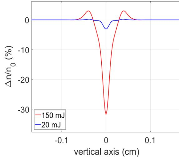
**Figure 2.2.3:** Profile of the density variation induced by the filamentation of the 780 fs pump laser set at 150 mJ (in red) and 20 mJ (in blue), measured at the 0 cm position of the filament axis, 1  $\mu$ s after the last laser pulse.
