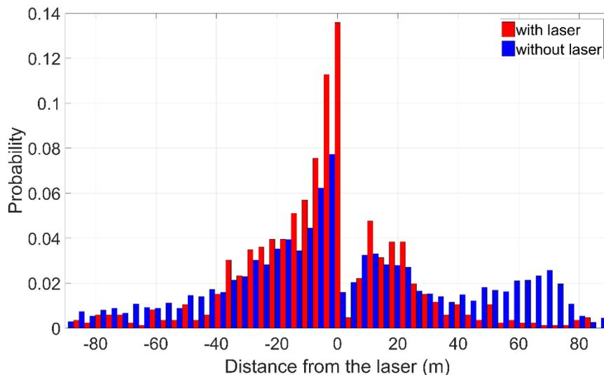
**Figure 4.3.3:** Distributions of the nearest distance from the VHF sources to the laser path for flashes with laser, and flashes without laser. The value of the mean absolute distance is presented for both with and without laser.
