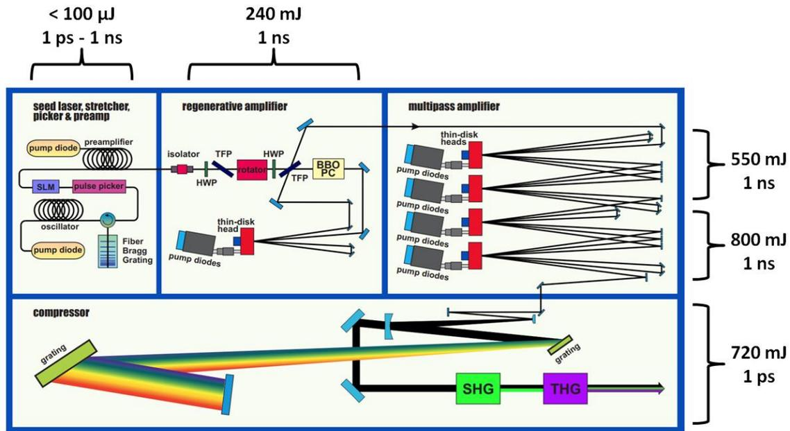
**Figure 1.1:** Layout of the LLR laser system
