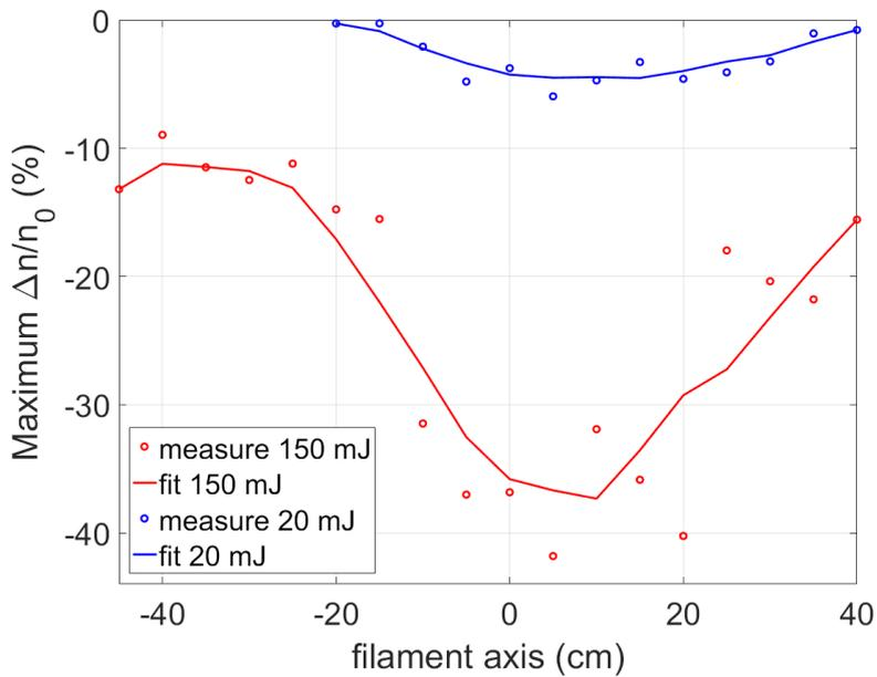
**Figure 2.2.4:** Evolution along the filament axis of the maximum of the density variation induced by the filaments created with a pump energy of 150 mJ (in red) and 20 mJ (in blue). The laser propagates from the negative to the positive values of the filament axis, and the focal plan of the 7 m lens is at  $z = 10$  cm.
