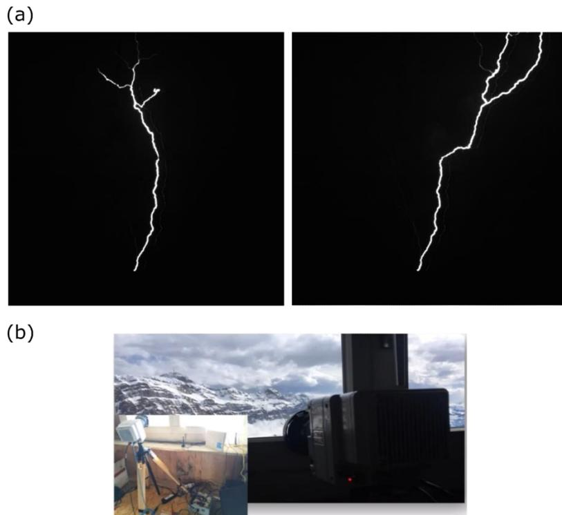
**Figure 2.1.2:** (a) Two frames recorded by the camera of an upward lightning strike on the 30<sup>th</sup> July 2021 at 15:38:10 UTC. (b) Picture of the camera in its room at the Kronberg Luftseilbahn.
