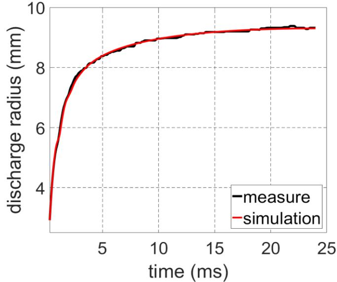
**Figure 2.4.1:** Comparison between the measured and simulated temporal evolution of the radius of the discharge for a capacitance value in the secondary circuit of  $C = 720$  nF.
