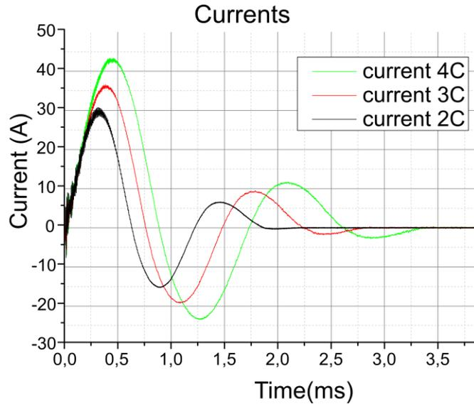
**Figure 2.2.1:** Current in the high voltage discharge measured for the three values of capacitance  $C = 350$  nF (labelled as 2C, in black),  $C = 540$  nF (labelled as 3C, in red) and  $C = 720$  nF (labelled as 4C, in green).
