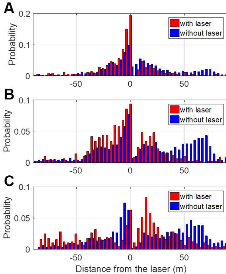
**Figure 4.3.2:** Cumulative histograms of VHF sources distance to the laser beam as per height slice of 30 m for all the events with and without laser. (A), (B) and (C) corresponding respectively to the height slices 0-30 m, 30-60 m and 60-90 m.
