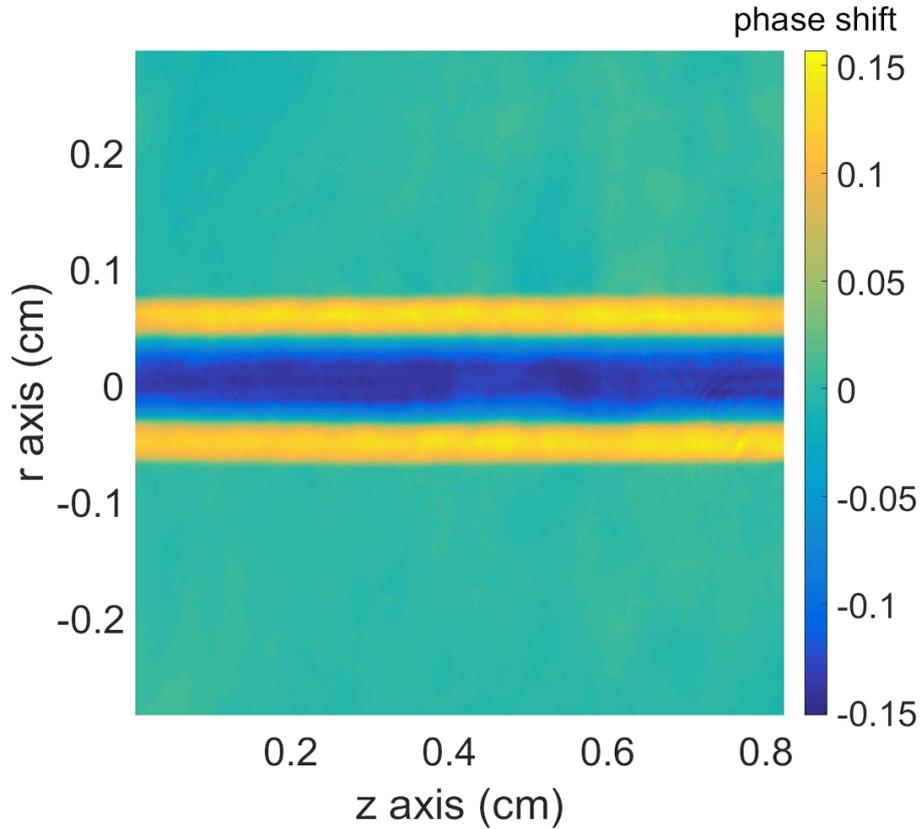
**Figure 1.2.2:** Example of a typically measured 2D phase map (unit:  $2\pi$  rad) induced by a  $fs$  filament in air (from a 14 mJ, 50 fs, 800 nm laser pulse focused at  $NA=0.0078$ ),  $r$  axis and  $z$  axis being respectively the vertical axis and the longitudinal axis (optical axis).
