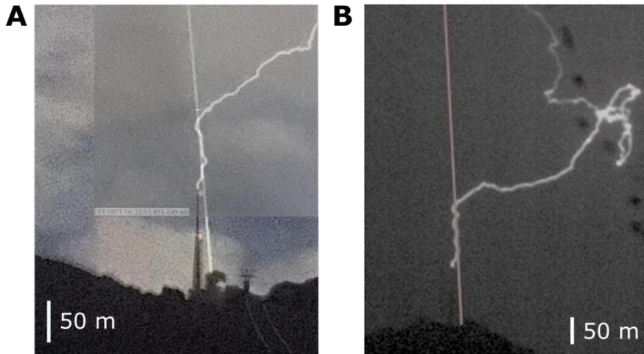
**Figure 4.2.1:** Snapshots of the lightning event of July 24 (L2) recorded in the presence of the laser by the two high-speed cameras located at Schwaegalp (A) and Kronberg (B). The trajectory of the laser path taken subsequently in cloudless sky through second harmonic generation is also overlaid.
