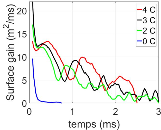
**Figure 2.3.6:** Measured surface gain of the cross section of the discharge  $2\pi r \frac{\partial r}{\partial t}$  for capacitance values in the secondary circuit of  $C = 720$  nF (labelled as 4C, in red),  $C = 540$  nF (labelled as 3C, in black),  $C = 350$  nF (labelled as 2C, in green), and for no capacitance (labelled as 0C, in blue).
