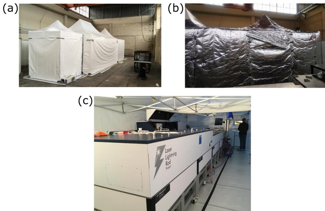
**Figure 3.1:** picture of (a) the tent, (b) the tent with its additional layer of insulative foil and (c) the laser inside the tent.
