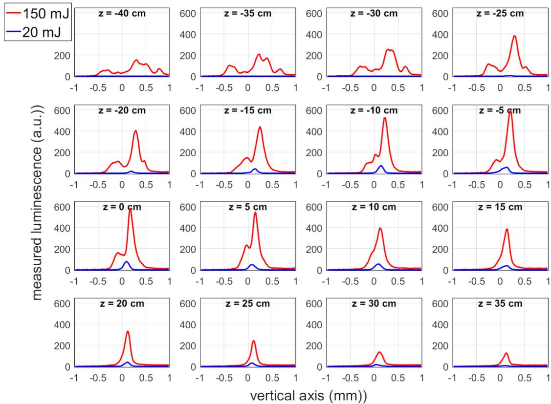
**Figure 2.1.3:** Plot of the luminescence profile along the vertical axis measured at different positions along the filament axis  $z$ , for an energy of 150 mJ (in red) and an energy of 20 mJ (in blue). The pulse duration is 780 fs.
