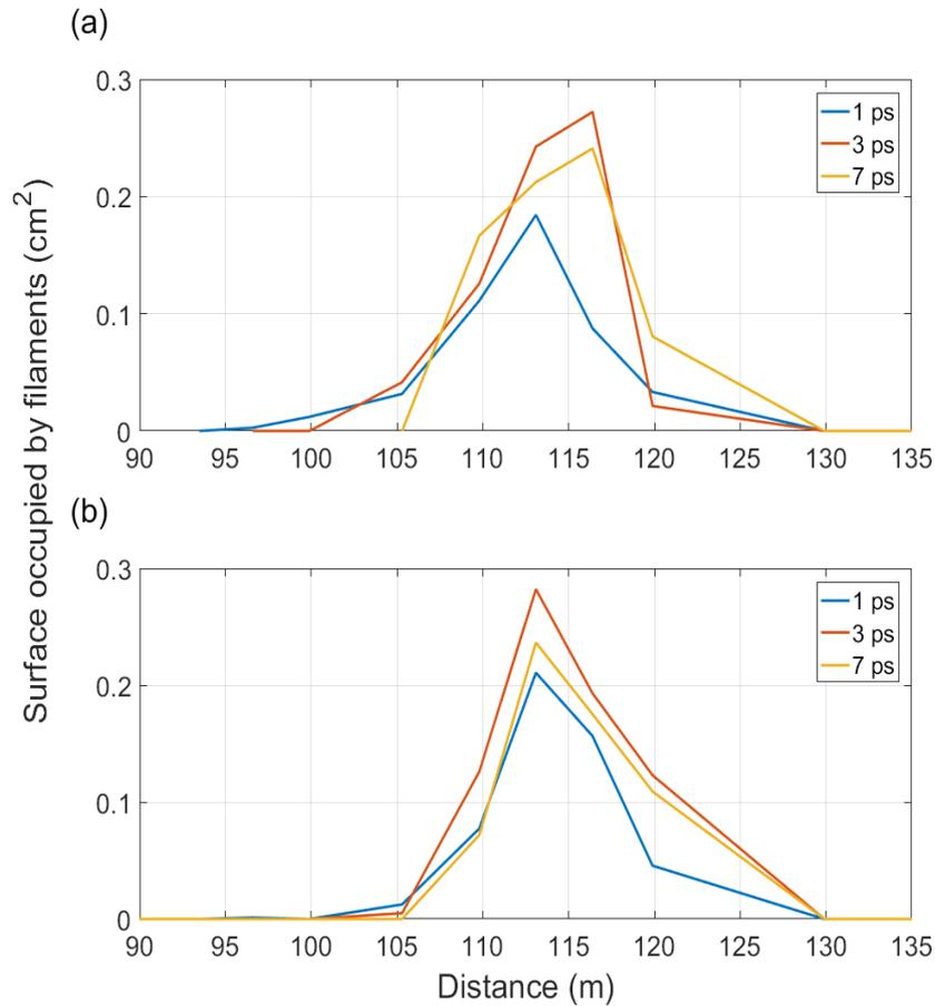
**Figure 5.3.3:** Spatial evolution of the surface occupied by filaments created by the 500 mJ (a) fundamental beam at 1030 nm and (b) the dual frequency beam at 1030+515 nm focused at 115 m, for several pulse durations ranging from 1 to 7 ps.
