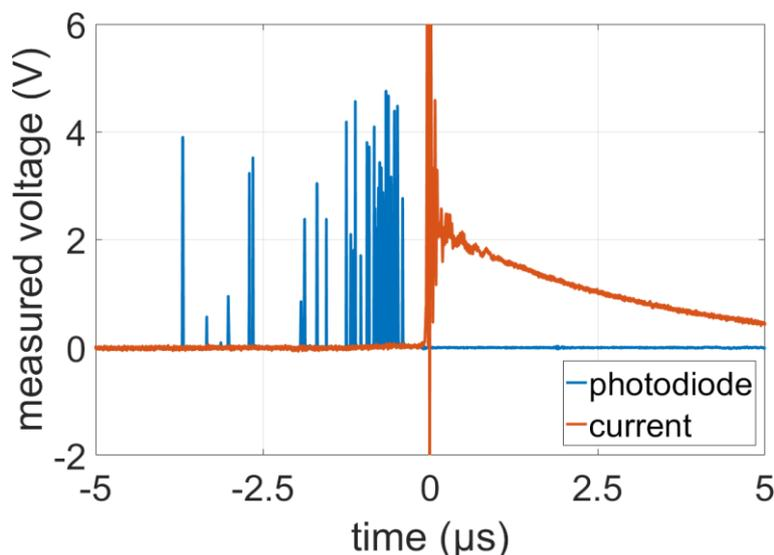
**Figure 8.3:** Measured voltage representing the (in red) discharge current and (in blue) the photodiode signal accumulated over 40 discharges. Each peak in the photodiode signal represents the temporal position of one of the 40 laser pulse as compared to the discharges.
