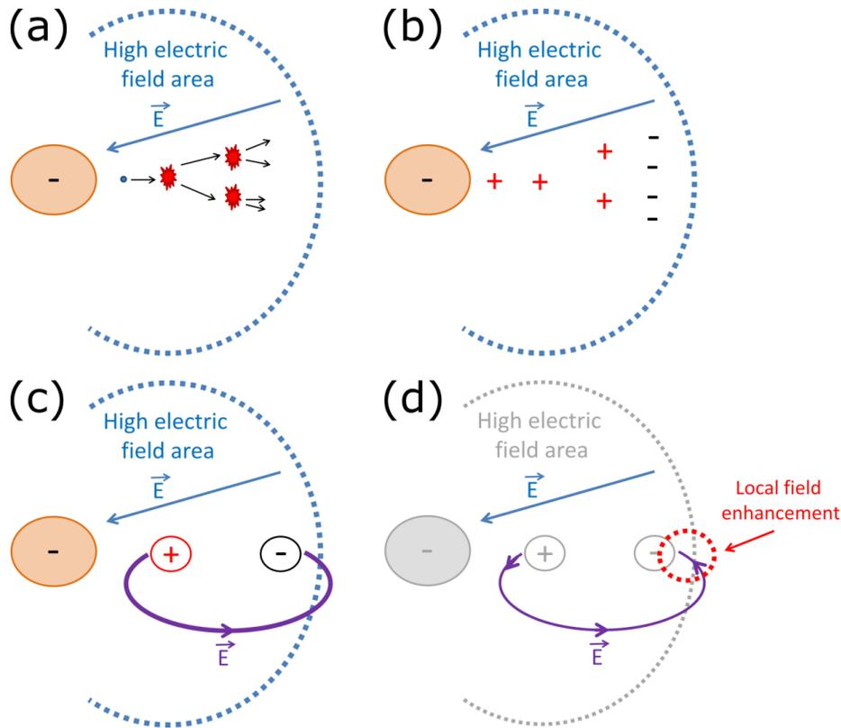
**Figure 2.2.1:** Different steps in the development of a streamer discharge. (a) It starts with an electron avalanche in the vicinity of the cathode. (b) The free electrons leave behind them positive ions as they propagate. (c) This space charge induces a secondary electric field. (d) It results in an enhanced electric field at the tip of the avalanche.
