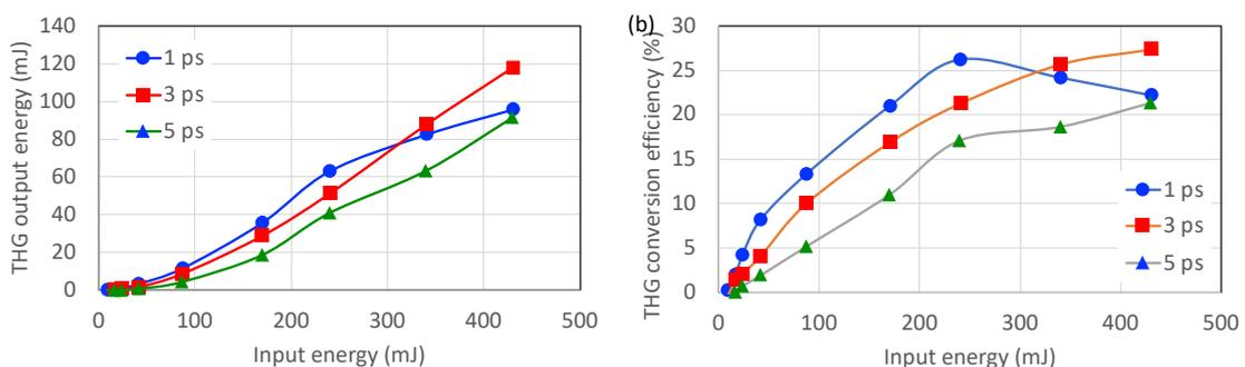
**Fig 2.3:** THG energy (a) and energy conversion efficiency (b) of the THG LBO crystal
