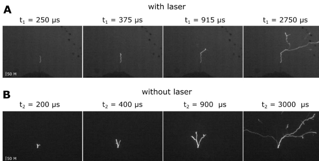
**Figure 4.2.4:** High speed camera images of upward leaders: (A) Images of the lightning path in the presence of the laser recorded on July 24 2021 at (L2) 250, 375, 915, and 2750  $\mu\text{s}$  after initiation of the discharge. (B) Images of the lightning path recorded on July 2. 2019 in the absence of laser 200, 400, 900, and 3000  $\mu\text{s}$  after initiation of the discharge.
