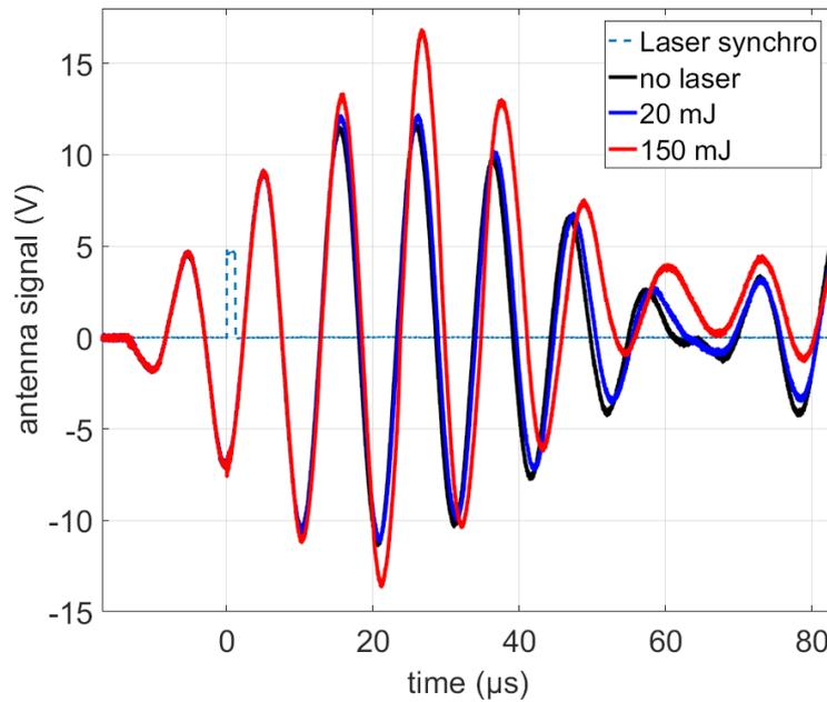
**Figure 3.2.1:** Plot of the oscilloscope measurement showing (in dashed blue) the signal of synchronization of the laser pulse, and the signal of the antenna measuring the voltage at the output of the Tesla generator without the laser (in black), in the presence of a laser pulse of energy 20 mJ (in blue), and in the presence of a laser pulse of energy 150 mJ (in red).
