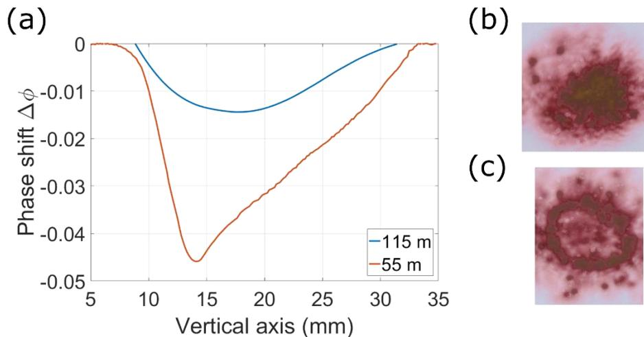
**Figure 7.2:** (a) Phase shift induced by the frequency doubled 500 mJ 1 ps pulse, focused at (red) 55 m and (blue) 115 m, measured at the geometrical focus of the beam 1  $\mu$ s after the last laser pulse. Filaments distribution measured at the same position, (b) 55 m and (c) 115 m as where the phase shift is measured.
