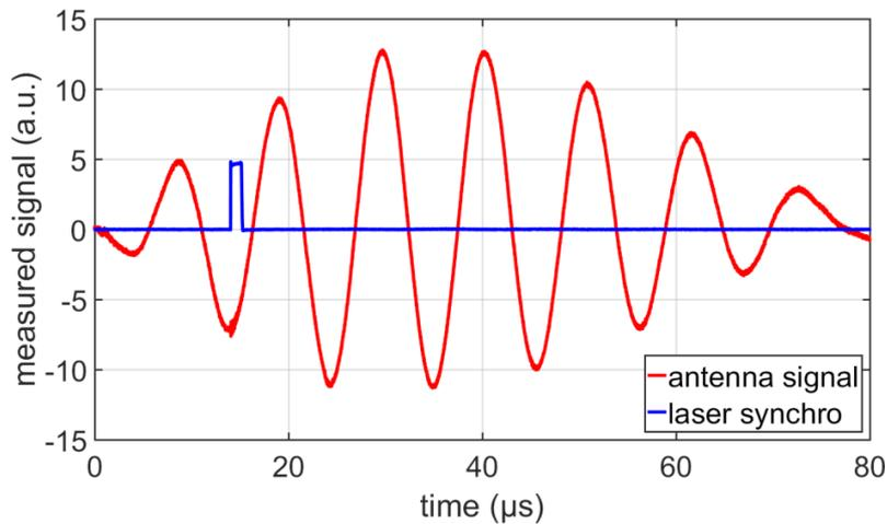
**Figure 3.1.2:** Plot of the oscilloscope measurement showing the signal of synchronisation of the laser pulse (in blue), and the signal of the antenna measuring the voltage at the high voltage electrode of the Tesla generator (in red).
