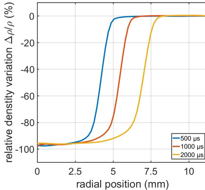
**Figure 2.6.1:** Measured radial profiles of the air density variation in the discharge for a capacitance value in the secondary circuit of 720 nF, measured at a delay of 500 μs (in blue), 1000 μs (in orange) and 2000 μs (in blue) after the beginning of the discharge. Note that the quantitative values of the density variation are not valid due to the presence of electron disturbing the measurement.
