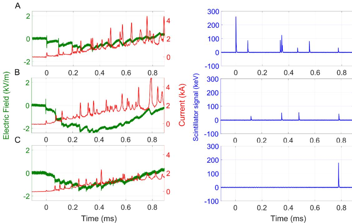
**Figure 4.4.1:** Electric signals measured for the 3 positive upward flashes L1 (A), L3 (B) and N6 (C). Top subplot for each event: The electric field scale is given on the left y-axis and the current on the right y-axis. Bottom subplot: X-ray signal detected by the Scintillator, where each peak corresponds to the integrated x-rays energy collected during the 50 ns sampling.
