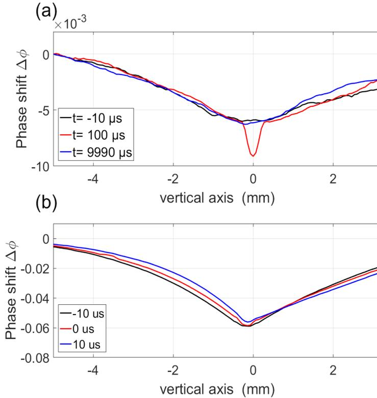
**Figure 3.3.2:** Phase shifts ( $2\pi$  rad) induced by the filamentation of a 0.8 mJ, 50 fs, 800 nm laser at a repetition rate of (a) 100 Hz and (b) 1000 Hz, measured at different delay from the last laser pulse.
