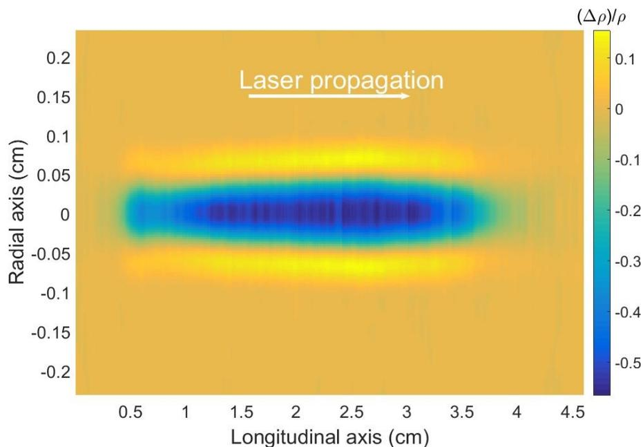
**Figure 2.3.1:** Longitudinal scan of the neutral density variation over the whole filament length. Measurements are performed 10  $\mu\text{s}$  after the creation of the filament. The filament is produced by focusing a laser pulse of 14 mJ, 50 fs focused at  $\text{NA}=0.0078$ .
