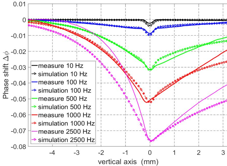
**Figure 3.3.1.** Phase shifts ( $2\pi$  rad) induced by the filamentation of 0.8 mJ, 35 fs laser pulses focused at  $f/100$ , measured 100 ms after the last laser pulse (full line) and corresponding simulations (circles), at various repetition rates ranging from 10 to 2500 Hz.
