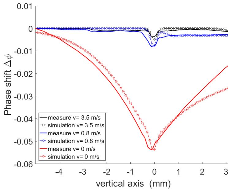
**Figure 3.5.1:** Phase shifts induced by the filamentation of 0.8 mJ, 35 fs laser pulses at a 1000 Hz repetition rate, focused at  $f/100$ . (a) Phase shifts measured (full line) and simulated (circles) with different air flows. Input parameters for simulations are  $\Delta T_0 = 18 \text{ K}$  and  $R_0 = 170 \mu\text{m}$ .
