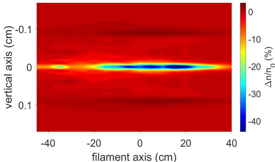
**Figure 3.2.1:** Measurement of the density variation of the under-dense channel responsible for the guiding of the discharge, created by a 150 mJ, 780 fs, 800 nm laser pulse focused at 7 m. This measurement was done 10  $\mu$ s after the laser pulse.
