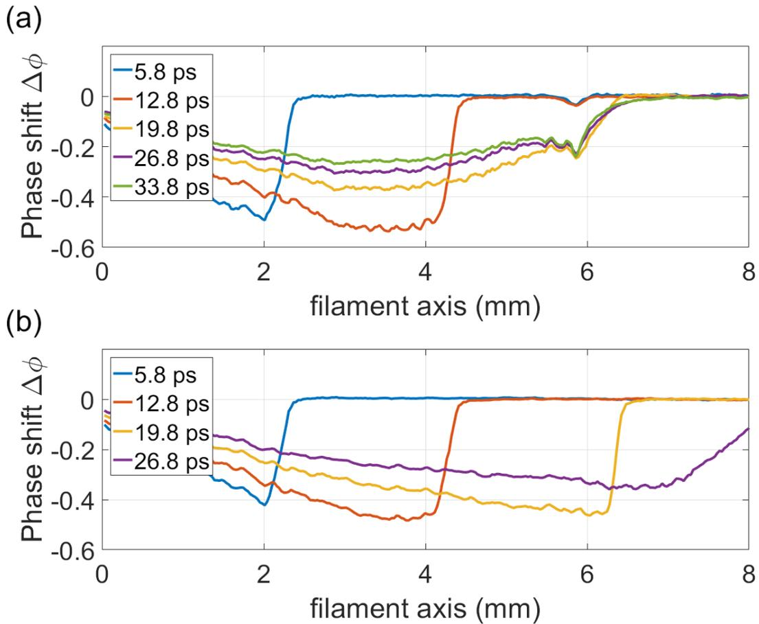
**Figure 3.9.3:** Measured phase shift along the filamentation axis measured at delays of 5.8 ps (in blue), 12.8 ps (in red), 19.8 ps (in yellow), 26.8 ps (in violet) and 33.8 ps (in green) measured at a repetition rate of (a) 100 Hz and (b) 10 Hz.
