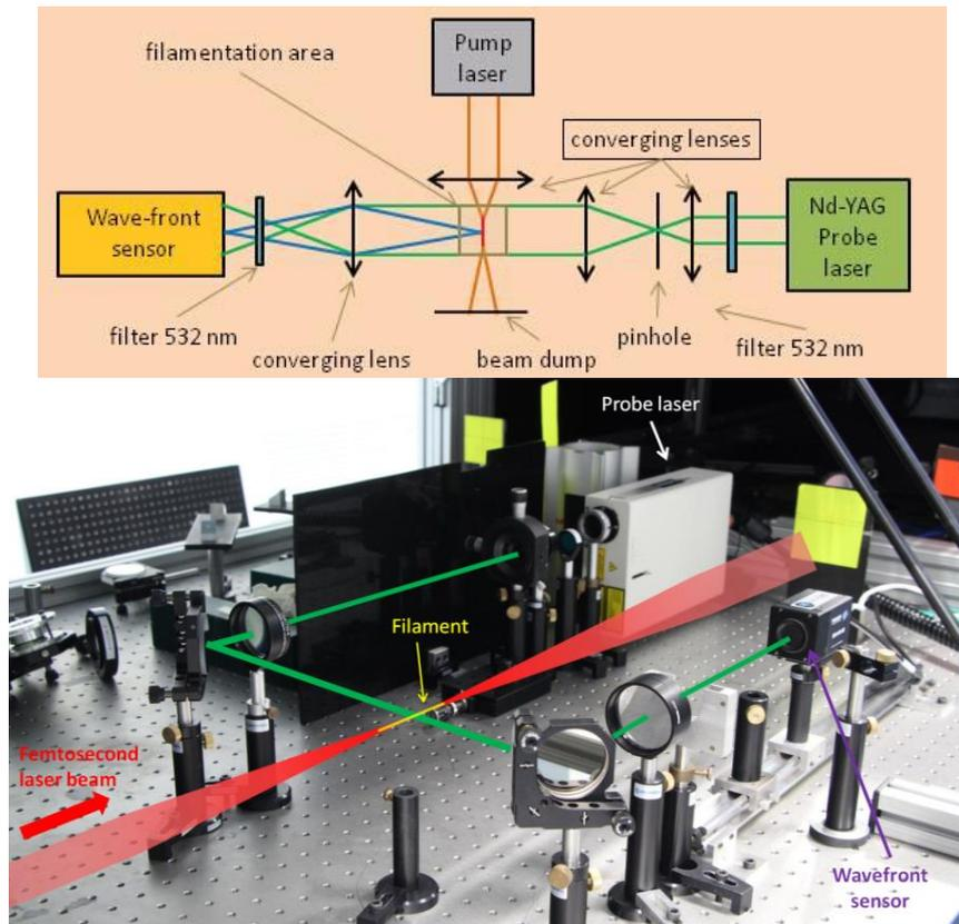
**Figure 2.1.1:** Schematics and photo of the experimental setup.
