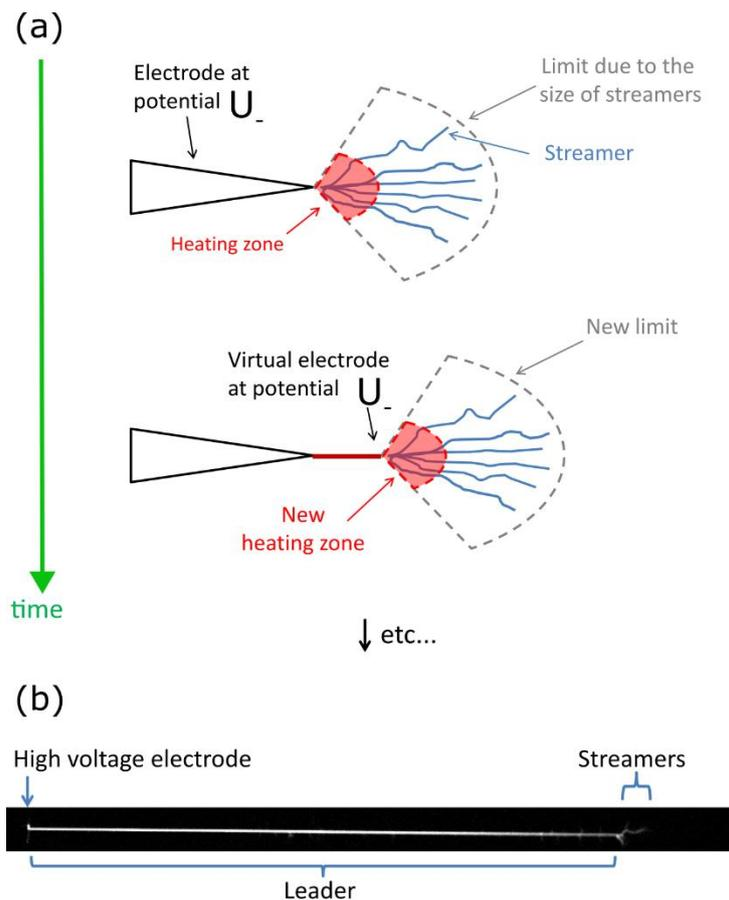
**Figure 2.3.1:** (a) Scheme of the cycle of propagation of a streamer-leader discharge. (b) Picture of a 1.4 m long guided streamer-leader discharge recorded by a high-speed camera, showing the leader part of the discharge with streamers emerging at its extremity.
