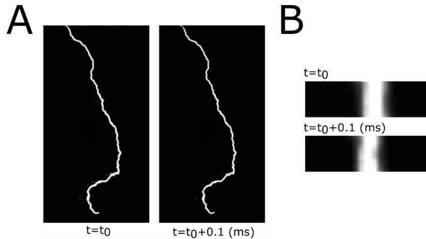
**Figure 4.7.1.1:** Consecutive frames recorded by the high-speed camera located at Schwagalp for the event N08, separated by 1 ms. (a) Full frames. (b) zoom on a part of the frames to highlight the movement of the leader path.
