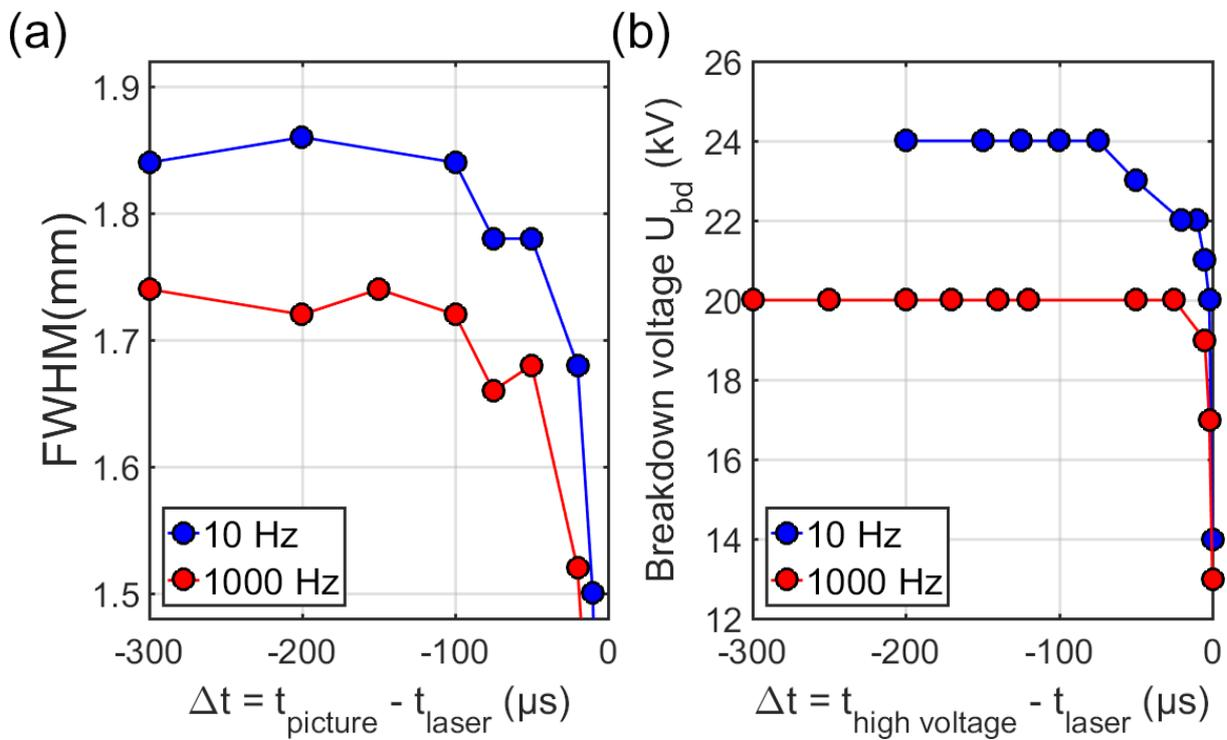
**Figure 3.7.4:** Evolution of (a) the discharge FWHM and (b) the breakdown voltage inducing by a 0.8 mJ, 35 fs laser pulses focused at  $f/100$  and at a repetition rate of 1000 Hz, as a function of the delay between the high voltage pulse and the last laser pulse.
