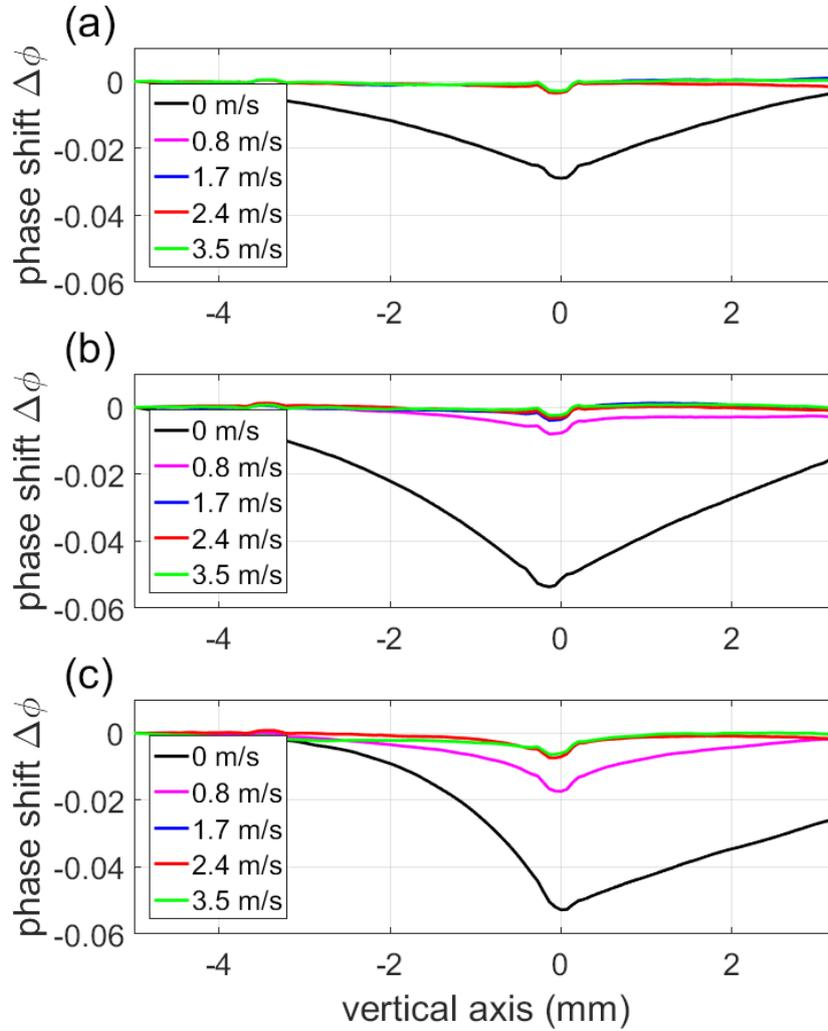
**Figure 3.5.2:** Measured phase shifts induced by the filamentation of 0.8 mJ, 35 fs laser pulses, focused at  $f/100$ , at a repetition rate of (a) 500 Hz, (b) 1000 Hz and (c) 2500 Hz, with different air flows.
