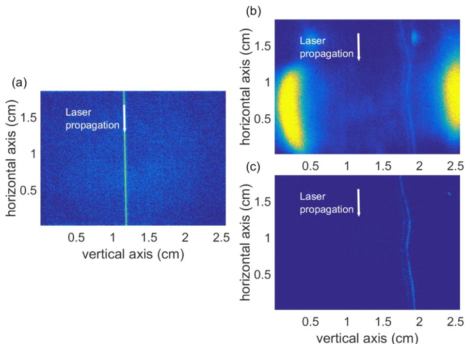
**Figure 3.1.2.1:** Schlieren imaging of two consecutive discharges separated by 100 ms. (a) image of the first long discharge, (b) image of the second short discharge, and (c) image of the second short discharge with the background subtracted to distinguish the discharge path.
