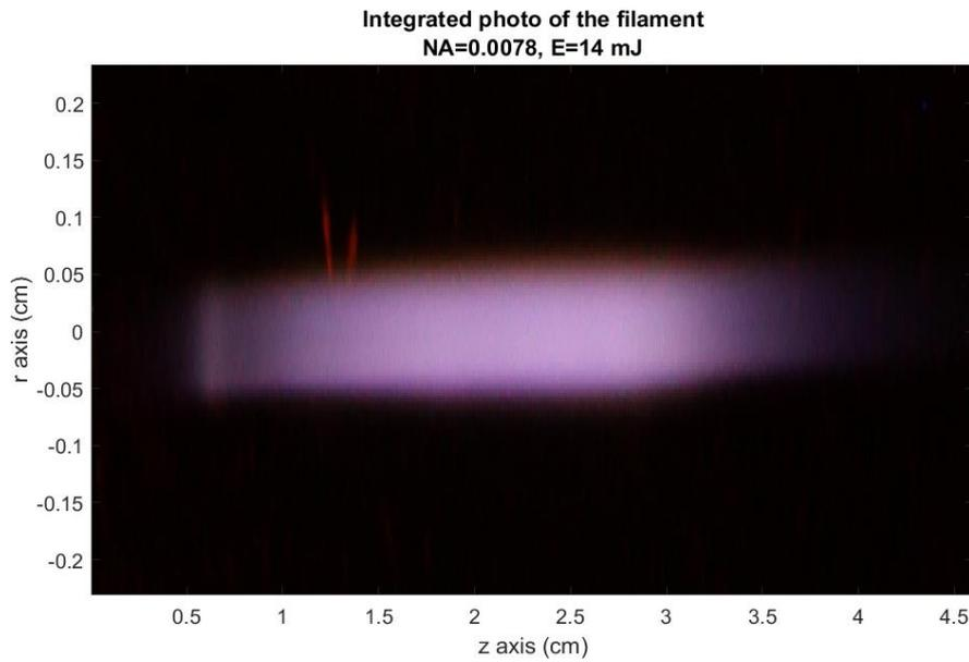
**Figure 2.3.2:** Picture of the luminescence of the 3 cm filament plasma characterized in Figure 2.3.1.
