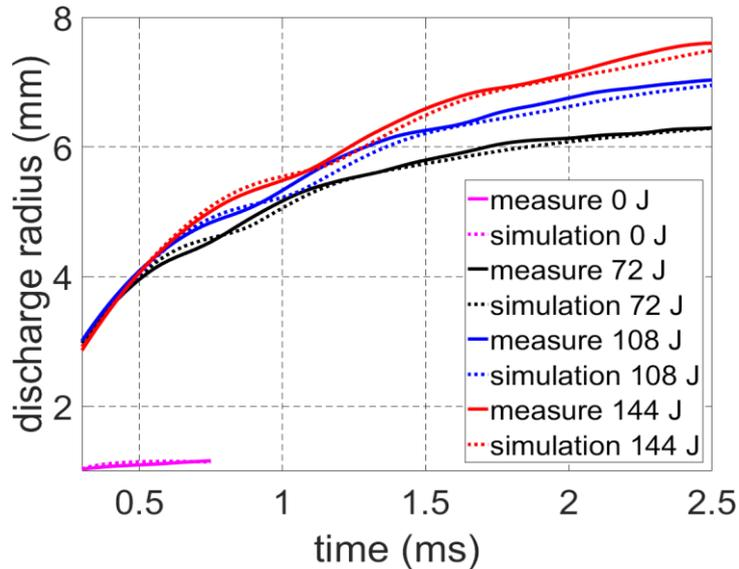
**Figure 2.4.2:** Comparison between the measured and simulated radius of the temporal evolution of the discharge for capacitance values in the secondary circuit of  $C = 720$  nF (labelled as 4C, in red),  $C = 540$  nF (labelled as 3C, in blue),  $C = 350$  nF (labelled as 2C, in black), and for no capacitance (labelled as 0C, in violet).
