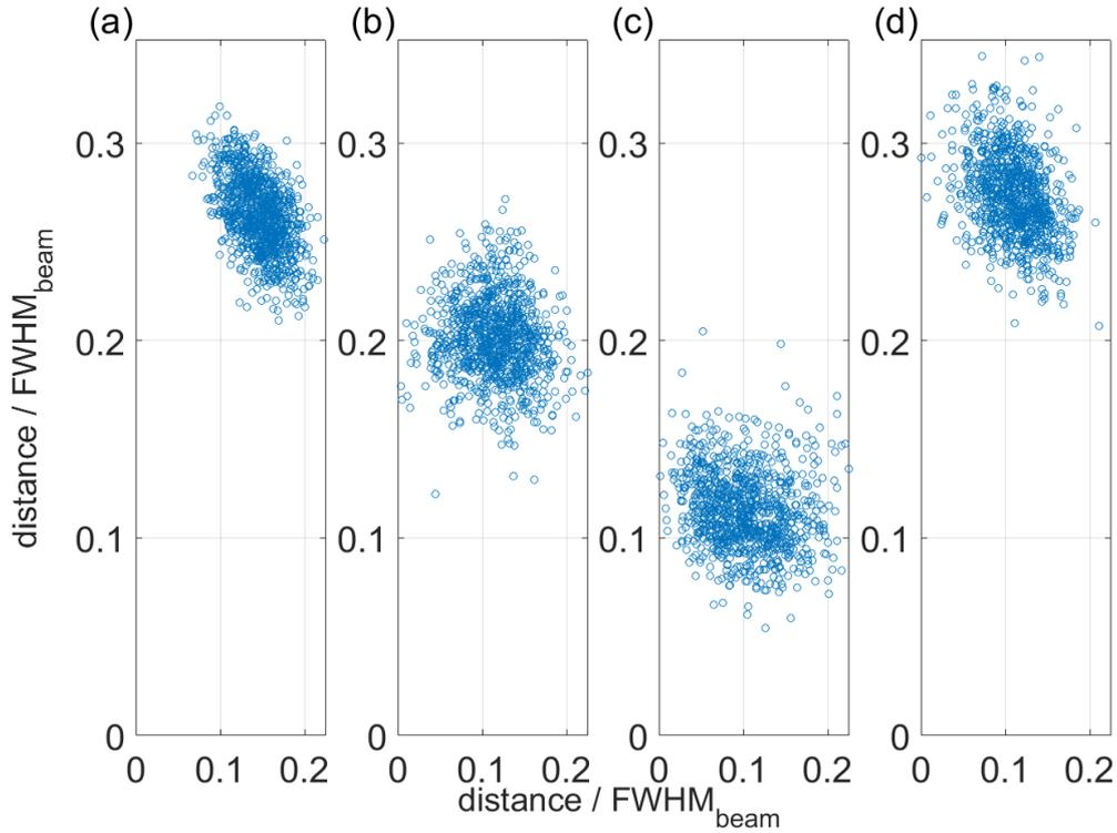
**Figure 3.6.1:** Downward shift of the mean position of the 0.8 mJ, 35 fs laser beam focused at  $f/100$  measured 25 cm after the filamentary zone, measured without air flow at 10 Hz (a), 100 Hz (b), 1000 Hz (c), and at 1000 Hz with air flow (d).
