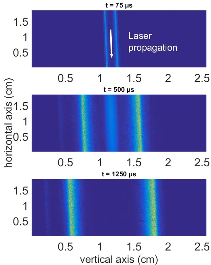
**Figure 2.3.3:** Schlieren images captured at delays of 75, 500 and 1250  $\mu\text{s}$  after the beginning of the discharge. The temporal evolution of the edge of the discharge can be observed (in yellow). Light emitted from the discharge can also be observed in the central part of the image captured at a delay of 500  $\mu\text{s}$ .
