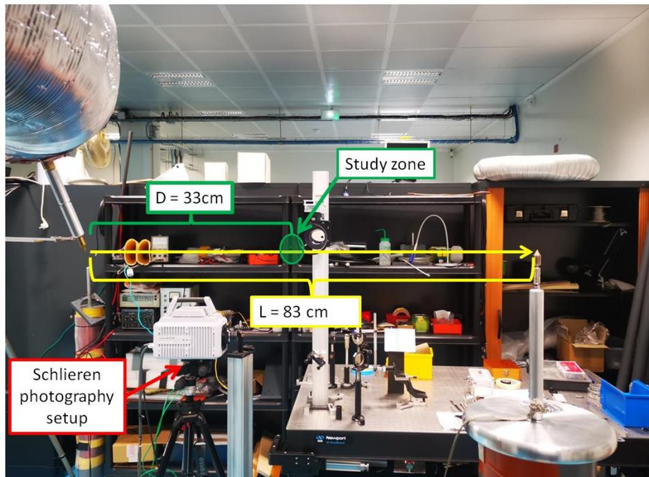
**Figure 2.3.2:** Experimental setup of the Schlieren imaging system.
