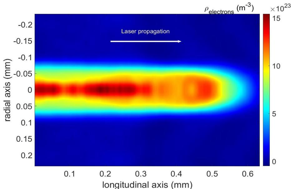
**Figure 2.4.2:** Electron density measured during the filamentation process.
