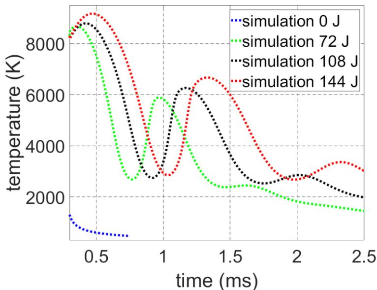
**Figure 2.4.3:** Simulation of the temporal evolution of temperature at the discharge center for capacitance values in the secondary circuit of  $C = 720$  nF (labelled as 4C, in red),  $C = 540$  nF (labelled as 3C, in black),  $C = 350$  nF (labelled as 2C, in green), and for no capacitance (labelled as 0C, in blue).
