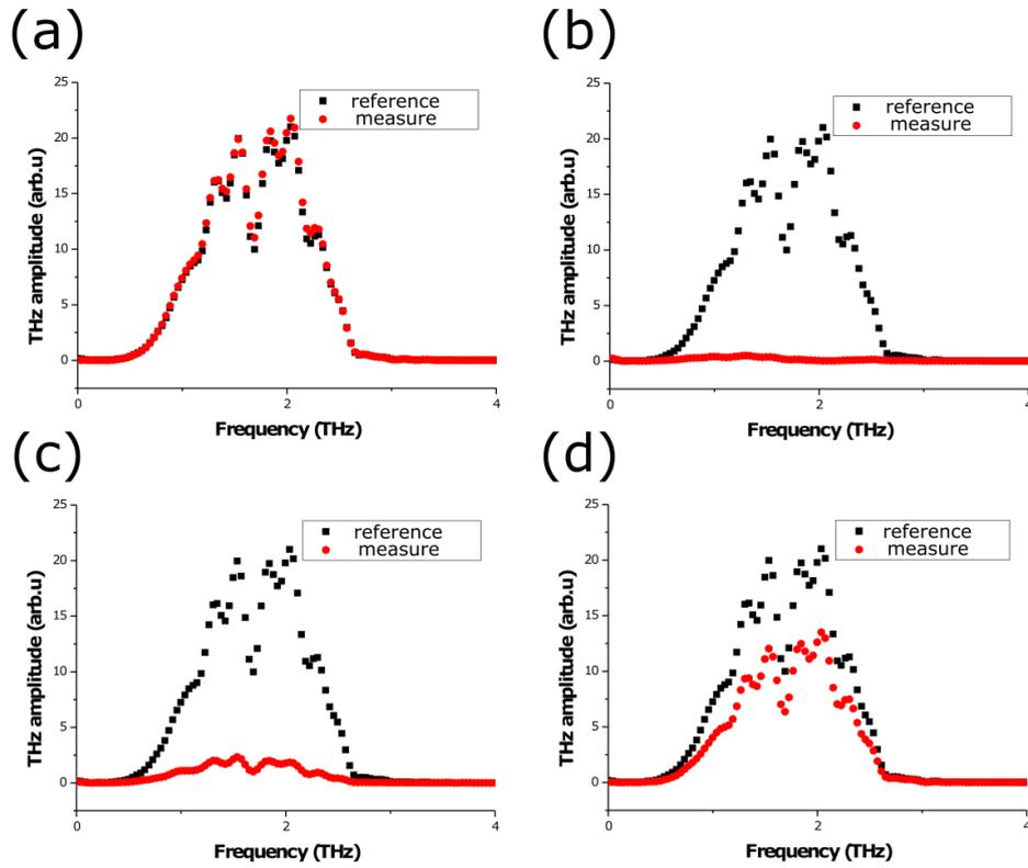
**Figure 3.4.2:** Comparison between the reference unperturbed THz spectrum and the THz spectrum measured at the delays (a) -16 ps, (b) 0 ps, (c) 133 ps, and (d) 246 ps relative to the last laser pulse.
