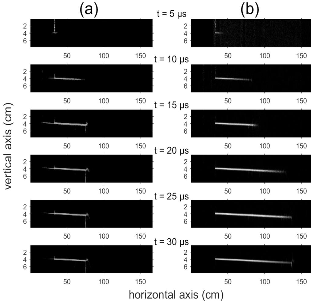
**Figure 3.1.3:** High speed camera frames showing the propagation of the electrical discharge guided by filaments created by a pump laser set at energy of 20 mJ (a) and 150 mJ (b), corresponding to the regular filamentation and superfilamentation regime, respectively. The high voltage electrode is located at the 32 cm position of the horizontal axis. The laser propagates from the left to the right of the frames.
