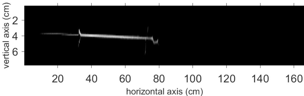
**Figure 3.1.4:** High-speed camera frame showing the propagation of the electrical discharge guided by filament created by a laser pulse with an energy of 20 mJ, taken 30  $\mu\text{s}$  after the laser pulse. The discharge propagates in two opposite directions (upstream and downstream of the laser propagation) in regard to the high voltage electrode, located at the 32 cm position of the horizontal axis. The laser propagates from the left to the right of the frame.
