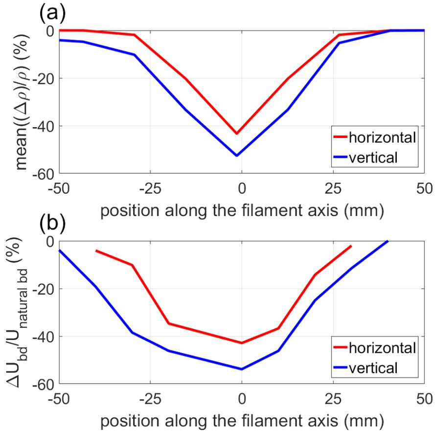
**Figure 3.8.6:** Comparison between (a) the mean of the simulated density variation between the two electrodes and (b) the measured reduction of the breakdown voltage, at different position along the filament axis for both a vertical (blue) and horizontal (red) filament, measured at a laser repetition rate of 1000 Hz.
