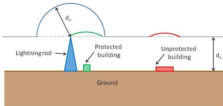
**Figure 1.1:** Illustration of a lightning rod capture region (in blue), showing a protected building whose capture region (in green) is inside the one of the lightning rod and an unprotected building whose capture region (in red) is outside the protection range of the lightning rod.  $d_s$  is the striking distance.
