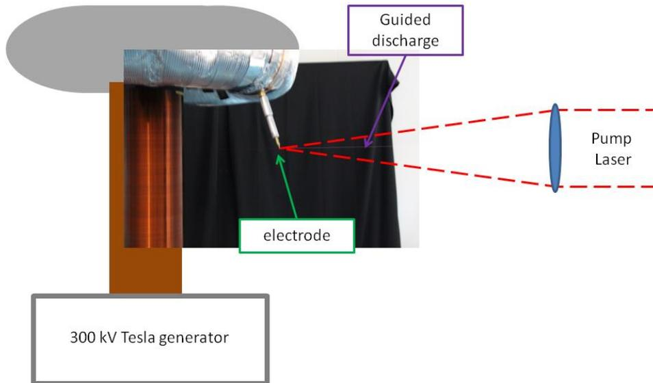
**Figure 3.1.1:** Experimental setup used to measure the length of the guided discharge as a function of the pump energy of the laser.
