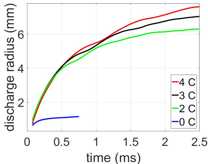
**Figure 2.3.5:** Measured temporal evolution of the discharge radius for capacitance values in the secondary circuit of  $C = 720$  nF (labelled as 4C, in red),  $C = 540$  nF (labelled as 3C, in black),  $C = 350$  nF (labelled as 2C, in green), and for no capacitance (labelled as 0C, in blue).
