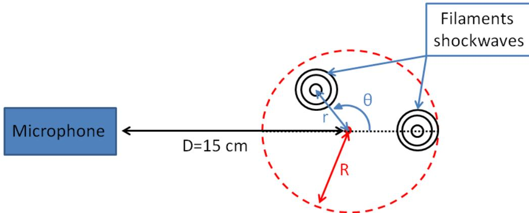
**Figure 4.3.2:** Schematic of the microphone measurement.
