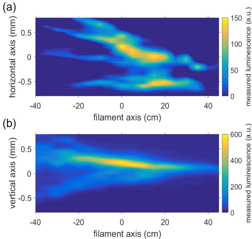
**Figure 2.3.2:** Picture of the luminescence from the plasma measured for an energy of 150 mJ, pulse duration 780 fs, taken from the top (a) and from the side (b). The picture is averaged over 50 laser pulses.
