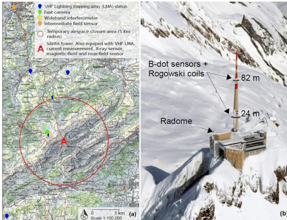
**Figure 2.1.1:** (a) Map of the experimental site, including auxiliary instruments and no-fly zone. (b) General view of the station and location of the Rogowski coils and B-dot sensors measuring lightning currents.
