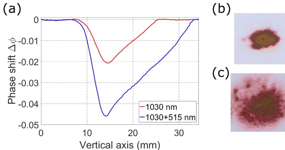
**Figure 7.3:** Phase shift induced by (in blue) the 500 mJ 1 ps frequency doubled beam and (in red) the fundamental beam, focused at 55 m, measured at the focal distance 1  $\mu$ s after the last laser pulse. Filaments distribution measured at the same position as where the phase shift is measured for (b) the fundamental and (c) the frequency doubled beam.
