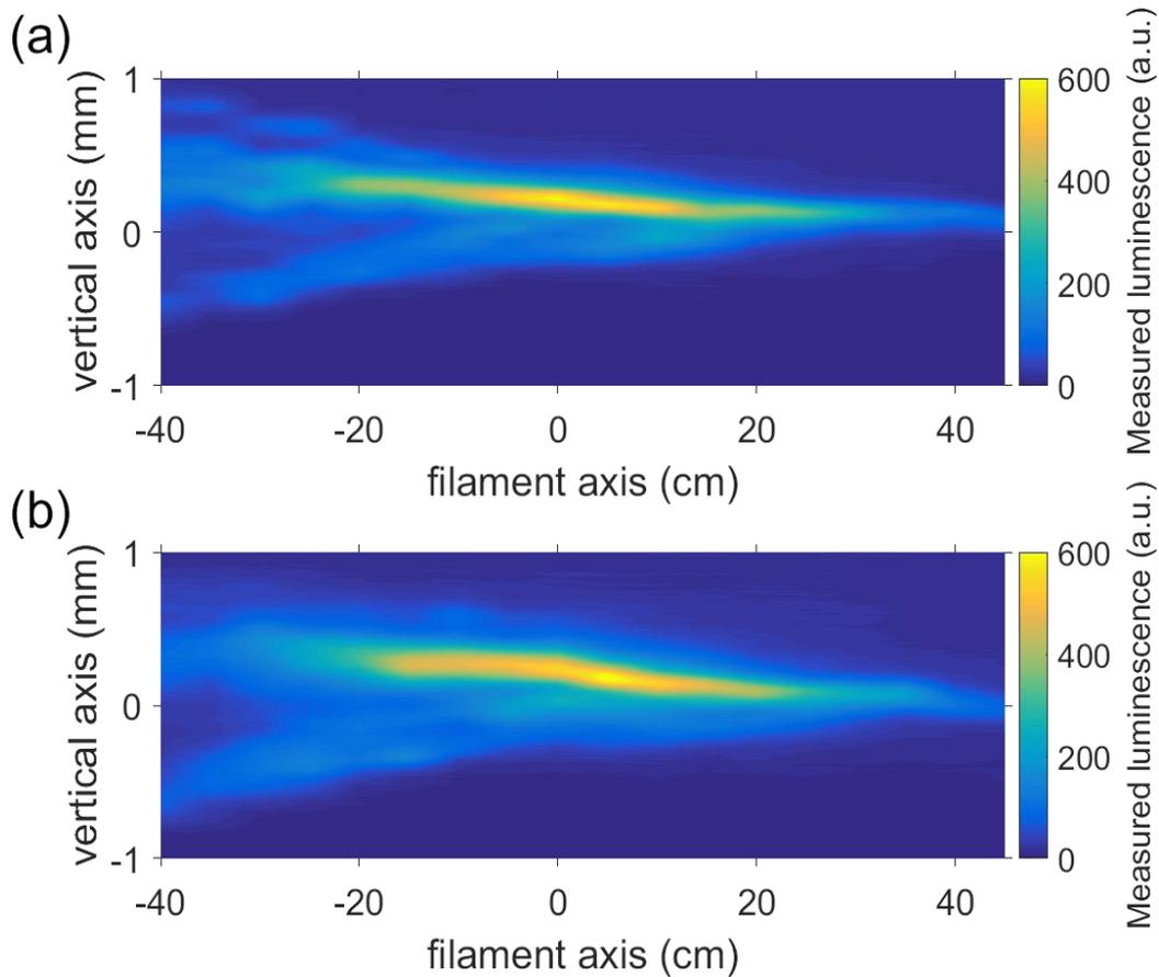
**Figure 2.1.4:** Picture of the luminescence from the plasma measured for an energy of 150 mJ, for a pulse duration of 780 fs (a) and 50 fs (b). The laser propagates from the negative to the positive values of the filament axis, and the lens focal plane is at  $z = 10$  cm.
