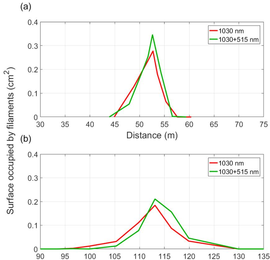
**Figure 5.2.2:** Spatial evolution of the surface occupied by filaments created by the 500 mJ 1 ps fundamental beam (red) or the frequency doubled beam (green), focused at either (a) 55 m or (b) 115 m.
