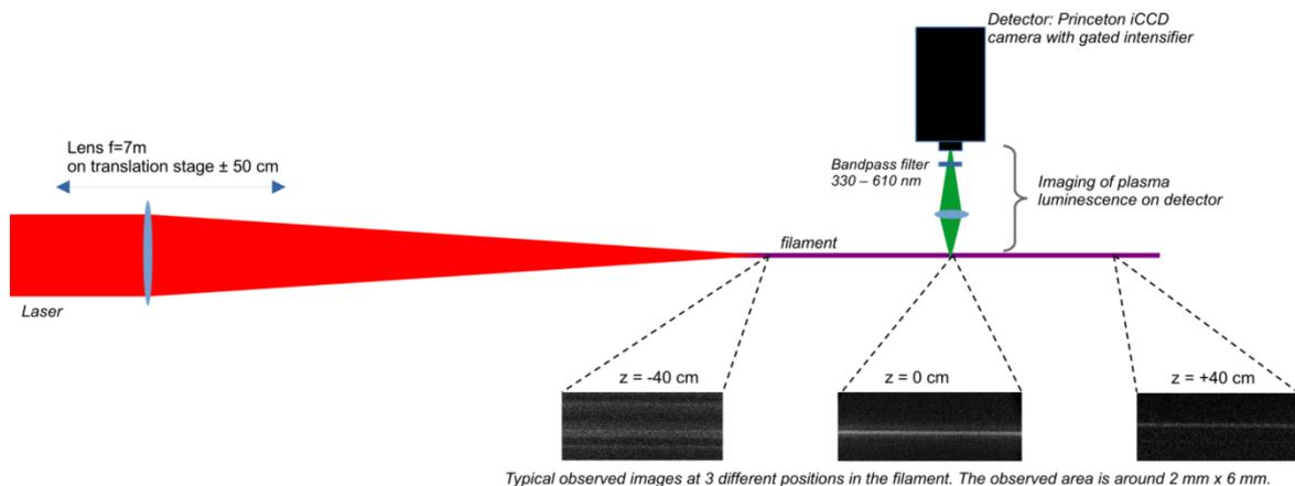
**Figure 2.1.1:** Experimental setup used to measure the plasma luminescence.
