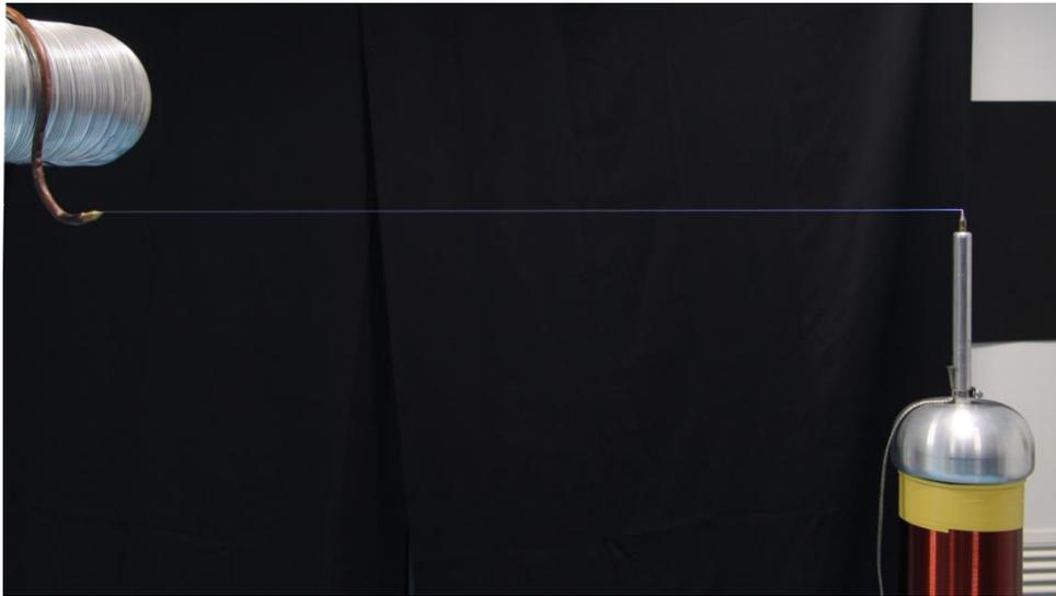
**Figure 1:** Picture of a 80 cm guided discharge.
