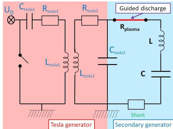
**Figure 2.1.1:** Electrical setup used to create long lived 80 cm long guided discharges. The Tesla generator (in red) produces the initial high voltage pulse creating the guided discharge, while the secondary circuit (in blue) injects a long lived current that increases the discharge lifetime.
