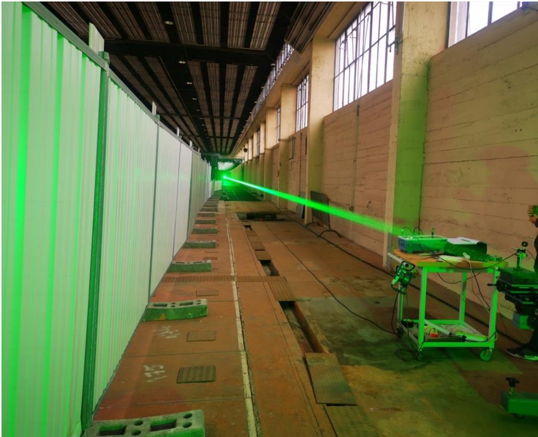
Figure 1: Picture of the frequency doubled beam propagating along the 140 m experimental zone.
