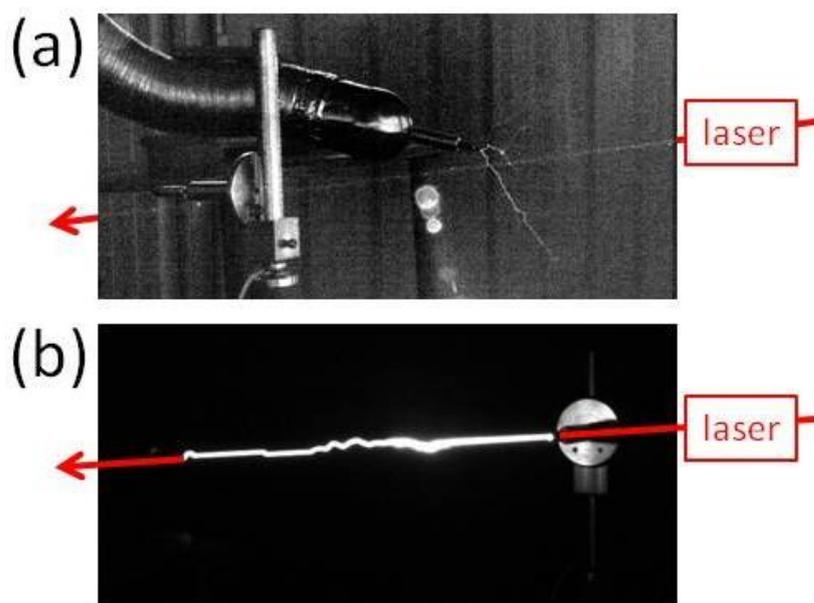
**Figure 8.6:** (a) Picture of the unguided discharge observed when using the laser focused at 115 m. (b) Picture of the partially guided 40 cm long discharge observed when using the laser focused at 55 m.
