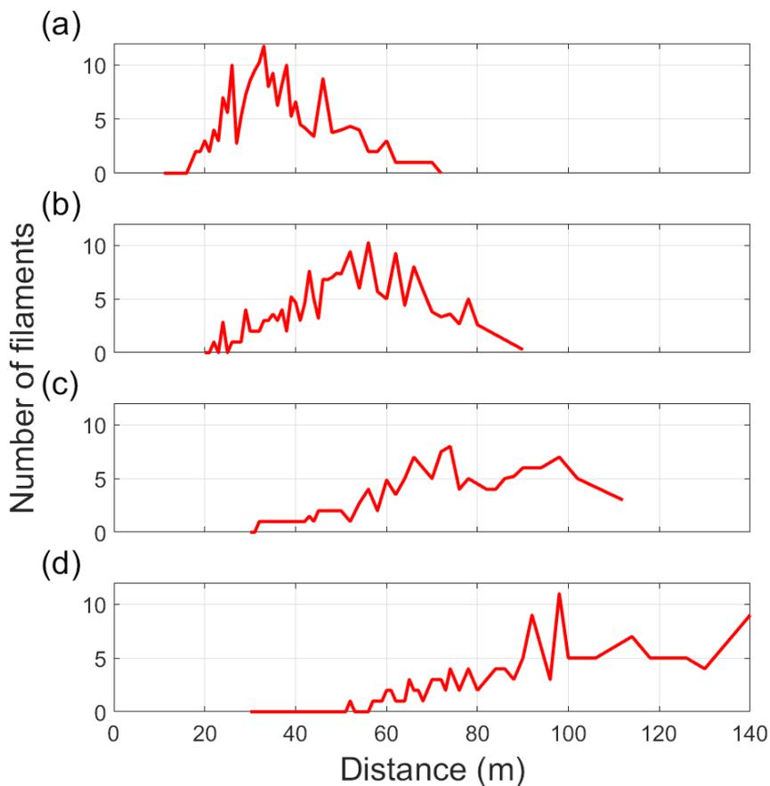
**Figure 4.2.2:** Evolution of the number of filaments along the laser propagation of a 500 mJ 1030 nm laser pulse for pulse durations of (a) 1 ps, (b) 3 ps, (c) 5 ps and (d) 7 ps.
