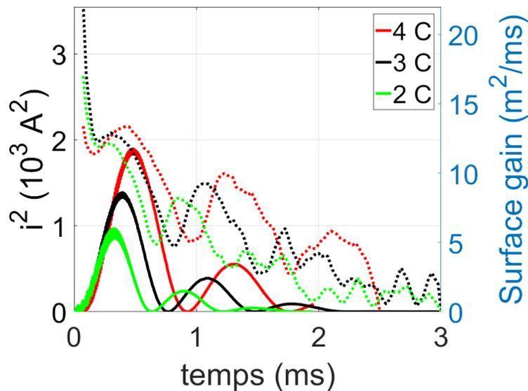
**Figure 2.3.7:** Comparison between the temporal evolution of the surface gain of the cross section of the discharge  $2\pi r \frac{\partial r}{\partial t}$  (dashed lines) and the temporal evolution of the square of the current (continuous lines), for capacitance values in the secondary circuit of  $C = 720$  nF (labelled as 4C, in red),  $C = 540$  nF (labelled as 3C, in black),  $C = 350$  nF (labelled as 2C, in green), and for no capacitance (labelled as 0C, in blue).
