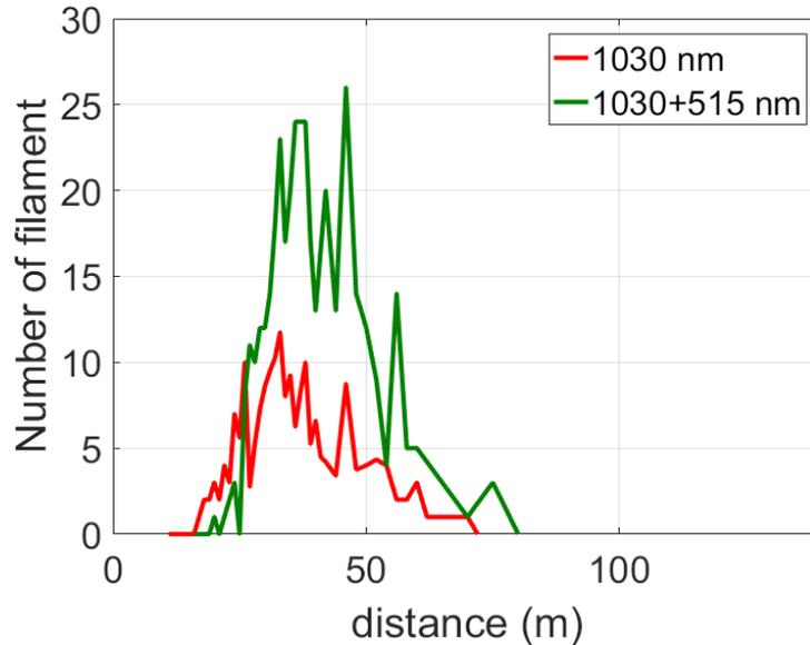
**Figure 4.2.3:** Evolution of the number of filaments along the laser propagation measured for the 1030 nm and 1030+515 nm pulses, with a pulse duration of 1 ps.
