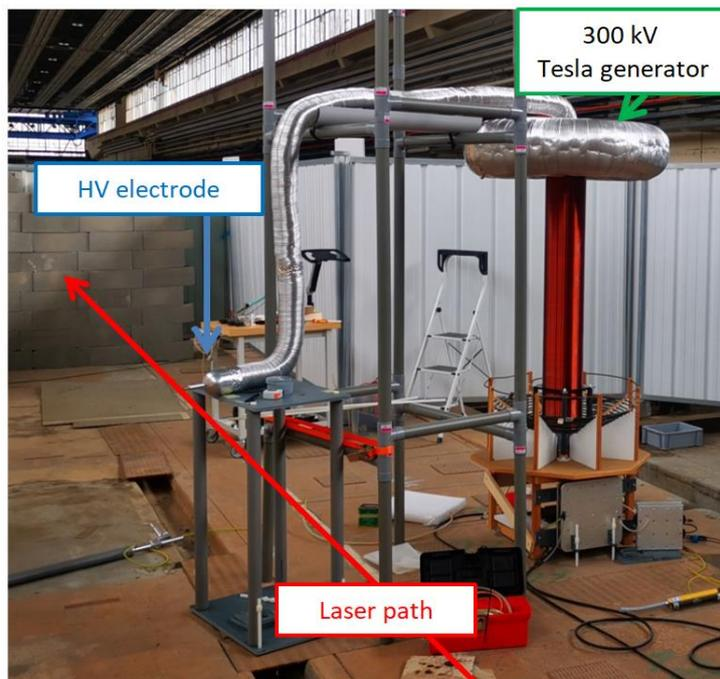
**Figure 8.5:** Experimental setup using the 300 kV Tesla generator.
