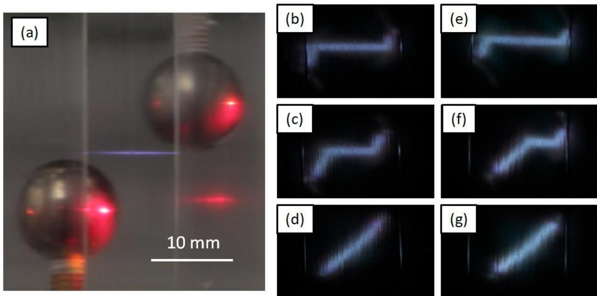
**Figure 3.7.3:** Pictures of the filament region showing the plasma luminescence and the two electrodes (a). Pictures of the discharge in air for three different triggering delays between the high voltage pulse and the last laser pulse at 10 Hz (b, c, d) and 100 Hz (e, f, g).
