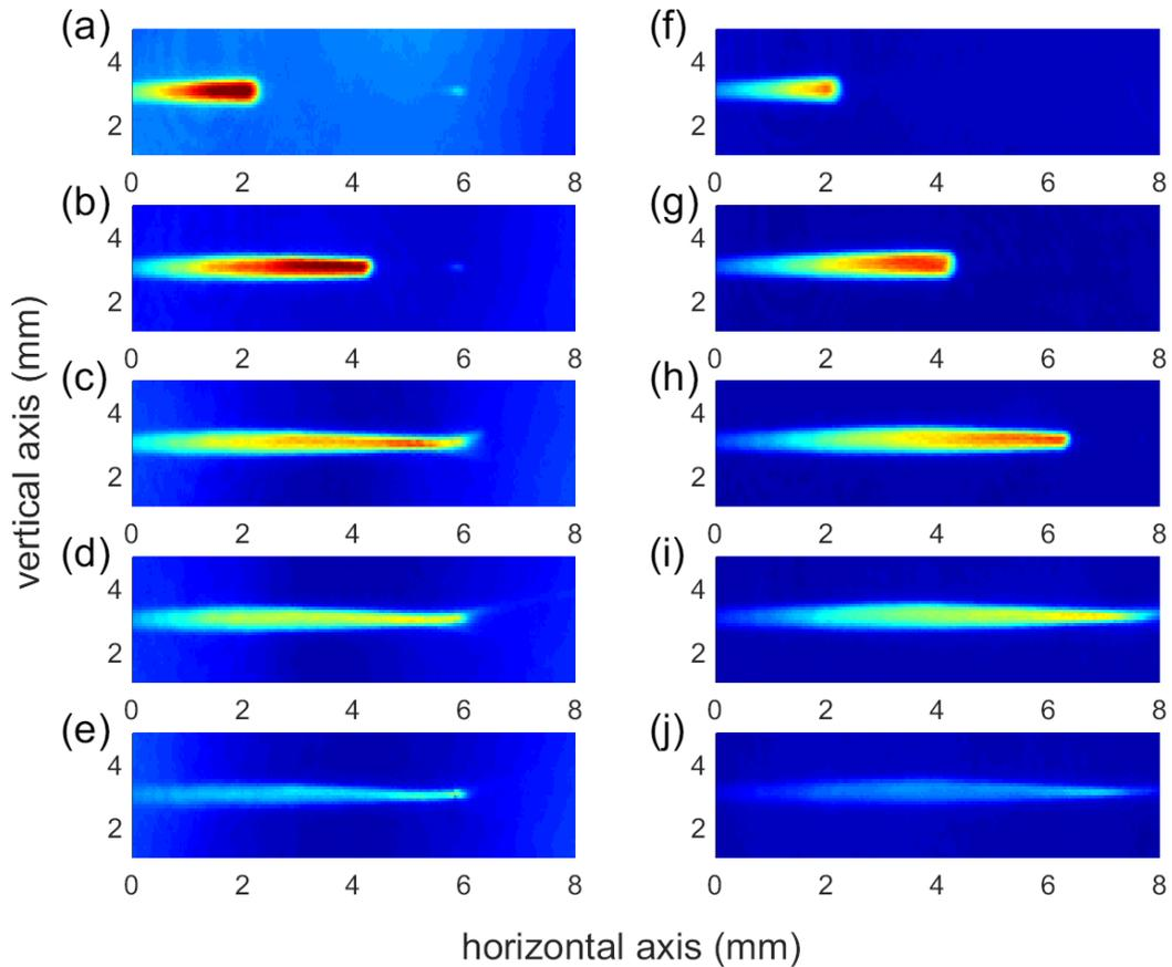
**Figure 3.9.2:** 2D maps of the phase shift measured by interferometry at a delay of (a and f) 5.8 ps, (b and g) 12.8 ps, (c and h) 19.8 ps, (d and i) 26.8 ps, and (e and j) 33.8 ps after the beginning of the filamentation, using a 14 mJ, 50 fs, 800 nm laser at a repetition rate of 100 Hz and 10 Hz, respectively.
