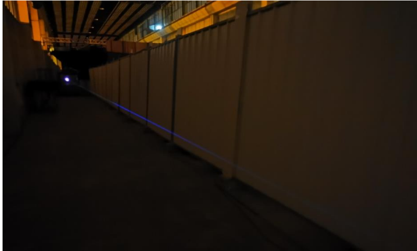
Figure 5.4.1: Picture of the luminescence emitted by filaments created by the 500 mJ laser focused at 55 m.
